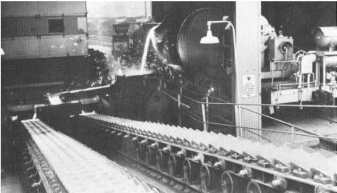
**Fig. 9.56** View of a pig casting machine in operation, showing hot metal being divided into two streams by the split runner to simultaneously fill the molds in each of the two strands.
