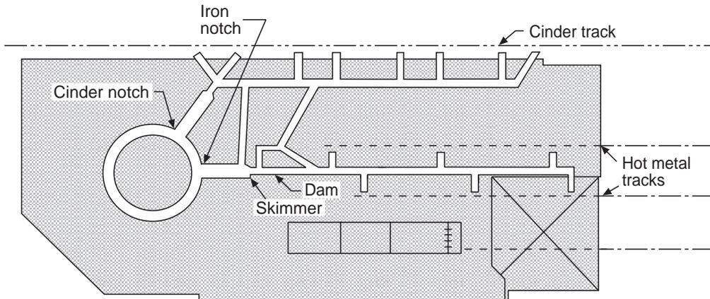
Fig. 9.46 Layout of a single taphole casthouse.
