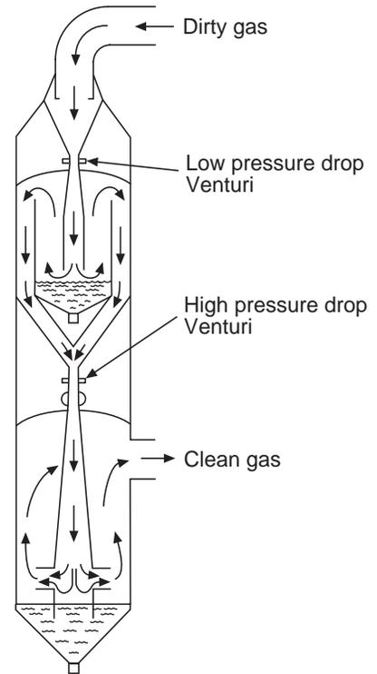
**Fig. 9.32** Schematic of an automatic two-stage venturi gas washer that controls blast furnace top pressure.
