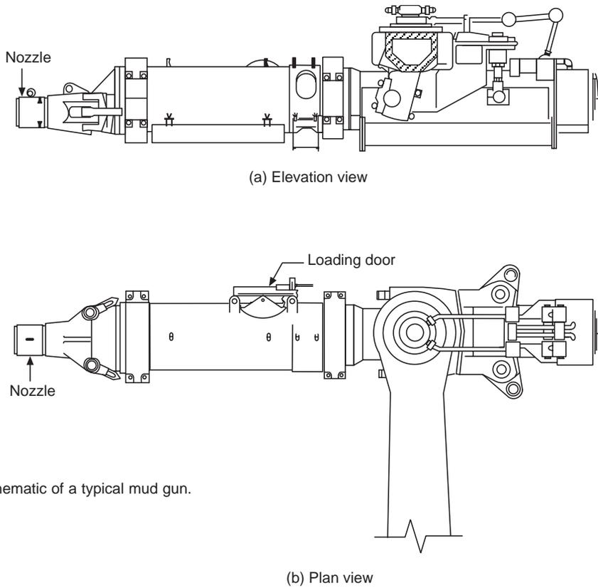
Fig. 9.50 Schematic of a typical mud gun.
