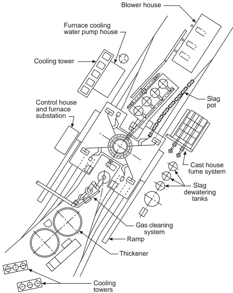
Fig. 9.48 Layout of a casthouse arrangement with four tapholes.
