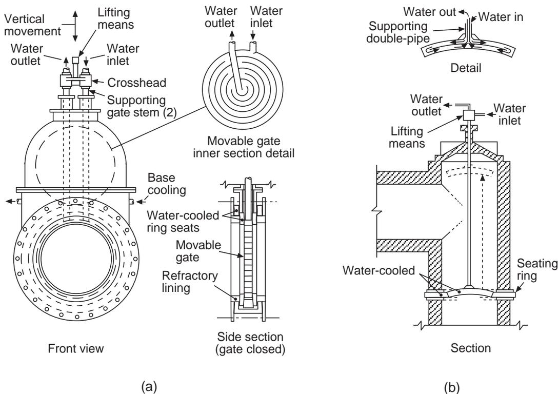
Fig. 9.37 Hot blast valves.
