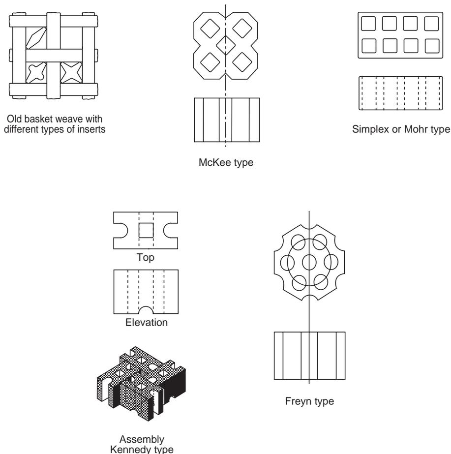
**Fig. 9.35** Different checker designs employed in blast furnace stoves. The basket weave design with inserts is no longer used.
