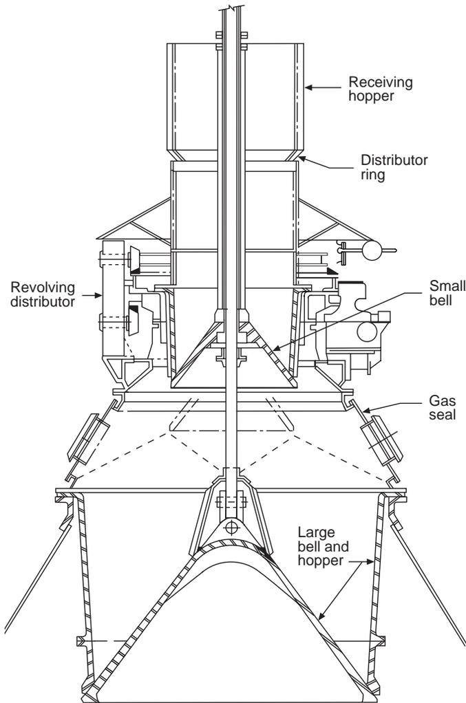
Fig. 9.22 Schematic of a typical two-bell top.
