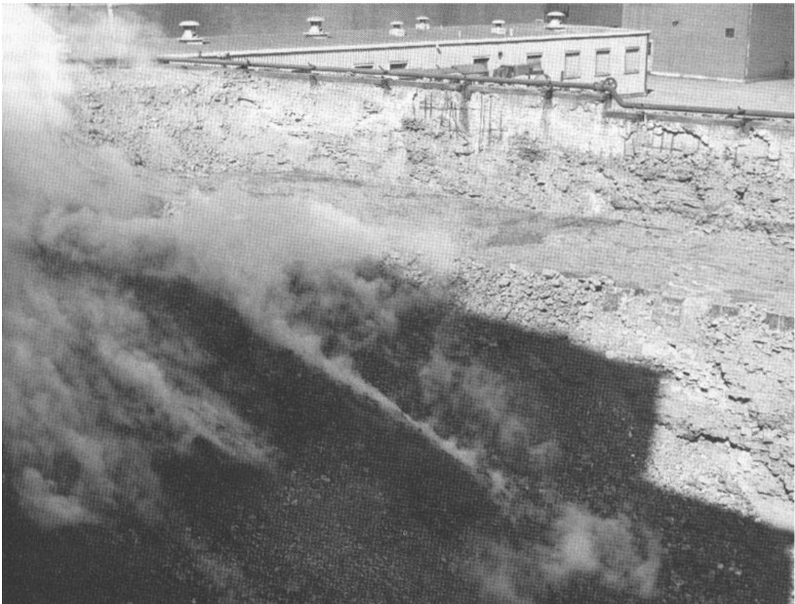
Fig. 9.54 Slag pit adjacent to a blast furnace.
