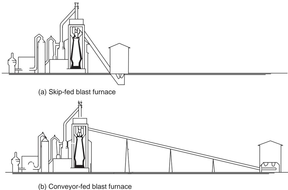
Fig. 9.16 Methods for delivering raw materials to the furnace top.
