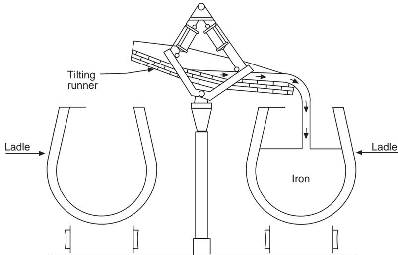
Fig. 9.52 Typical tilting runner arrangement.
