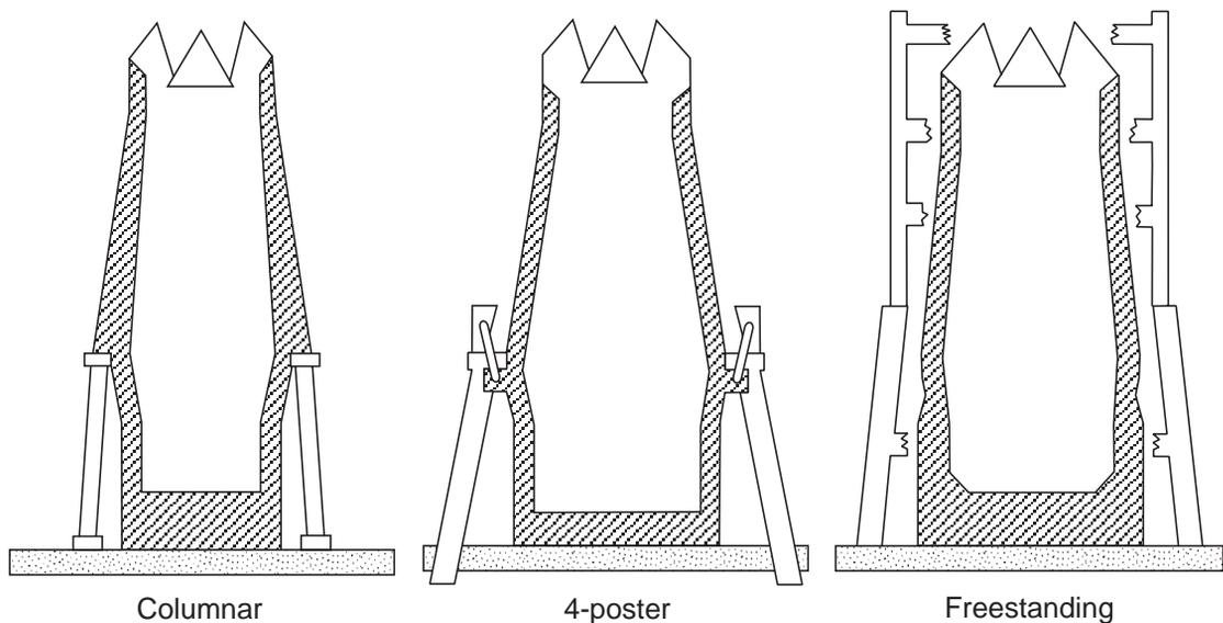
Fig. 9.2 Blast furnace support structures.
