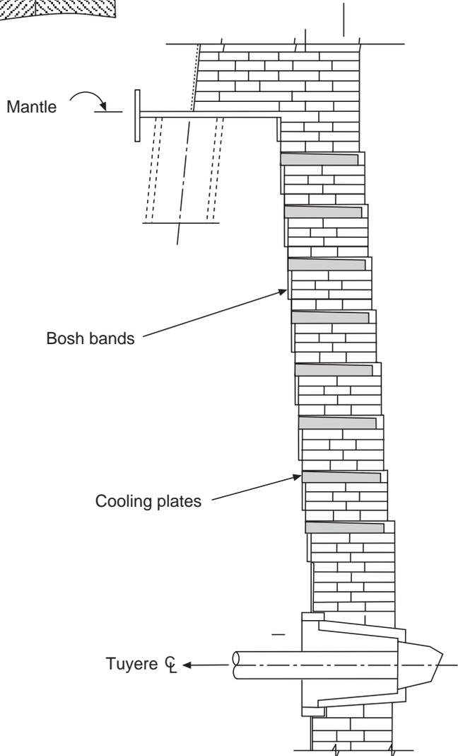
Fig. 9.7 Bosh band configuration with copper plate cooling.
