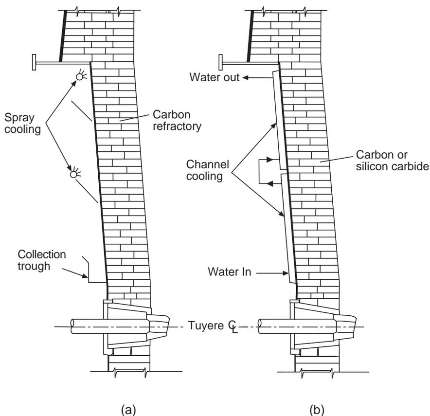
**Fig. 9.8** Cooling types for gas-tight bosh jackets: (a) spray cooling, (b) enclosed water panels or channel cooling.
