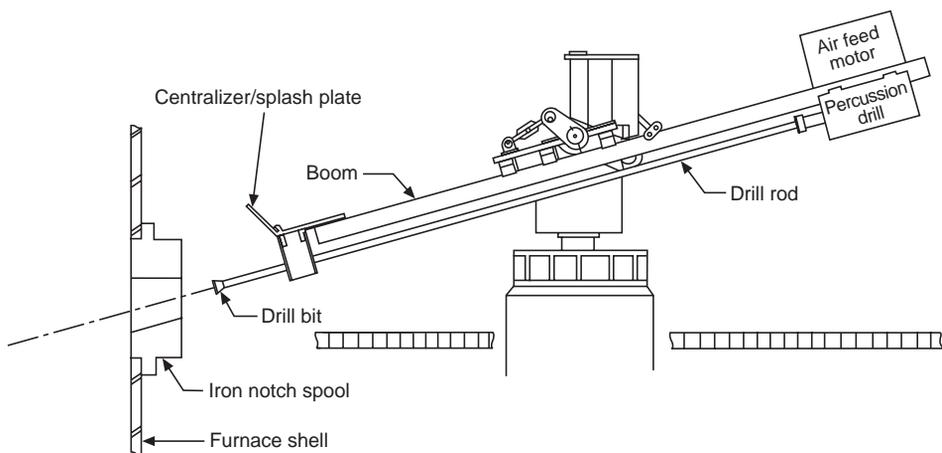
Fig. 9.49 Schematic of a typical taphole drill.
