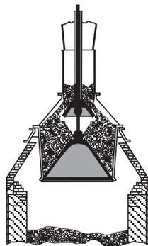
Large bell remains closed while small bell opens to admit charge to large bell hopper.
