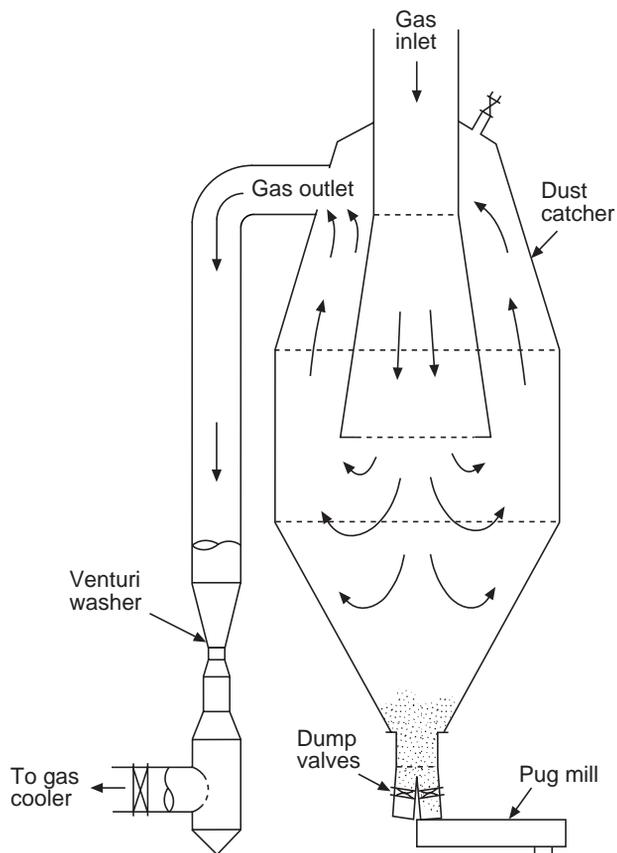
Fig. 9.30 Schematic of a dustcatcher and a venturi washer.
