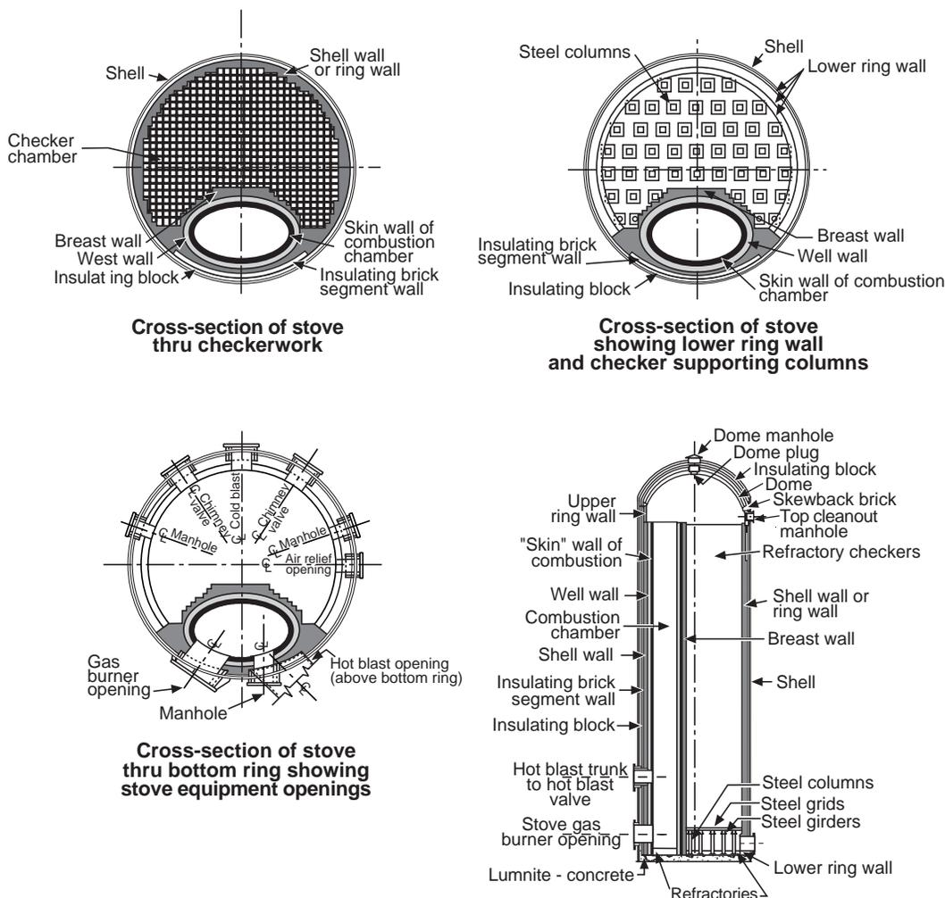
Fig. 9.34 Vertical section through a stove with cross-sectional views at several elevations.
