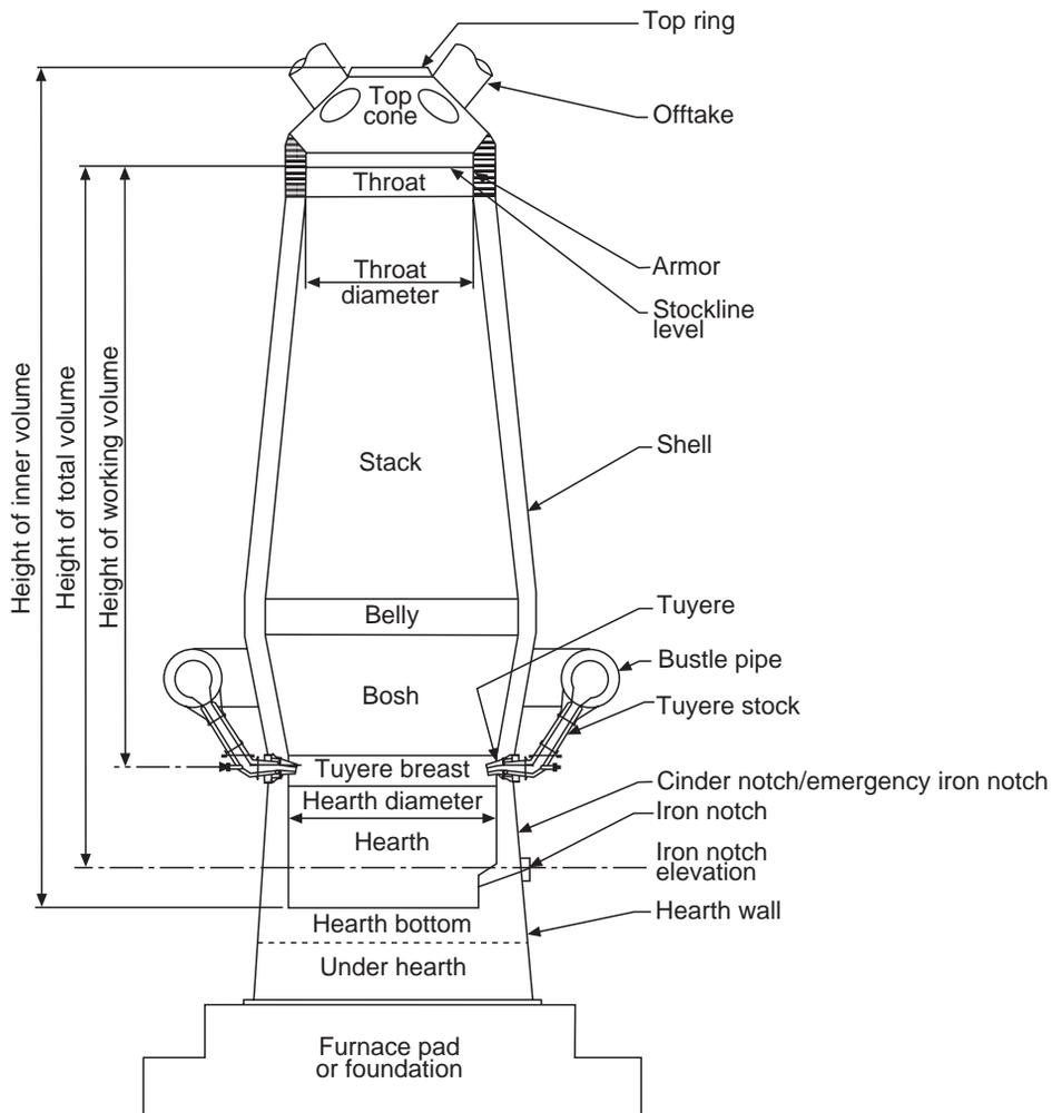
Fig. 9.1 Schematic of a blast furnace, illustrating some of the defined terms.
