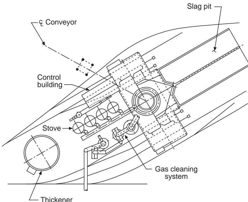
Fig. 9.47 Layout of a casthouse arrangement with two tapholes.
