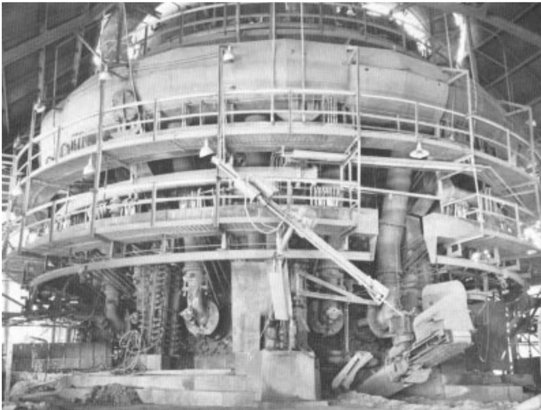
Fig. 9.51 Photograph of a blast furnace at the end of a tap with the mud gun in position at the taphole. The taphole drill is retracted and ready to be swung into position for use for the next tap.
