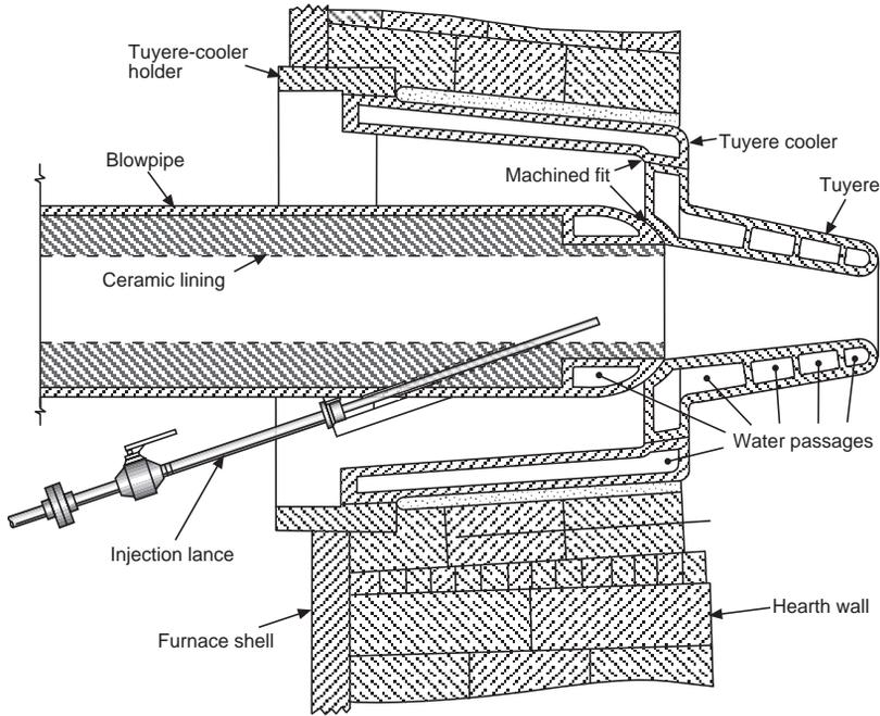
Fig. 9.6 Tuyere and blowpipe assembly.
