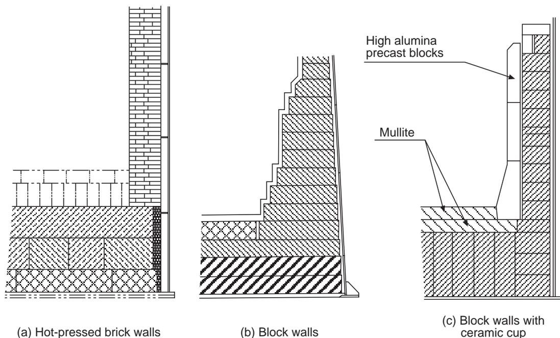
Fig. 9.3 Hearth wall refractory configurations.
