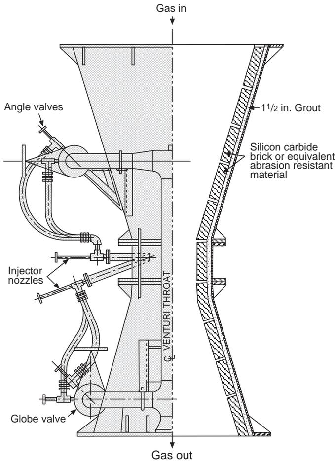
**Fig. 9.31** Schematic arrangement of a venturi-type unit for washing blast furnace gas; at right is a cut-away drawing to show the lining.
