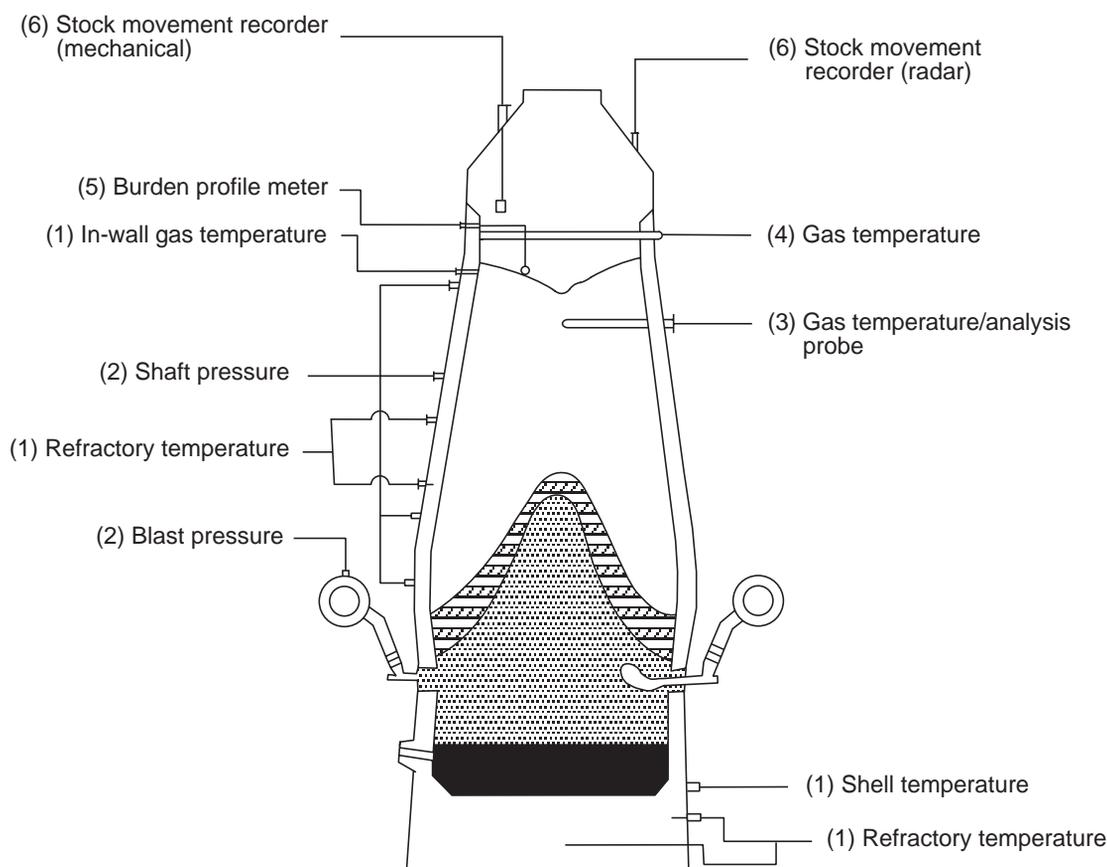
Fig. 9.59 Schematic of a well-instrumented, modern blast furnace.
