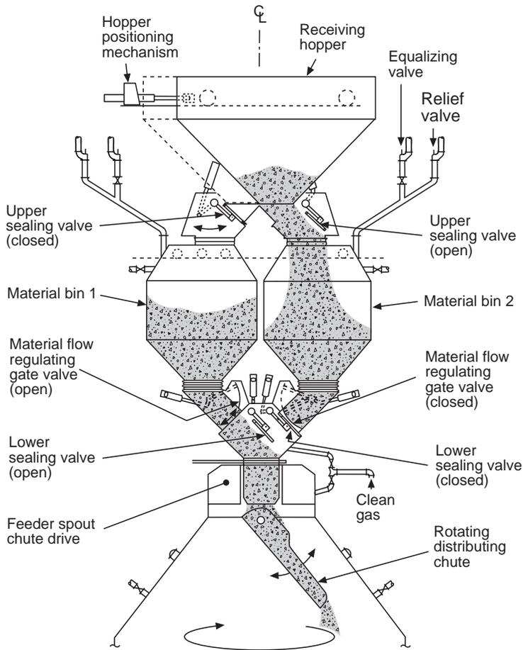
**Fig. 9.26** Schematic of a bell-less top with pressurized hoppers and a rotating distributing chute.
