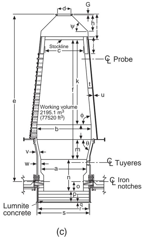
**Fig. 9.12** (a) Mantle stave cooling; (b) bosh cooling by copper staves; and (c) furnace lines of a typical, mantle-supported North American blast furnace. Dimensions for the furnace in (c) are presented in Table 9.1.
