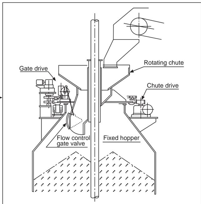
(b) Flow control gate valve of rotating chute
