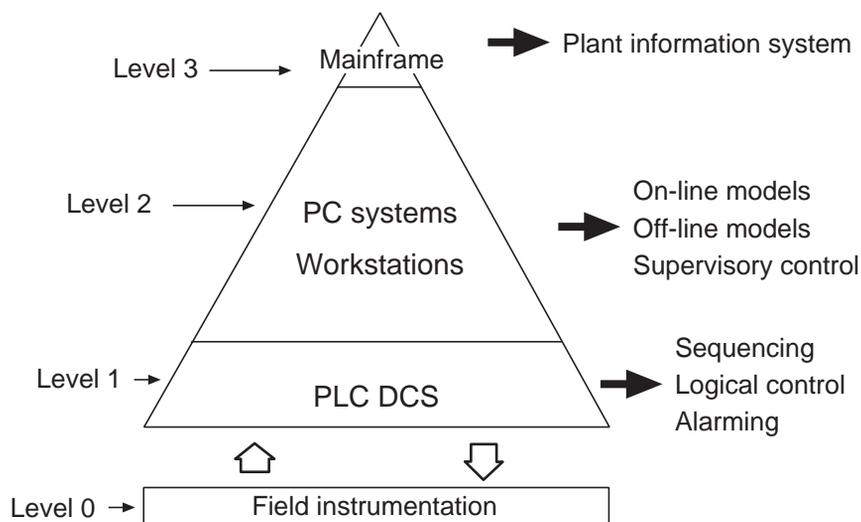
Fig. 9.57 Typical architecture for a modern process control system
