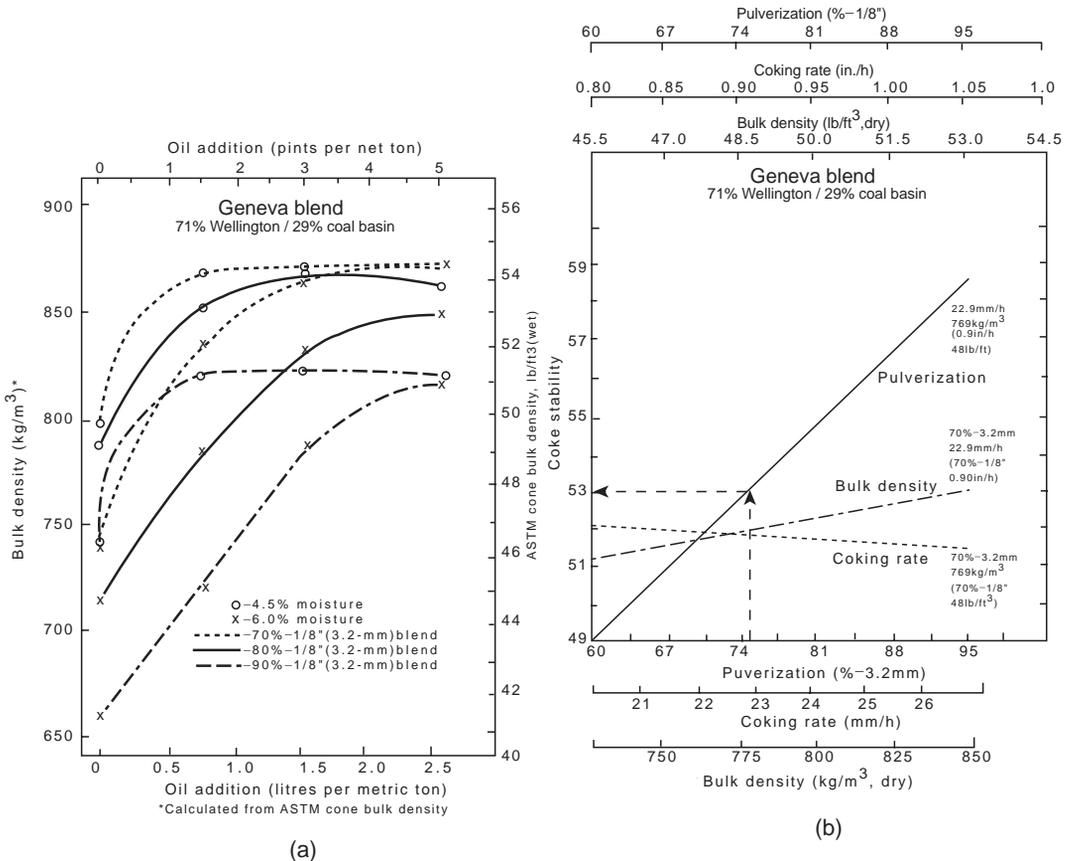
Fig. 7.20 (a) Bulk density response to oil additions for a coal blend; (b) changes in coke stability resulting from changes in coal pulverization, bulk density and coking rate.
