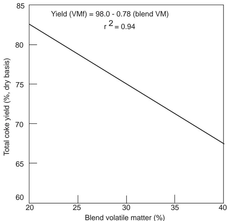
Fig. 7.9 Relationship between coal volatile matter and coke yield. (From Ref. 17)
