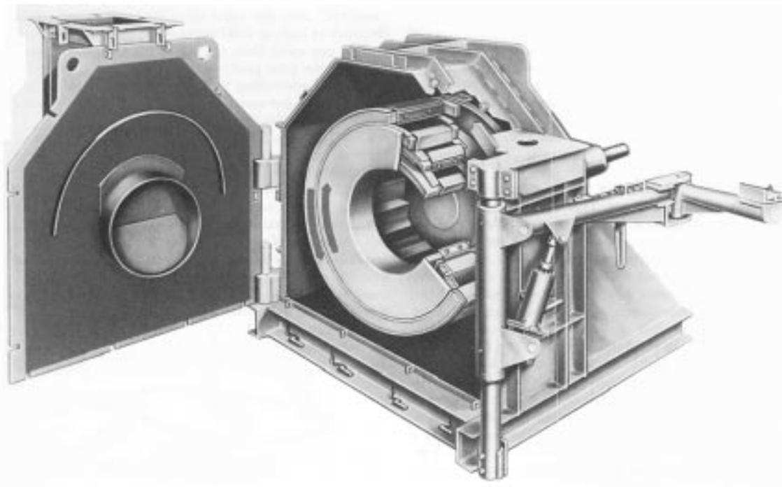
Fig. 7.18 Cut-away view of a cage mill for pulverizing coal.
