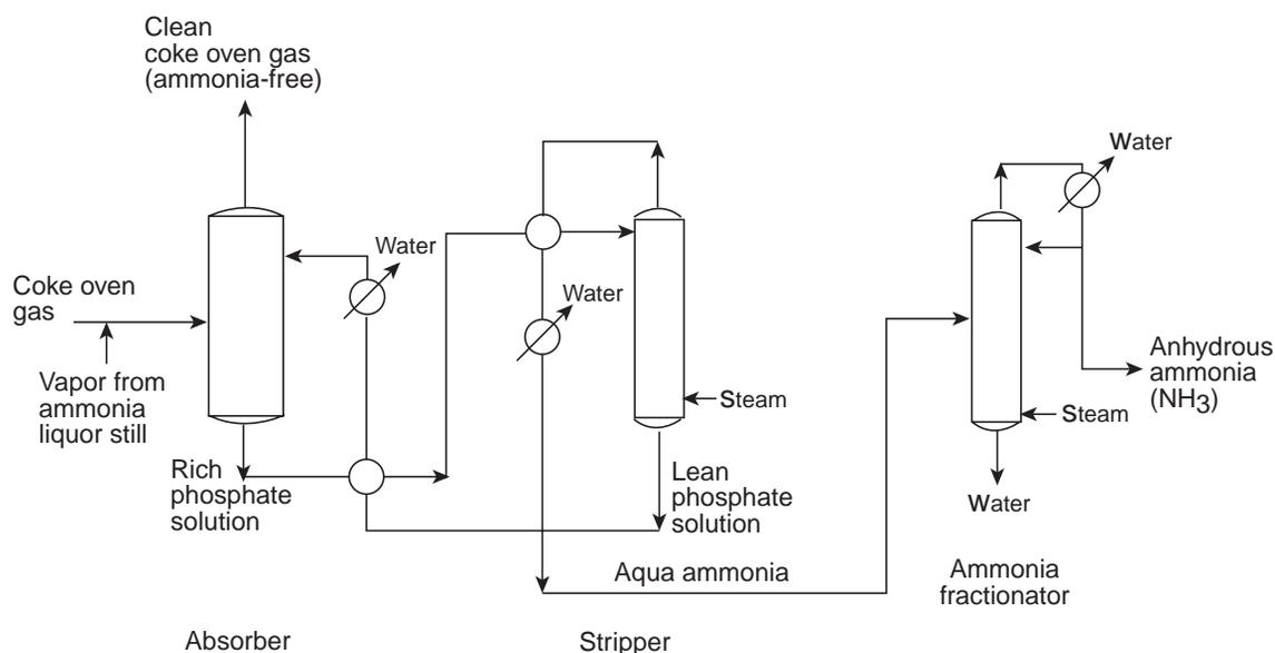
Fig. 7.104 USS PHOSAM process for producing anhydrous ammonia.
