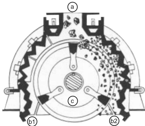
**Fig. 7.17** Reversible impactor for pulverizing coal: (a) feed chute, (b) breaker plates, (c) rotor.
