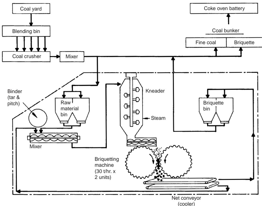
Fig. 7.57 Schematic flow of diagram of Nippon Steel's briquette blending system.
