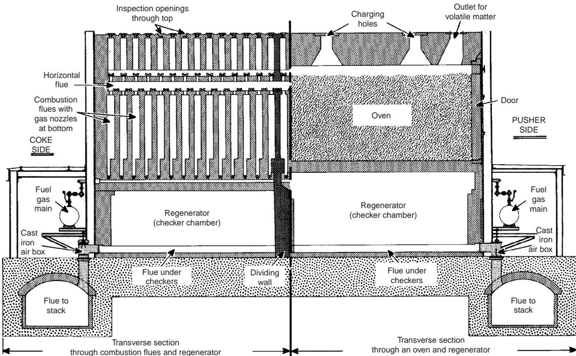
**Fig. 7.59** Transverse sections of Koppers regenerative single-divided byproduct coke oven battery. Section at left is through combustion chambers (flues), that at right is through oven chamber.
