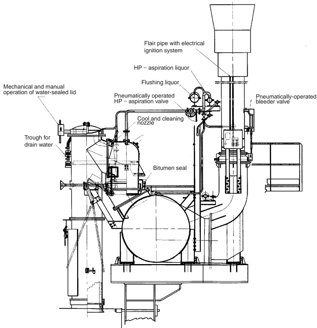
Fig. 7.85 Cross-section through the collecting main.
