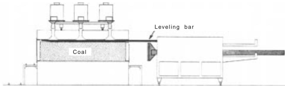
(c) The leveling door at the top of the oven door on the pusher side has been opened, and the leveling bar on the pusher has been moved back and forth across the peaked coal piles to level them. The bar next is withdrawn from the oven, the leveling door and charging holes are closed, and the coking operation begins.
