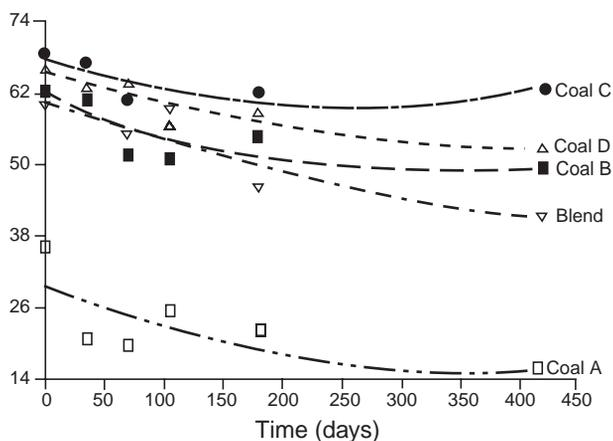
Fig. 7.12 Effect of oxidation on CSR. (From Ref. 24)
