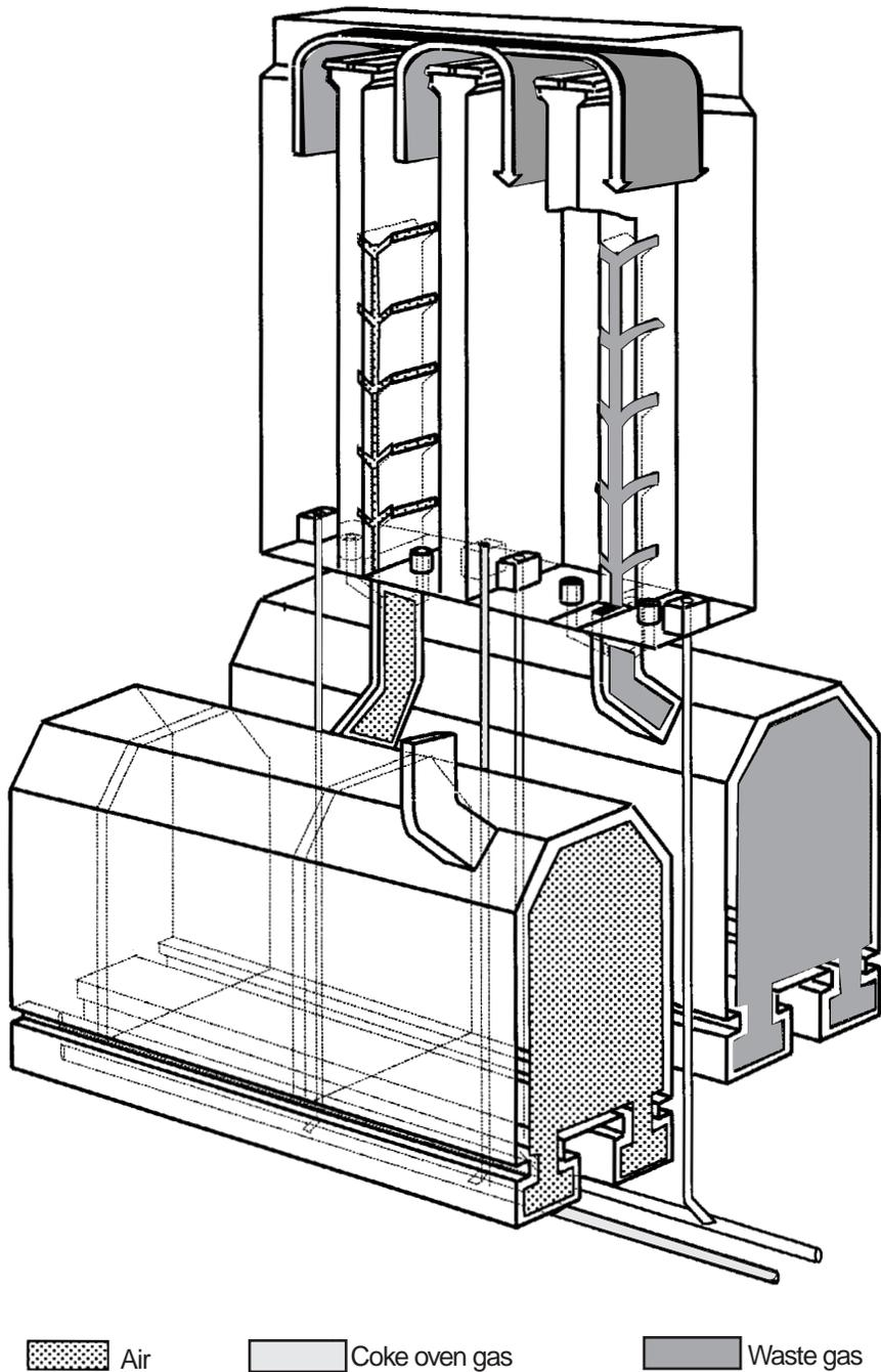
Fig. 7.76 Heating unit for a double pair flue underjet oven operating on coke oven gas.
