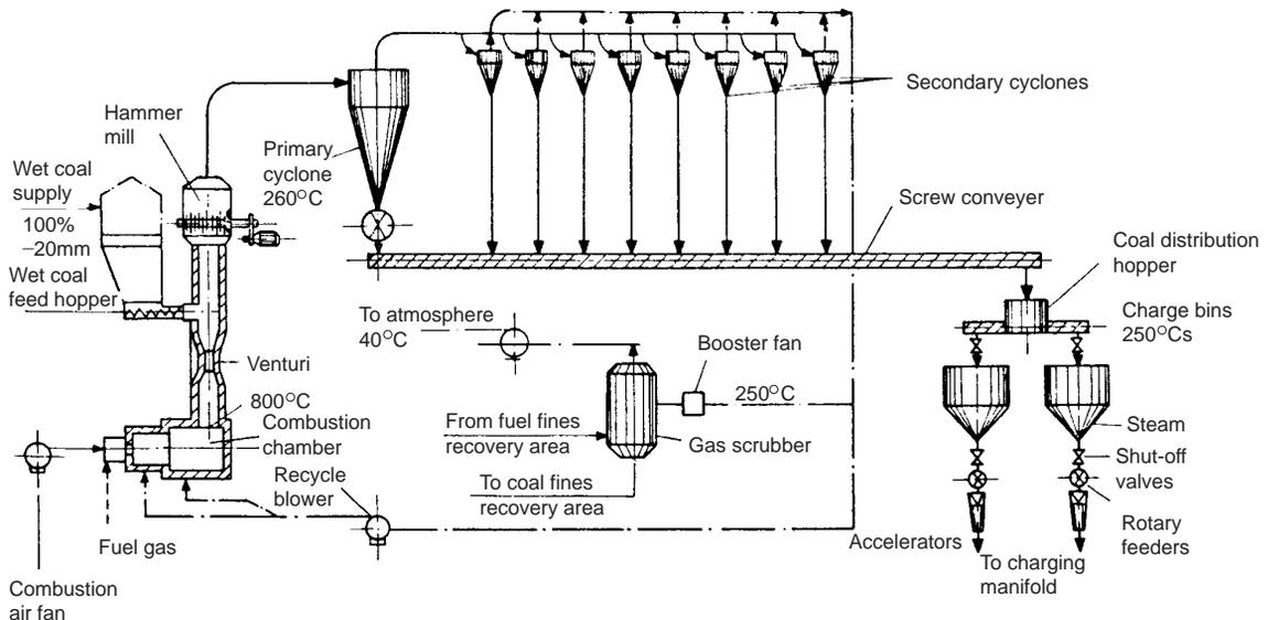
Fig. 7.53 Schematic arrangement of a Cerchar type of coal preheating plant.
