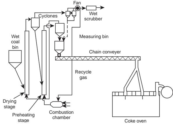
Fig. 7.52 Schematic arrangement of a Rosin-Buttner type of coal preheating unit.
