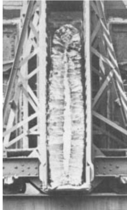
**Fig. 7.25** View of coke being pushed from oven, showing central line of cleavage and block-like structure of the coke.
