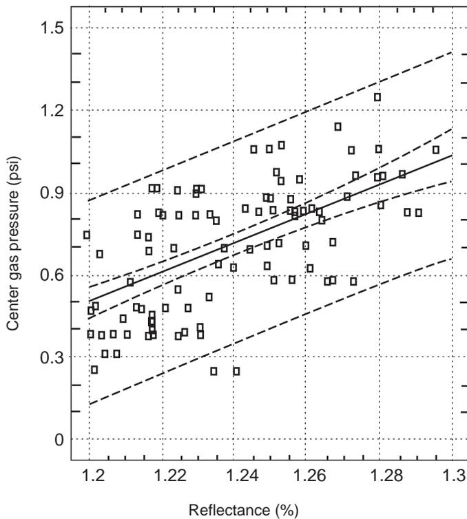
Fig. 7.11 Effect of rank on gas pressure. (From Ref. 20)
