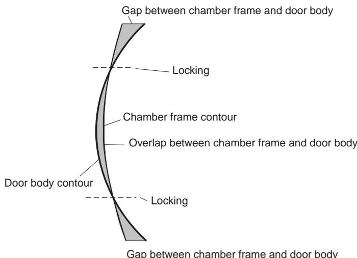
Fig. 7.86 Deformation differences between the chamber frame and the door body.
