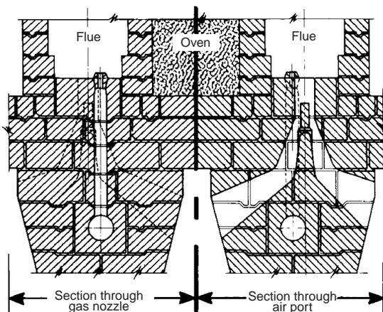
**Fig. 7.62** Enlarged sections through gas nozzles and air ports of a Koppers-Becker combination gun-flue type of byproduct coke oven, showing detail of part of Fig. 7.61(b).
