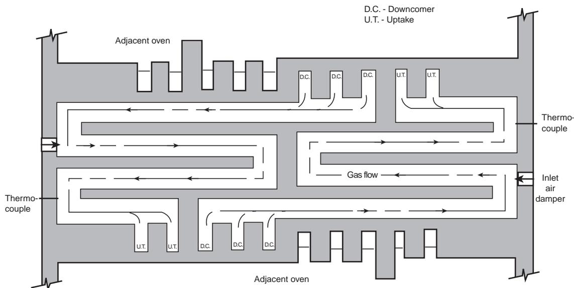
**Fig. 7.119** Sole flue arrangement.
