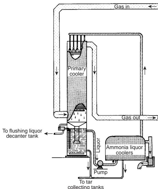
Fig. 7.95 Schematic diagram of a direct primary cooler
