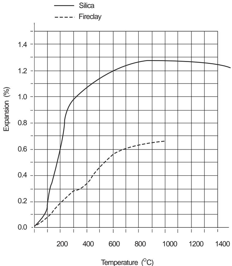
Fig. 7.78 Thermal expansion of silica and fireclay material.
