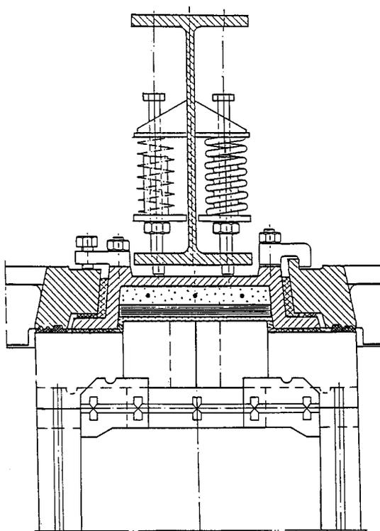
Fig. 7.84 Cross-section of the bracing system.
