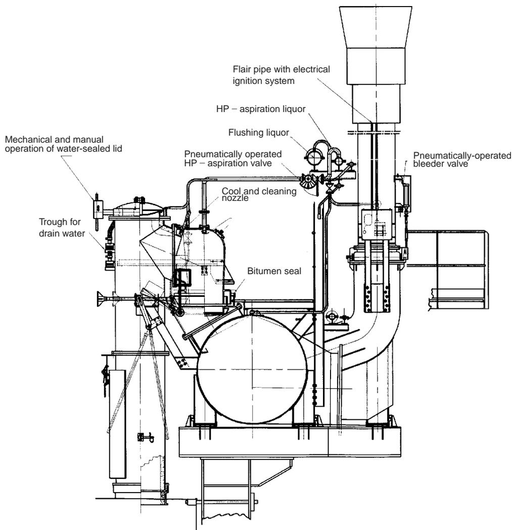
**Fig. 7.35** Thyssen Still Otto collecting main and ascension pipe with oval water-sealed cap for automatic gooseneck cleaning.
