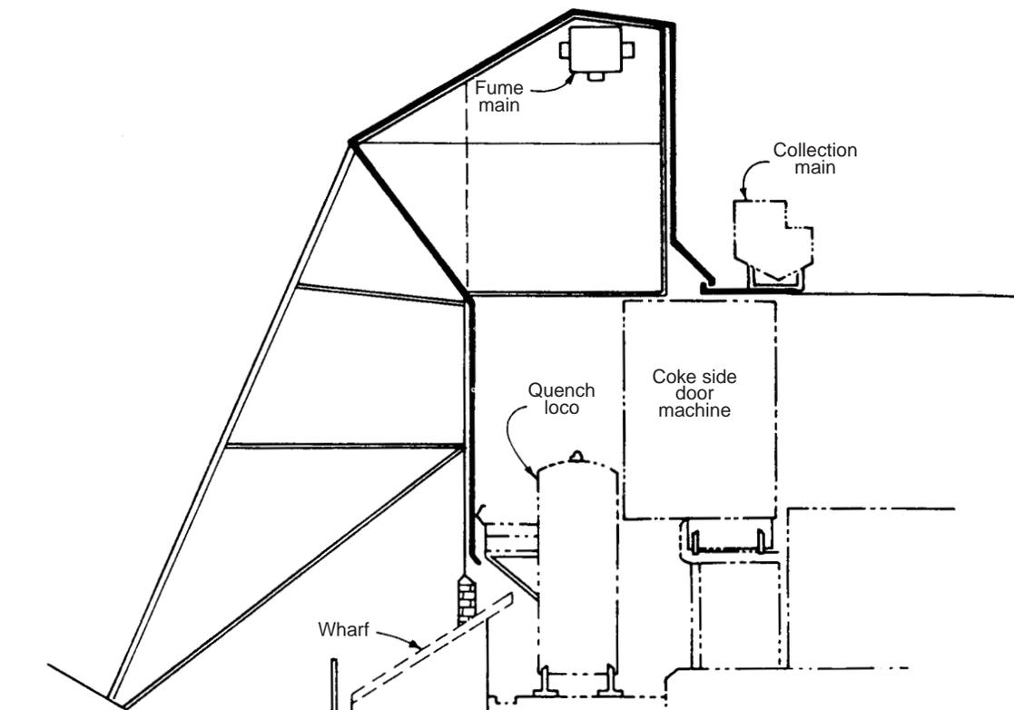
Fig. 7.47 Coke side shed for collecting emissions from a byproduct coke oven during the pushing operation.
