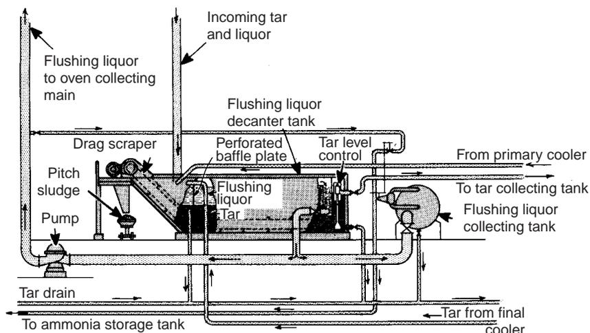
Fig. 7.91 Schematic representation of a flushing liquor decanter tank or hot tar drain tank
