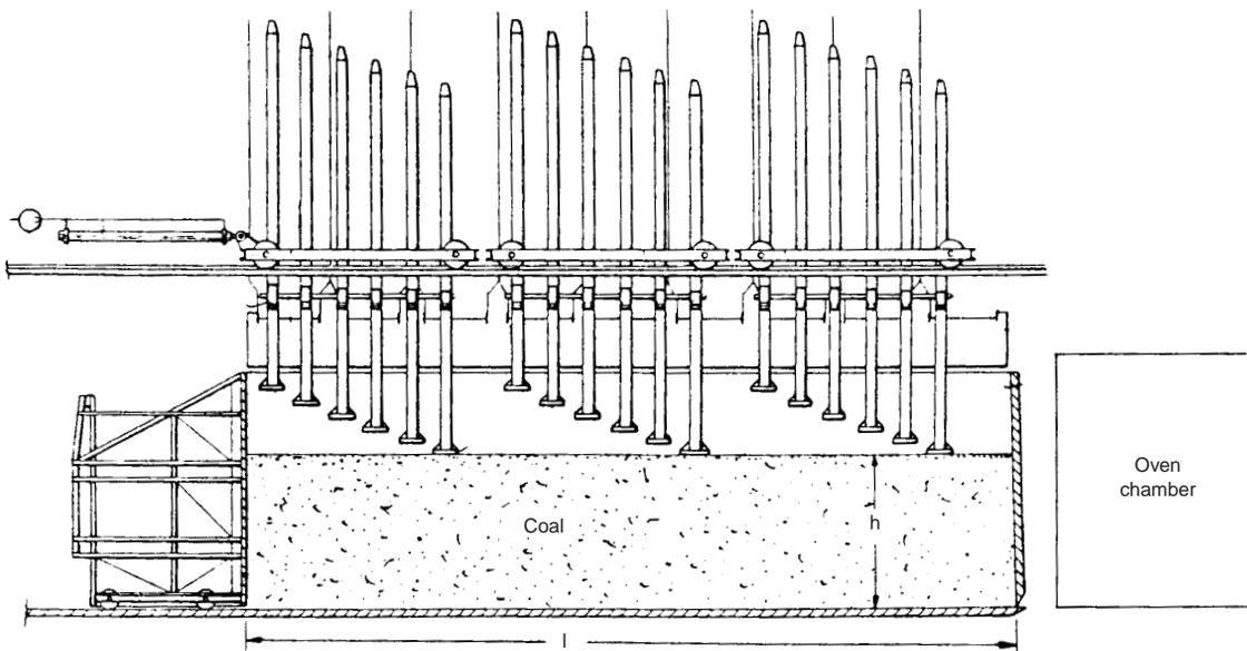
Fig. 7.55 Schematic section showing side view of a stamp charging unit.
