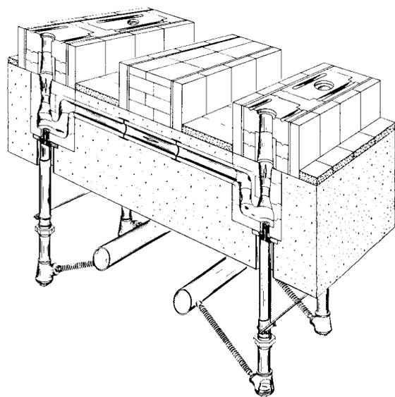
Fig. 7.68 Waste-gas recirculating duct arrangement for a Koppers-Becker low-differential combination underjet byproduct coke oven battery.
