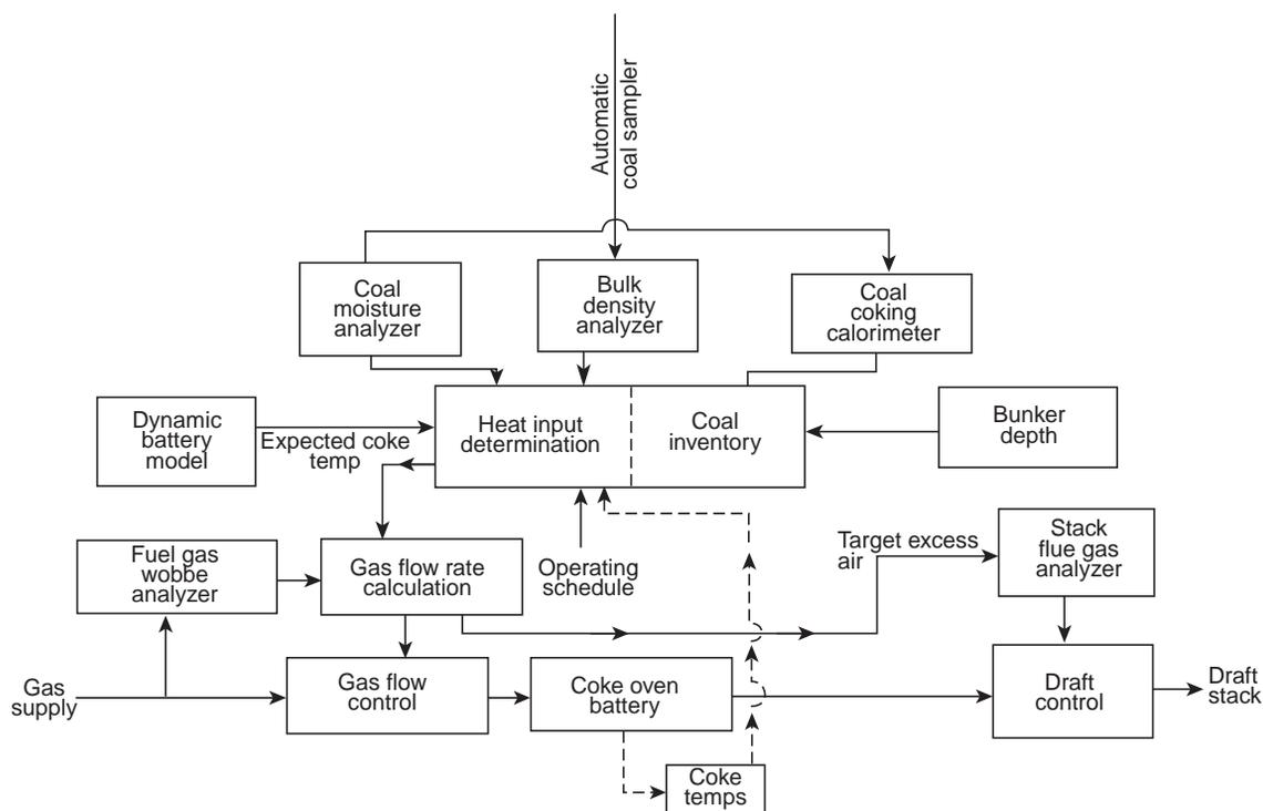
Fig. 7.46 Feedforward coke oven battery heating control system.
