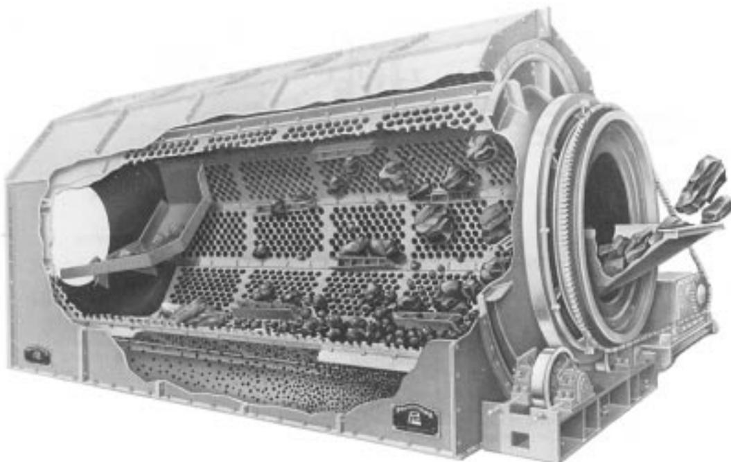
**Fig. 7.15** Cut-away view of a rotary Bradford breaker.
