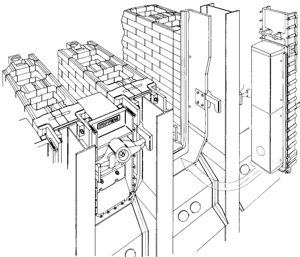
**Fig. 7.66** Section showing arrangement of flue ends, door and jambs of a Koppers-Becker low-differential combination underjet coke oven battery.
