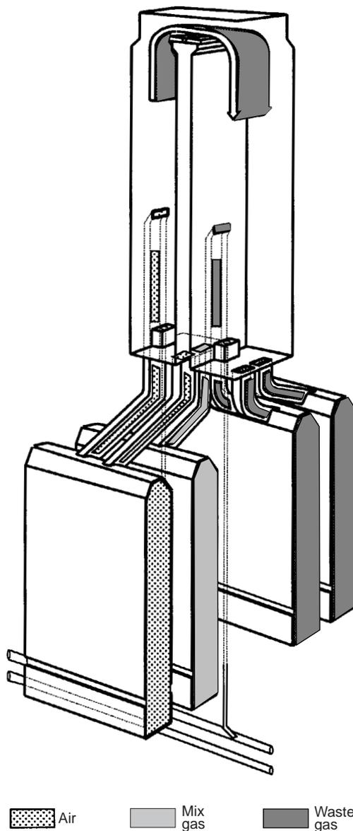
Fig. 7.73 TSOA twin-flue heating unit system operating on mix gas.
