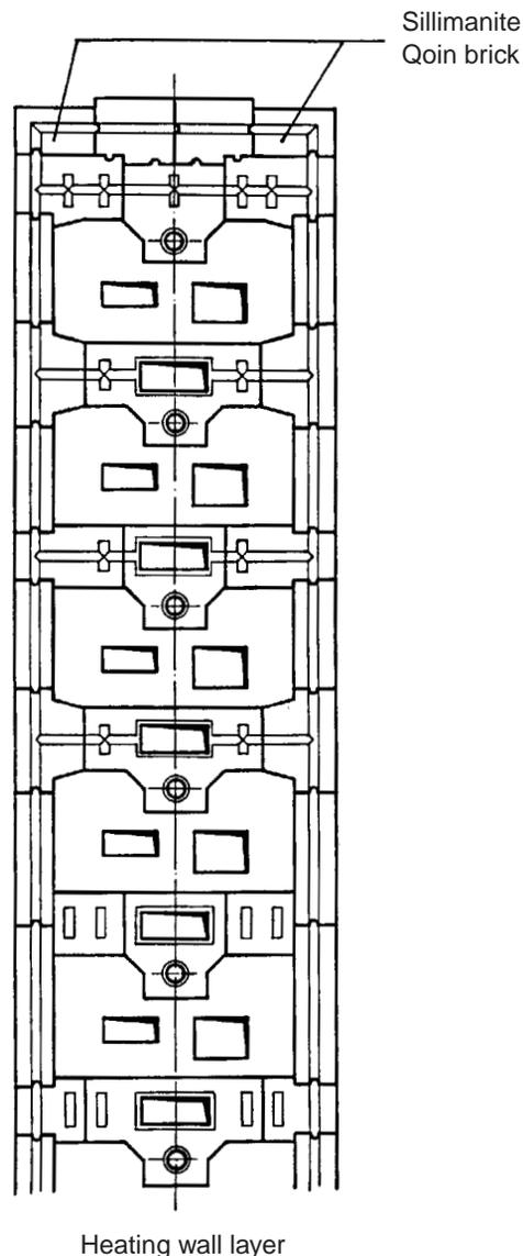
Fig. 7.80 Wall bond for a twin flue underjet oven system.
