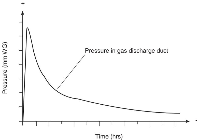
Fig. 7.87 Pressure development in the gas discharge duct after the start of the coking time.
