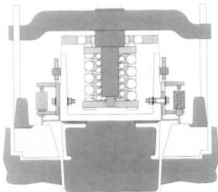
**Fig. 7.34** Cross-section through the Thyssen Still Otto Autoseal™ door with automatic adjustment of the contact pressure by means of compressing spring system.
