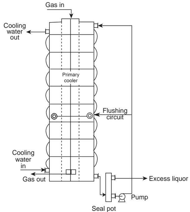
Fig. 7.97 Schematic diagram of a horizontal tube type indirect cooler.
