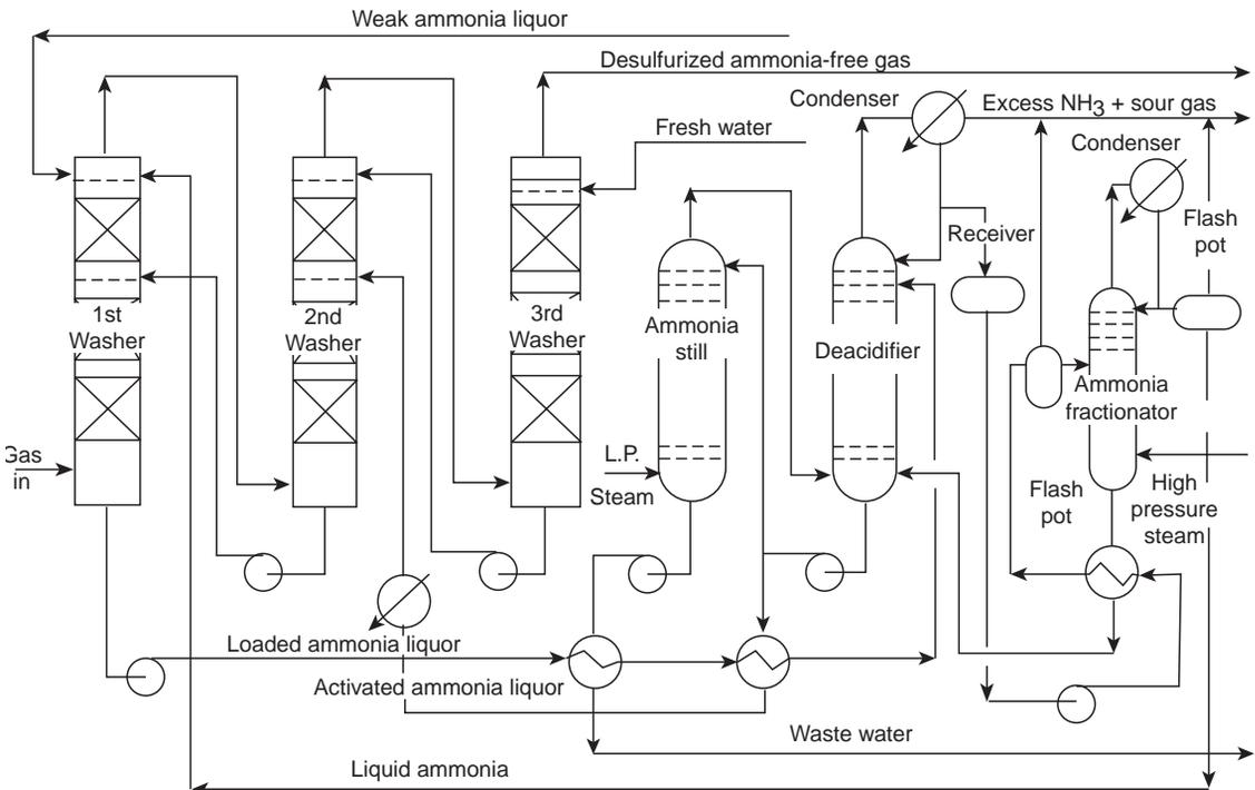
Fig. 7.116 Flowsheet of the DESULF process.
