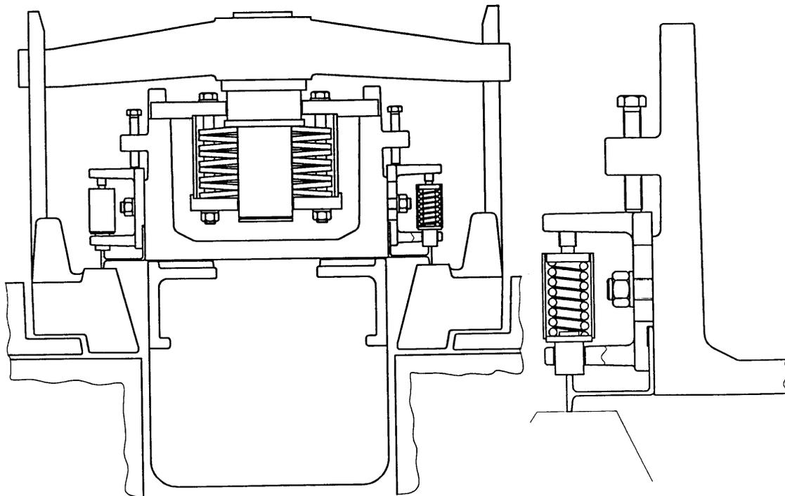
Fig. 7.89 Cross-section of a door and sealing element.
