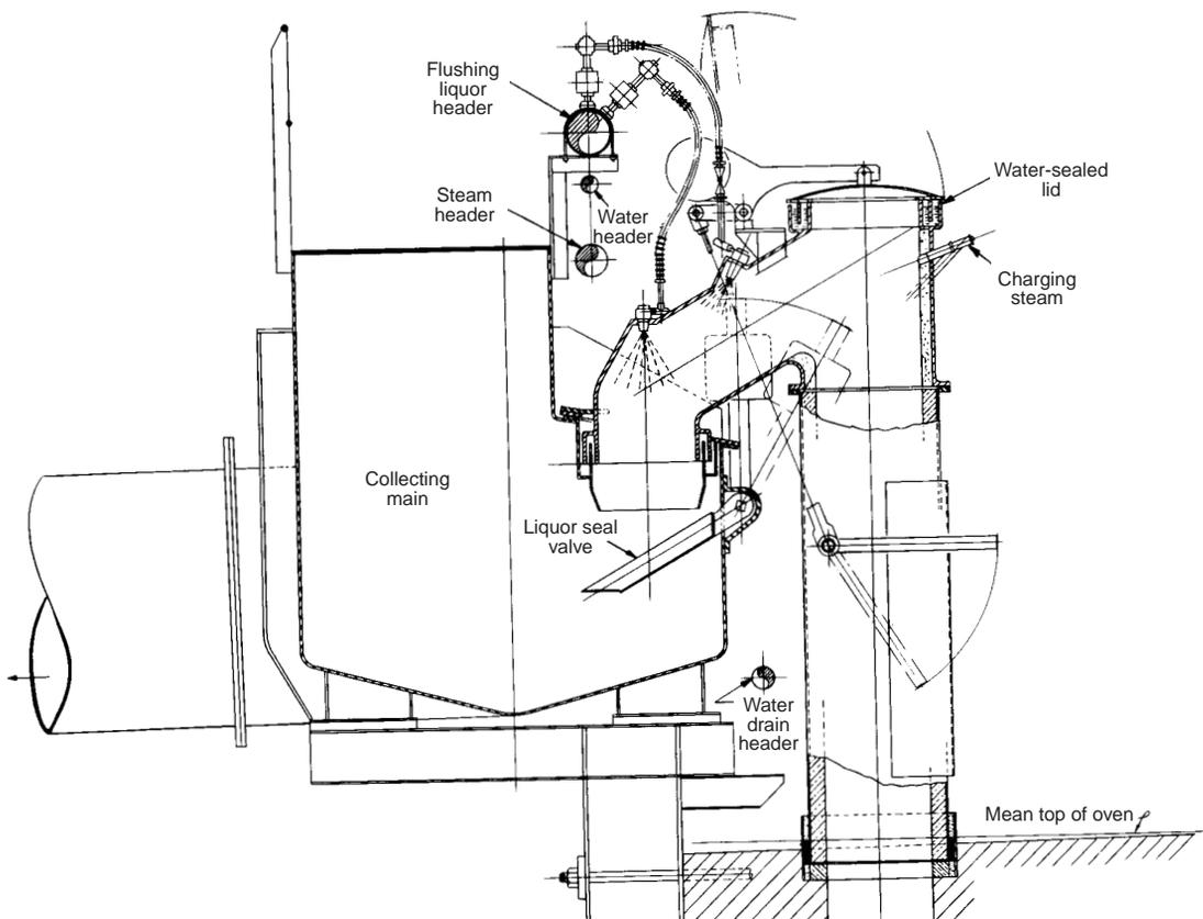
Fig. 7.70 Cross-section through a collecting main and ascension pipe on a byproduct coke oven charged with wet coal.
