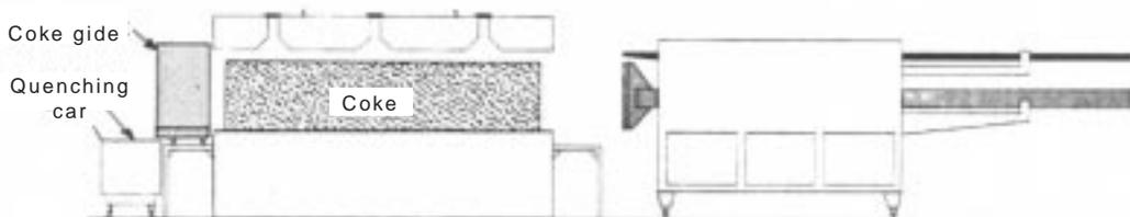
(d) Coking of the coal originally charged into the oven has been completed (in about 18 hours) and the oven is ready to be "pushed." The oven doors are removed from each end, and the pusher, coke guide and quenching car are moved into position.
