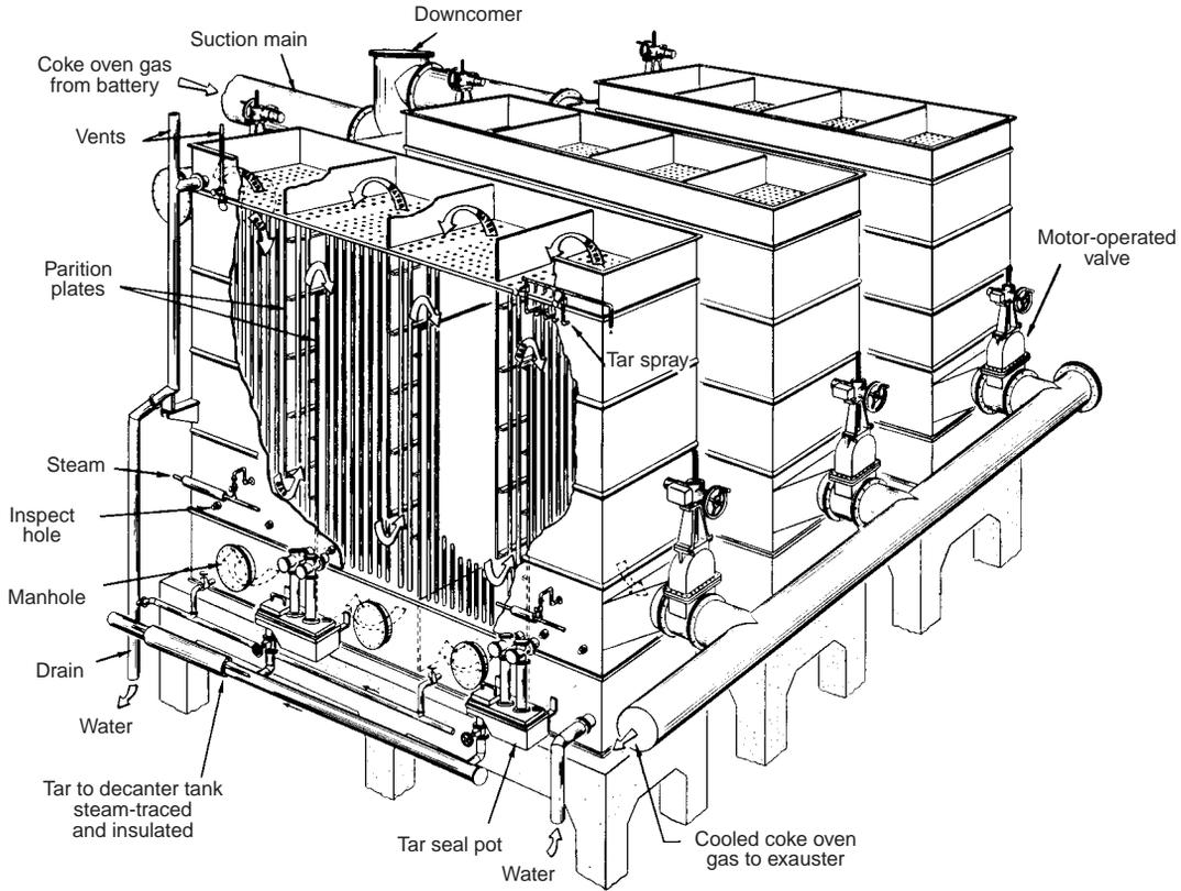
Fig. 7.96 Three indirect primary coolers of the vertical tube type.
