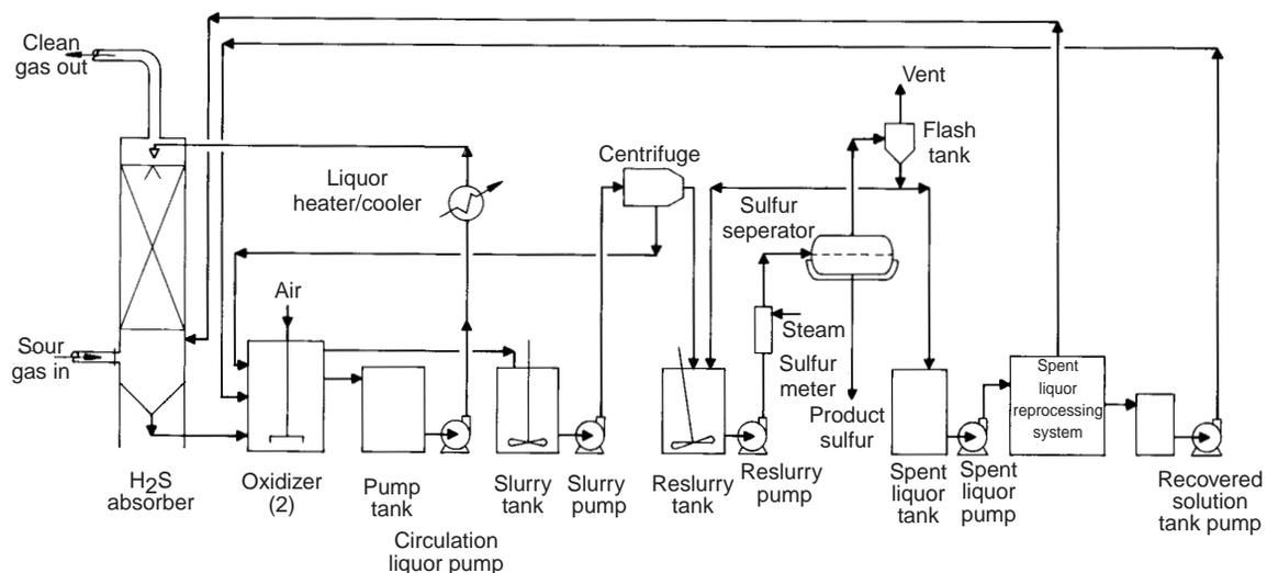
Fig. 7.113 Flow diagram of the Holmes-Stretford process for desulfurization of coke oven gas..
