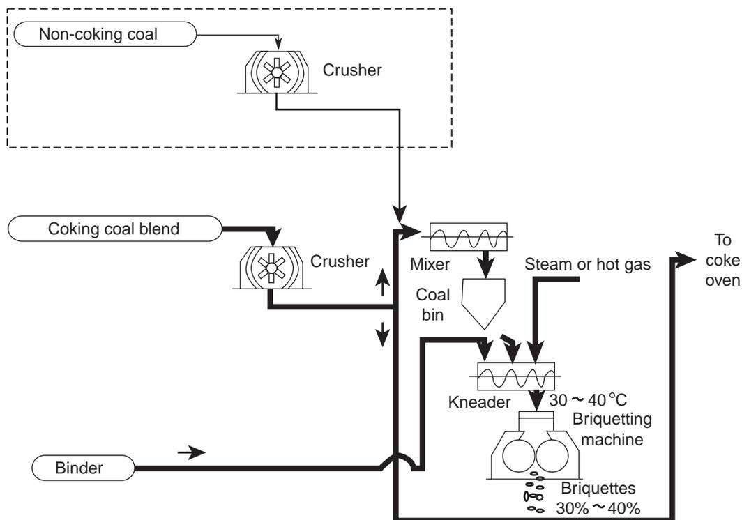
Fig. 7.56 Simplified flow diagram of Sumi-coal system.
