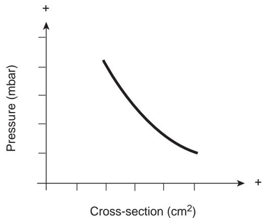
Fig. 7.88 Dependence of gas pressure on the gas discharge duct cross-section.
