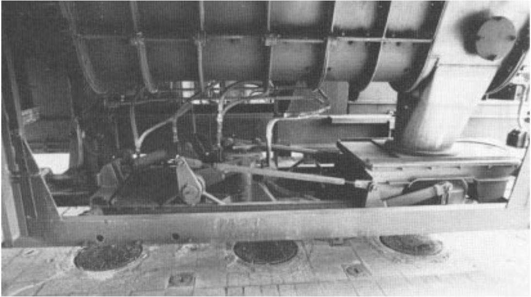
**Fig. 7.39** View of an automatic charging hole lid lifter assembly as mounted on a coal charging car.
