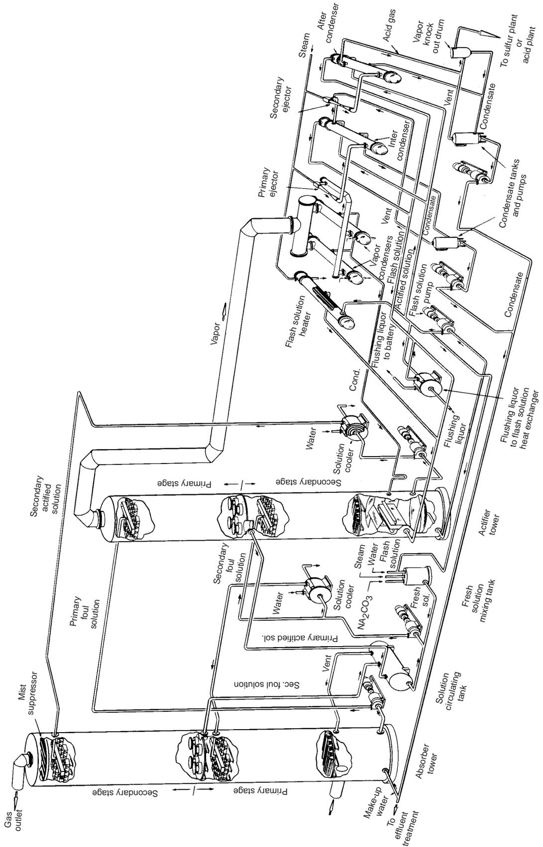
Fig. 7.111 Flow diagram of a two-stage vacuum carbonate process for removal of hydrogen sulfide from coke oven gas.
