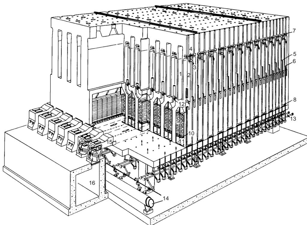
**Fig. 7.69** Sectional view of a Koppers twin-flue underjet byproduct coke oven battery. Legend: 1. oven; 2. burning flue; 3. waste-gas flue; 4. turnaround; 5. high gas port; 6. low gas port; 7. differential heating flue; 8. recirculating duct; 9. checker brick; 10. sole-flue ports; 11. sole flue; 12. air port; 13. rich-gas manifolds; 14. rich-gas main; 15. air and waste-heat boxes; 16. waste-heat flue.
