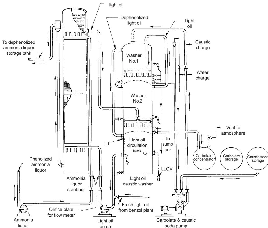
Fig. 7.105 Diagrammatic representation of the equipment for recovery of phenol by the solvent extraction process.
