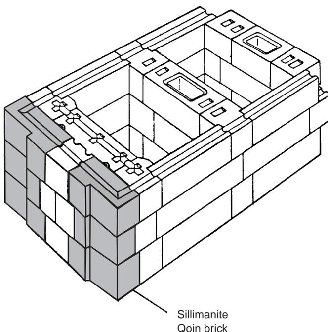
Fig. 7.82 End flue design, wall perspective.
