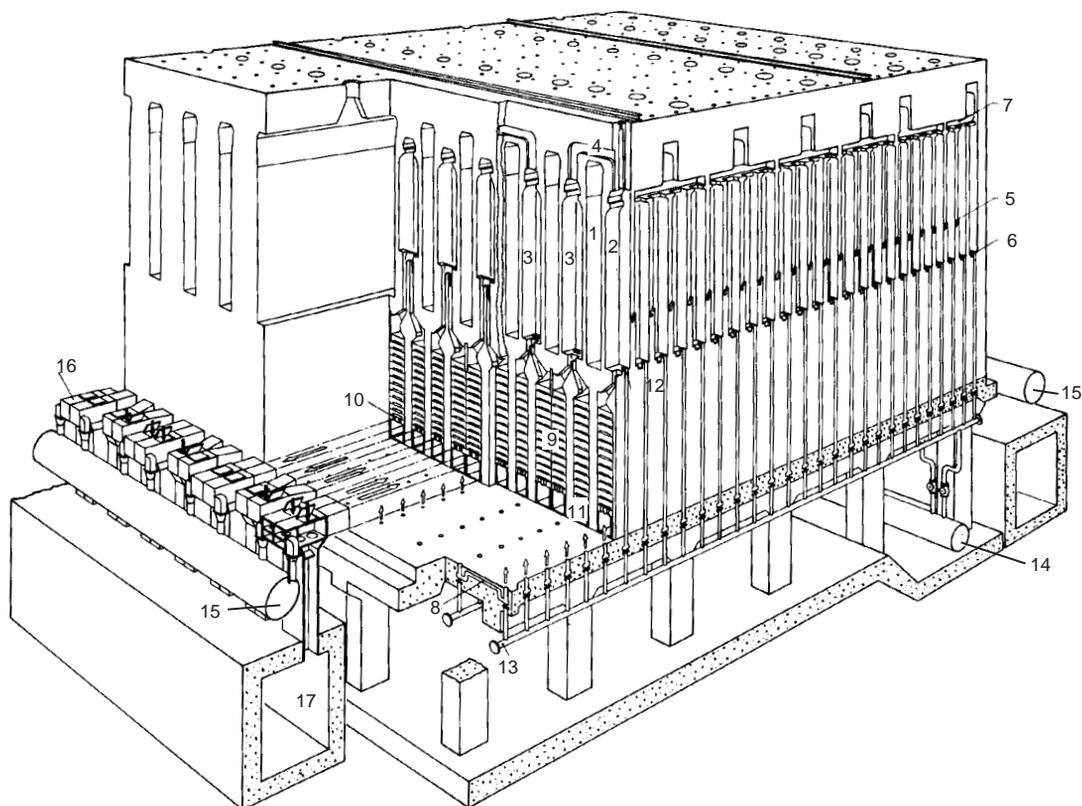
**Fig. 7.67** Sectional view of a Koppers-Becker low-differential combination underjet coke oven battery operating on rich gas. Legend: 1. oven; 2. burning flue; 3. waste-gas flue; 4. cross-over flue; 5. high air port; 6. low air port; 7. horizontal collecting flue; 8. recirculating duct; 9. checker brick; 10. sole-flue parts; 11. sole flue; 12. gas port; 13. rich-gas manifold; 14. rich-gas main; 15. blast furnace gas main; 16. gas or air and waste heat boxes; 17. waste heat flue.
