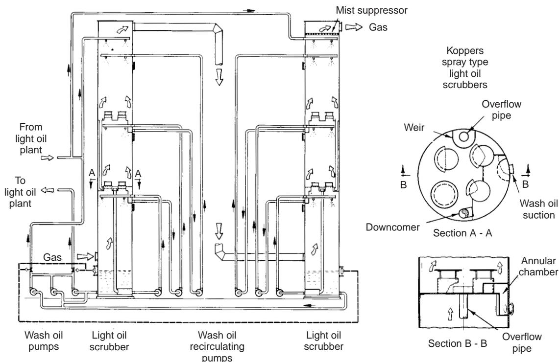
Fig. 7.110 Flow diagram of spray-type light oil scrubbers.
