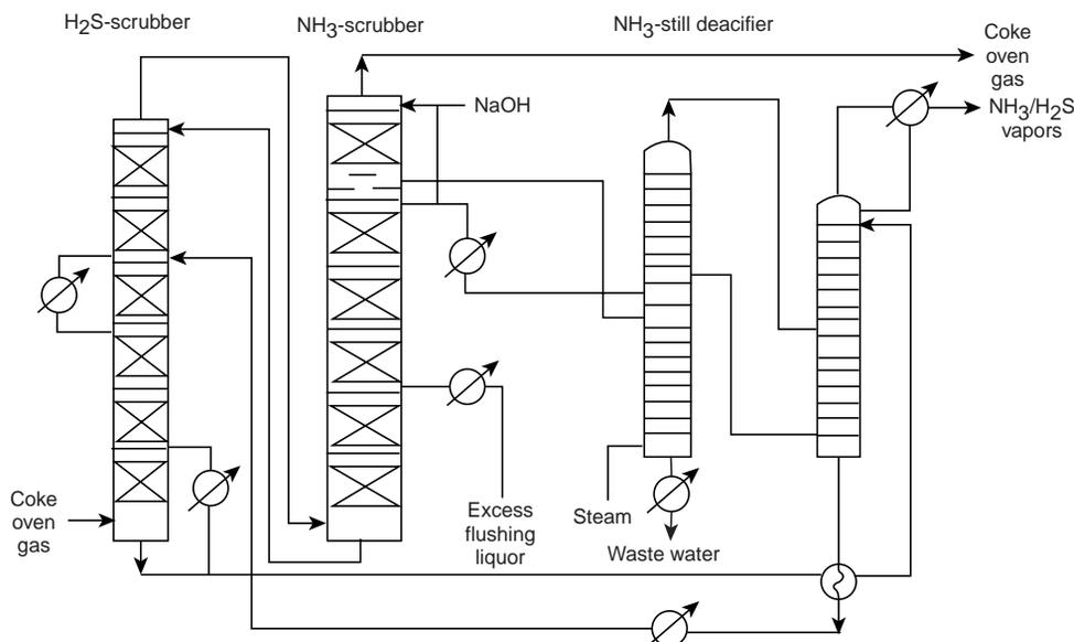
Fig. 7.114 Schematic of the ammonia/hydrogen sulfide circulation scrubbing process.
