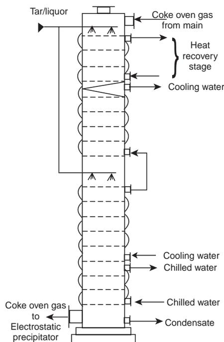
Fig. 7.98 Indirect primary cooler
