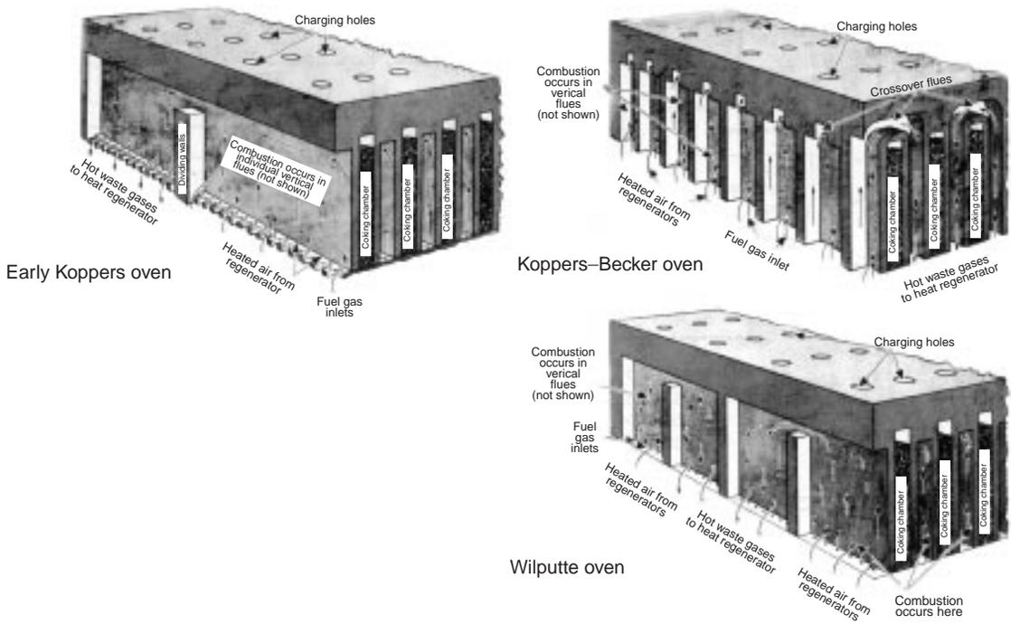
**Fig. 7.58** Schematic representation of the differences in firing methods employed in the three most common types of byproduct coke ovens used in the United States. Individual flues are not shown. The firing procedures shown are for a single phase of heating which is reversed at the end of a specified period, at which time the flow directions indicated by the arrows become reversed.
