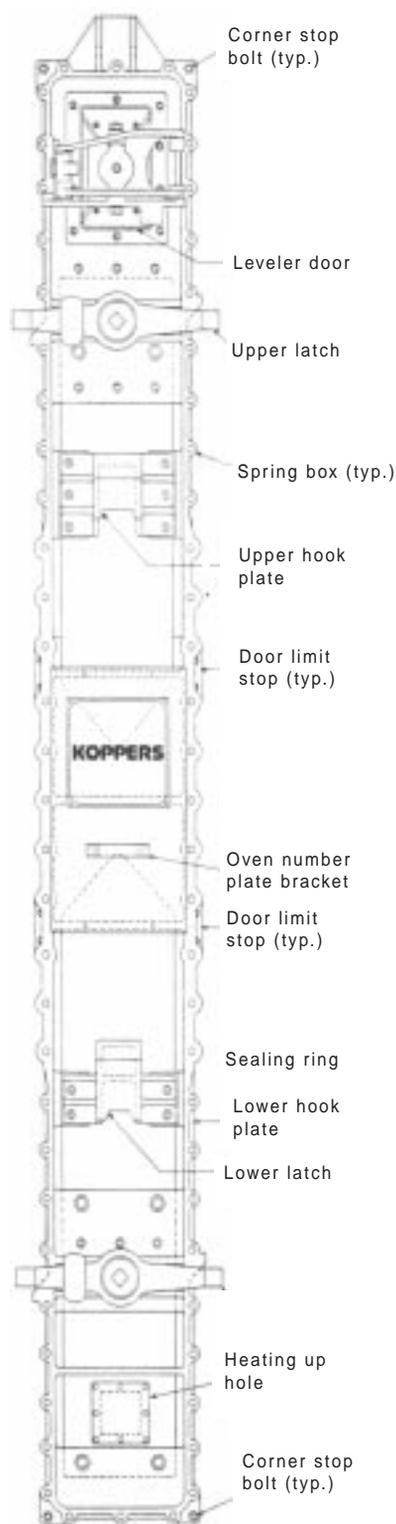
Fig. 7.26 Face view of a Koppers coke oven door of the self-sealing type.
