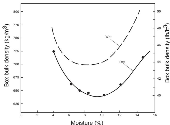
Fig. 7.19 Effect of moisture content on the bulk density of selected (Concord) coal.
