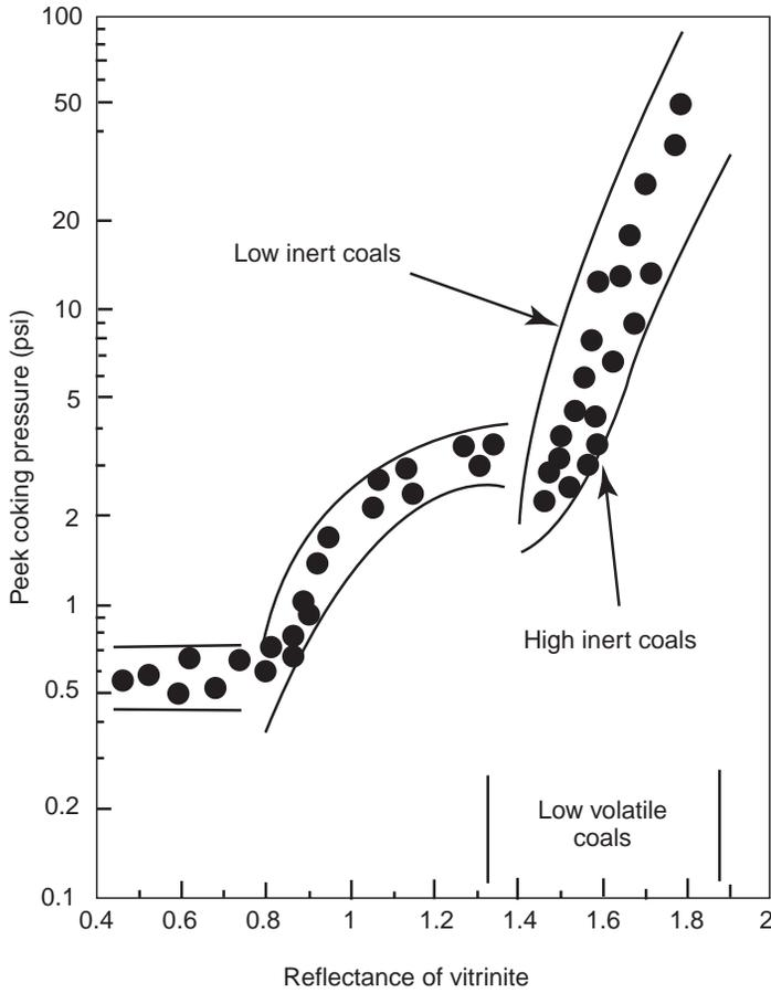
Fig. 7.10 Effect of coal rank and coal type on wall pressure. (From Ref. 19)
