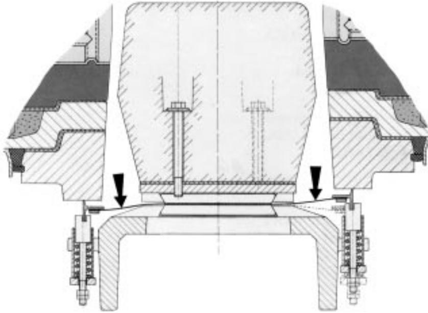
Fig. 7.31 Cross-section of Krupp-Uhde door.
