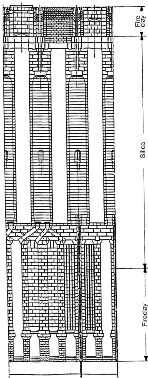
Fig. 7.79 Refractory cross-section of a twin flue underjet compound oven.
