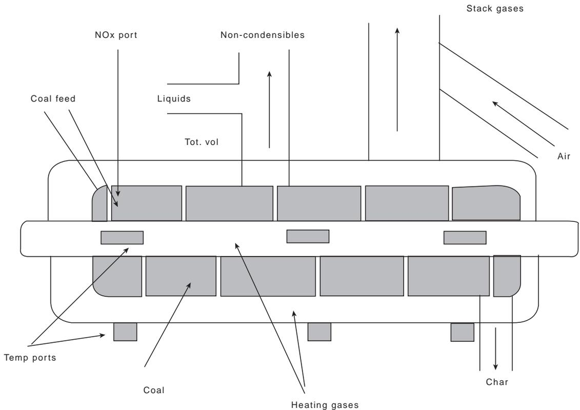
Fig. 7.124 Antaeus pyrolyzing reactor vessel.
