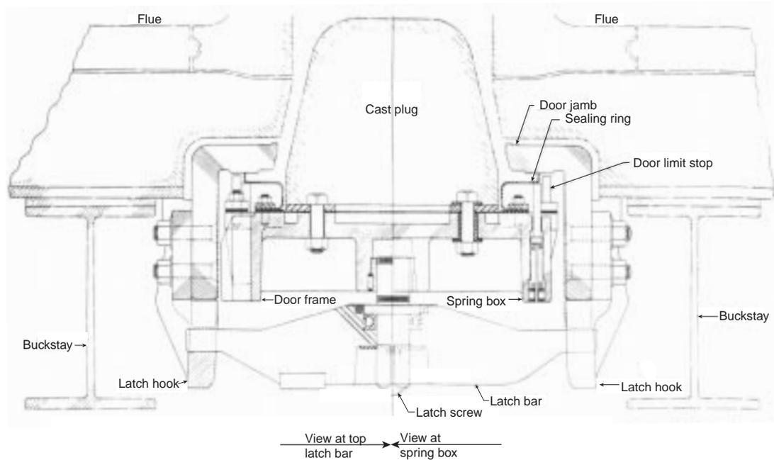
Fig. 7.27 Horizontal section of the self-sealing coke oven door shown in Fig. 7.26.
