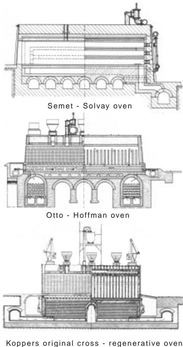
**Fig. 7.23** Early designs of recovery type coke ovens, not to same scale.
