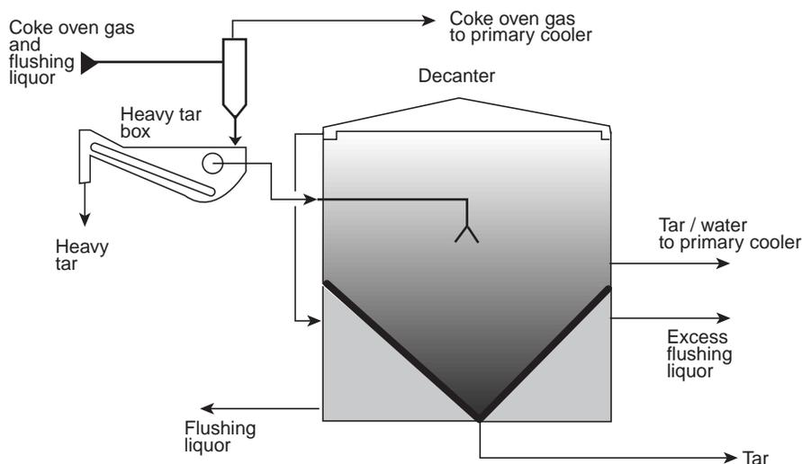
Fig. 7.92 Flushing liquor handling system with a circular decanting tank
