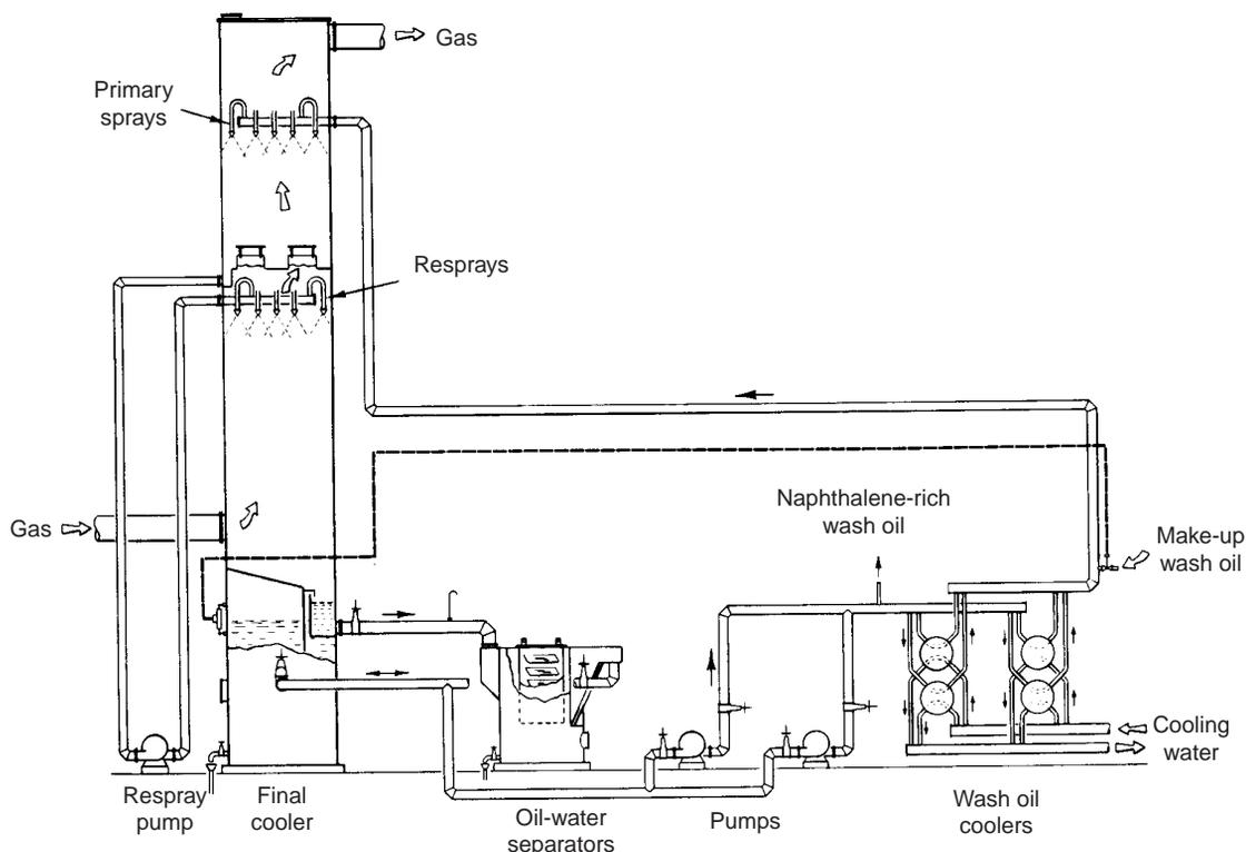
Fig. 7.108 Final cooler of the wash oil spray type
