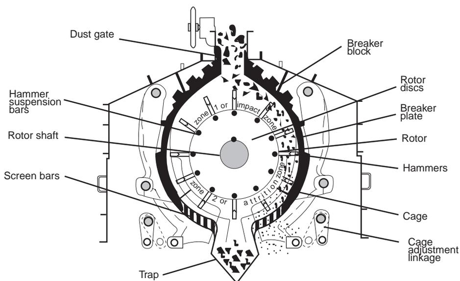
Fig. 7.16 Sectional view of a reversible hammer mill.
