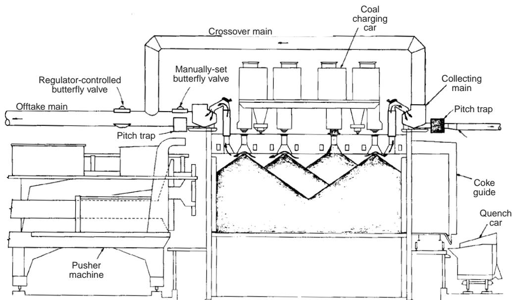
Fig. 7.71 Schematic arrangement of a coke oven equipped for staged charging or sequenced charging
