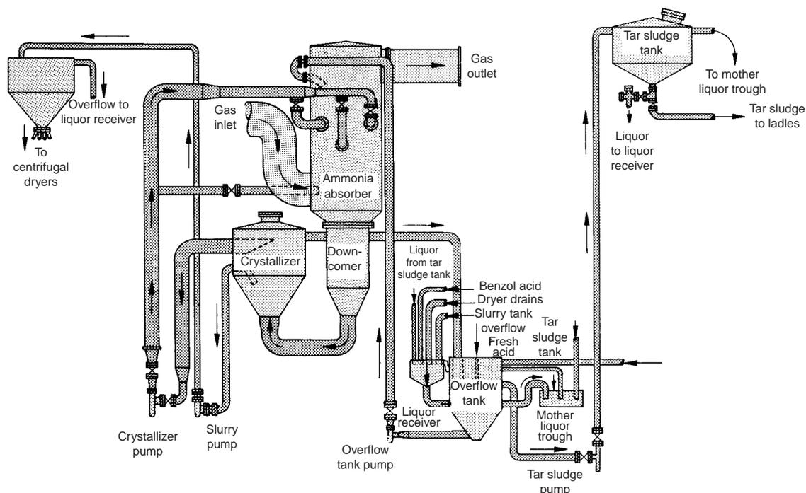
Fig. 7.102 Schematic flowsheet of the operation of an Otto spray-type absorber for the recovery of ammonia as ammonium sulfate.
