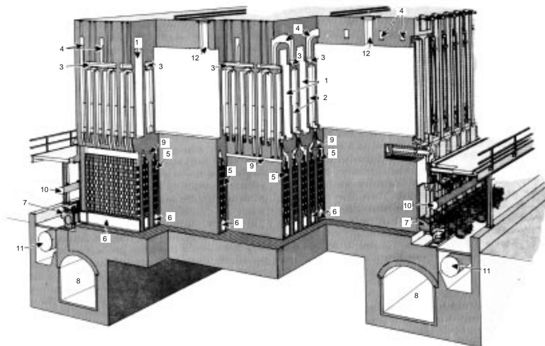
**Fig. 7.60** General perspective cut-away section of Koppers-Becker combination ovens with gun-flue heating facilities (see Fig. 7.63 for underjet-fired type). Legend: 1. oven chamber; 2. vertical combustion flues; 3. horizontal flues; 4. cross-over flues; 5. regenerators; 6. oven sole flues; 7. gas and air connections to waste-gas flue; 9. gas ducts for coke oven; 10. oven gas main; 11. blast furnace gas main; 12. charging holes.
