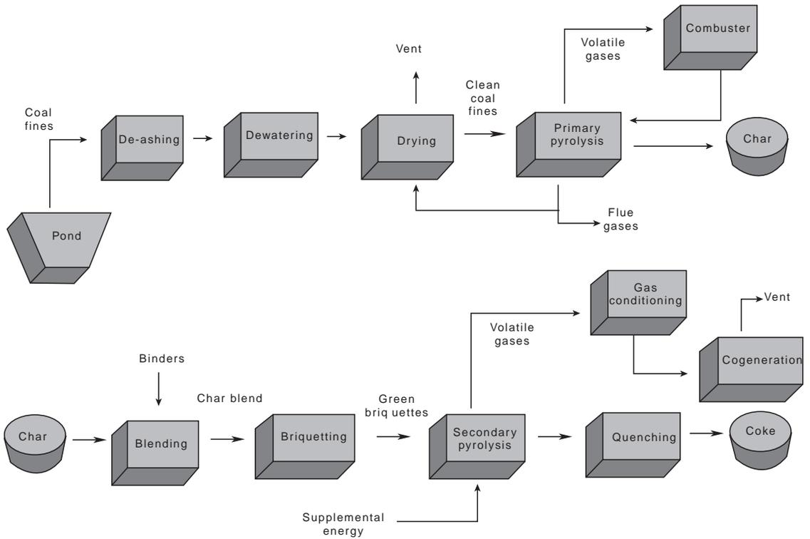
Fig. 7.123 Schematic of the Antaeus Continuous Coke<sup>SM</sup> process.
