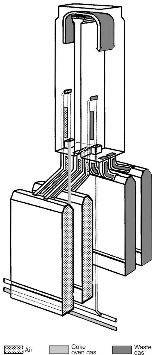
Fig. 7.72 TSOA twin-flue heating unit system operating on coke oven gas.
