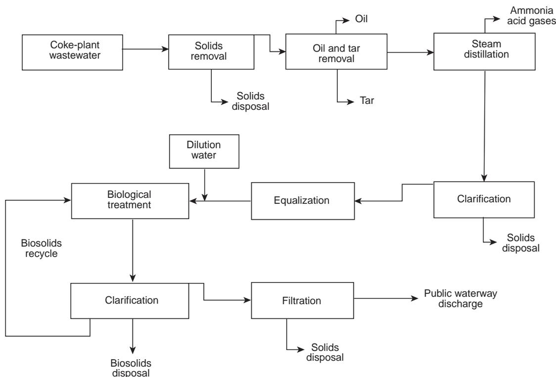
Fig. 7.117 Simplified diagram of a system for biological treatment of coke plant wastewaters.
