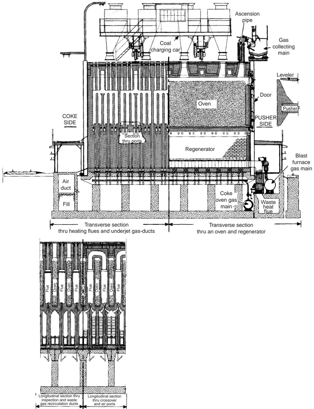
Fig. 7.63 Transverse and longitudinal sections through Koppers-Becker combination gun-flue type of byproduct coke oven, showing detail of part of Fig. 7.61(b).
