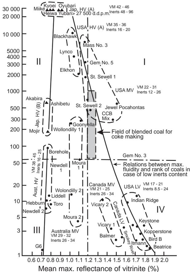
Fig. 7.6 D130/15 Prediction using reflectance and maximum fluidity. (From Ref. 13)
