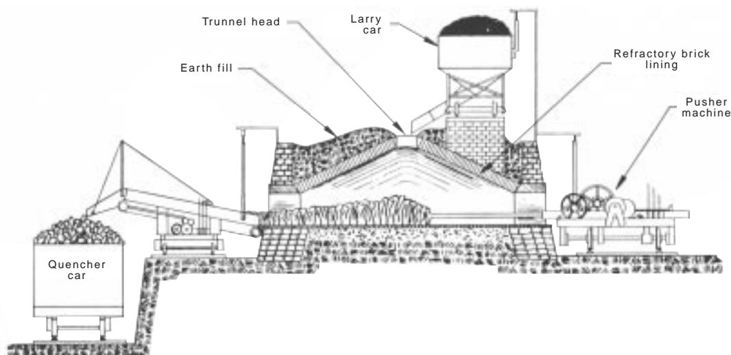
**Fig. 7.21** Ideal section of a beehive coke oven in a single block battery, showing refractory lining, earth fill, larry car, pusher, quencher car and other details, including the trunnel head at the top through which the coal was charged and the volatile products escaped. Vertical lines in the coke bed indicate the fissures that developed during coking, giving beehive coke its characteristic columnar structure.
