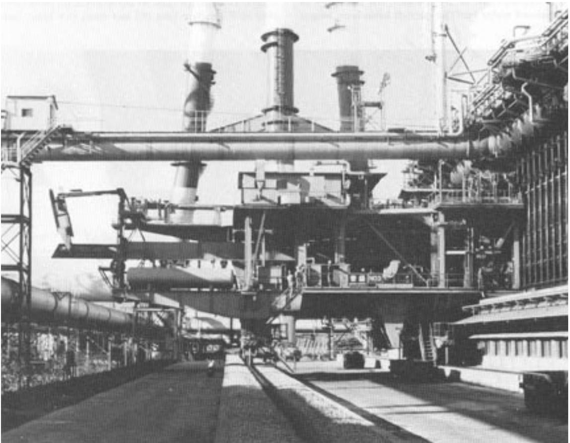
**Fig. 7.40** Pusher side equipment of a battery of byproduct coke ovens, showing the machine which is equipped to level the coal charge in the oven and also push the finished coke out of the oven, as well as remove and replace oven doors before and after the pushing operation.
