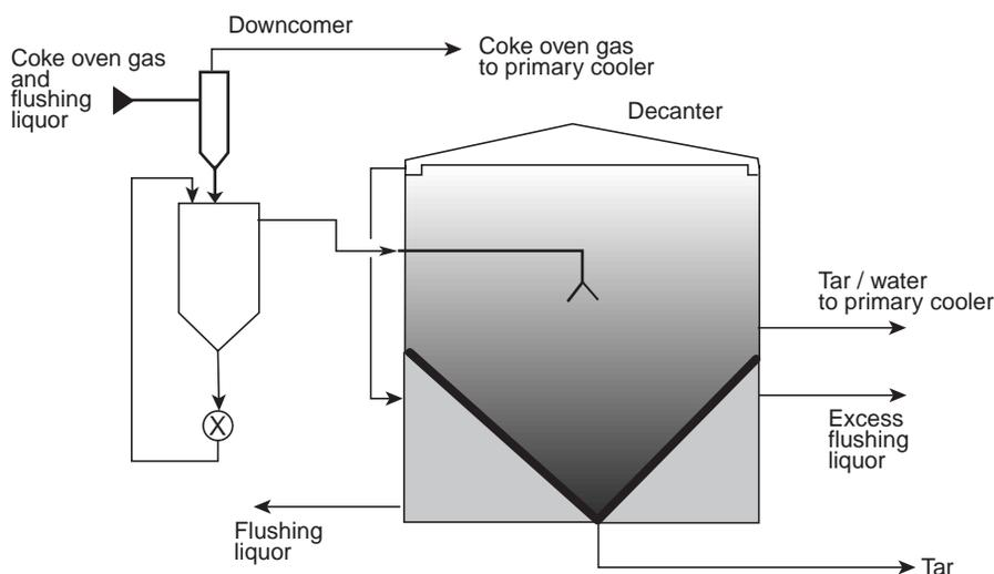
Fig. 7.93 Flushing liquor handling system without a heavy tar box.
