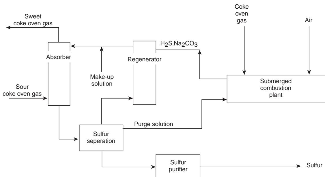
**Fig. 7.112** Flow diagram of the Takahax process for desulfurization of coke oven gas.
