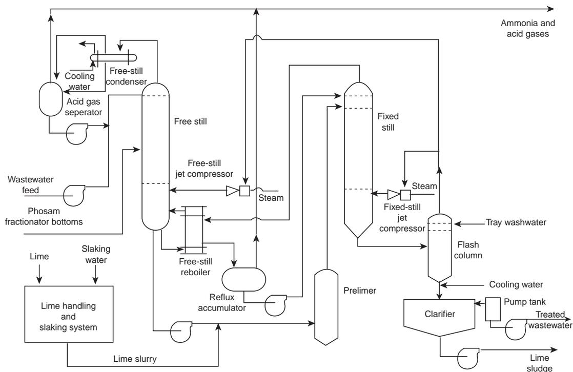
Fig. 7.101 Flow diagram of the USS CYAM system.
