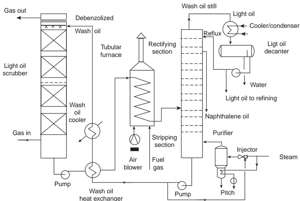
Fig. 7.107 Typical flowsheet of a light oil recovery system with coal tar wash oil.
