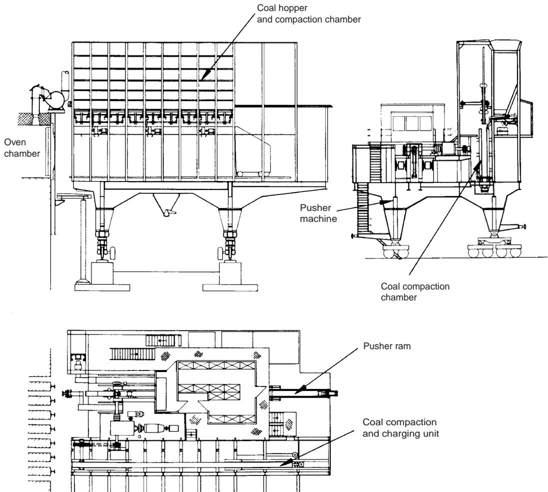
Fig. 7.54 Top, side and end elevations of a coke oven pushing machine incorporating a stamp charging unit.
