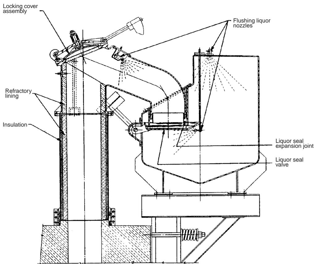
Fig. 7.36 Wilputte arrangement of standpipe, liquid-sealed damper valve, collecting main and automatic elbow cleaner.
