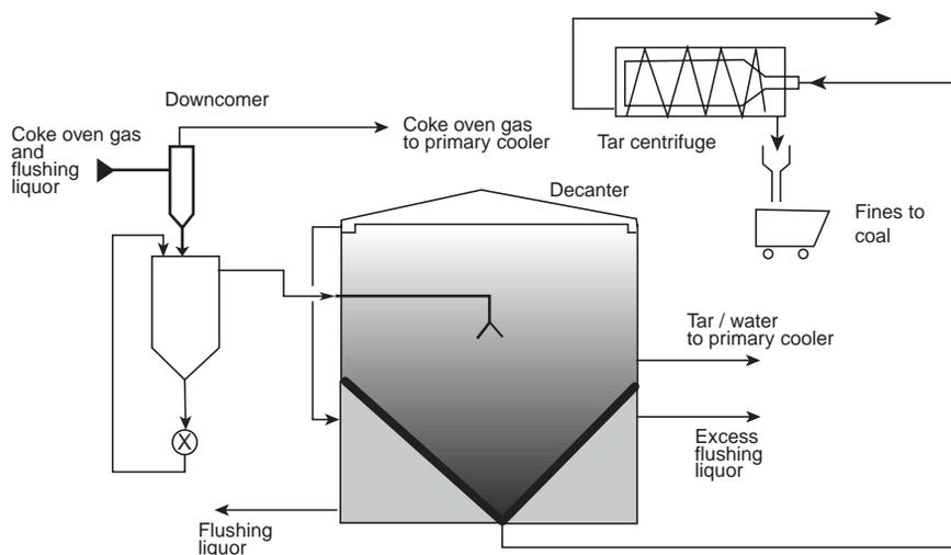
Fig. 7.94 Flushing liquor handling system with a centrifuge to reduce fines content.
