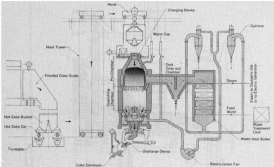
Fig. 7.45 Flow diagram of a dry-quenching system
