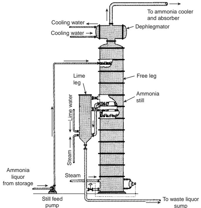
Fig. 7.100 Diagrammatic representation of the essential parts and operation of an ammonia still.
