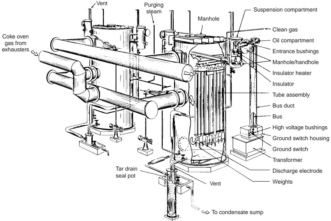
Fig. 7.99 Electrostatic precipitators of the tube type.
