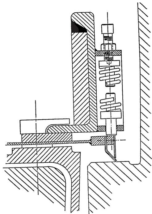
Fig. 7.33 Saturn door cross-section through retrofit seal.
