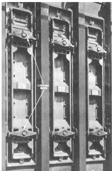
**Fig. 7.29** Wilputte design of self-sealing coke oven doors, showing spring loaded bars that maintain metal-to-metal contact between the door and jamb.
