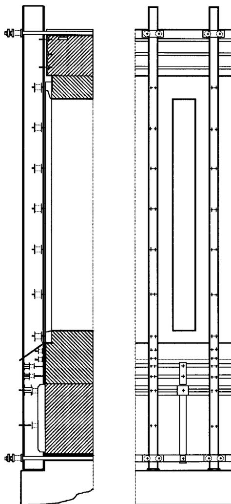
Fig. 7.83 Bracing system for a twin flue underjet oven system.
