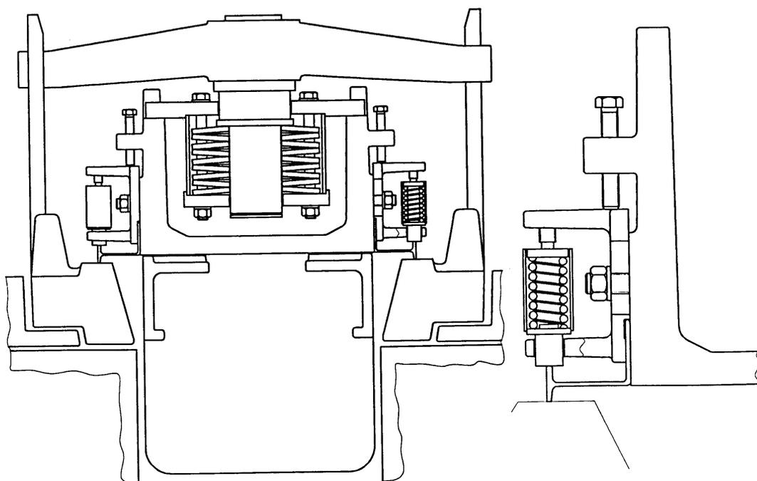
**Fig. 7.30** Thyssen Still Otto self-sealing coke oven door with spring loaded sealing strips.
