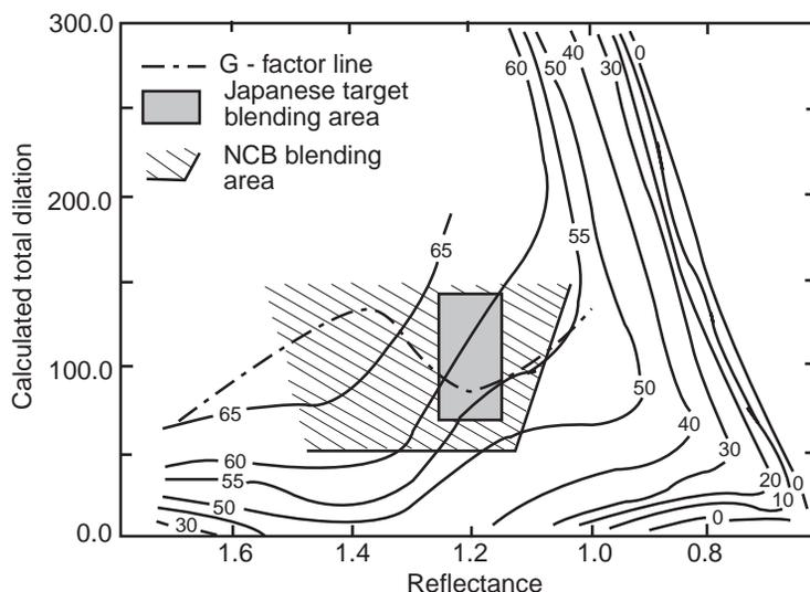
Fig. 7.8 Stability prediction using total dilatation and rank. (From Ref. 14)
