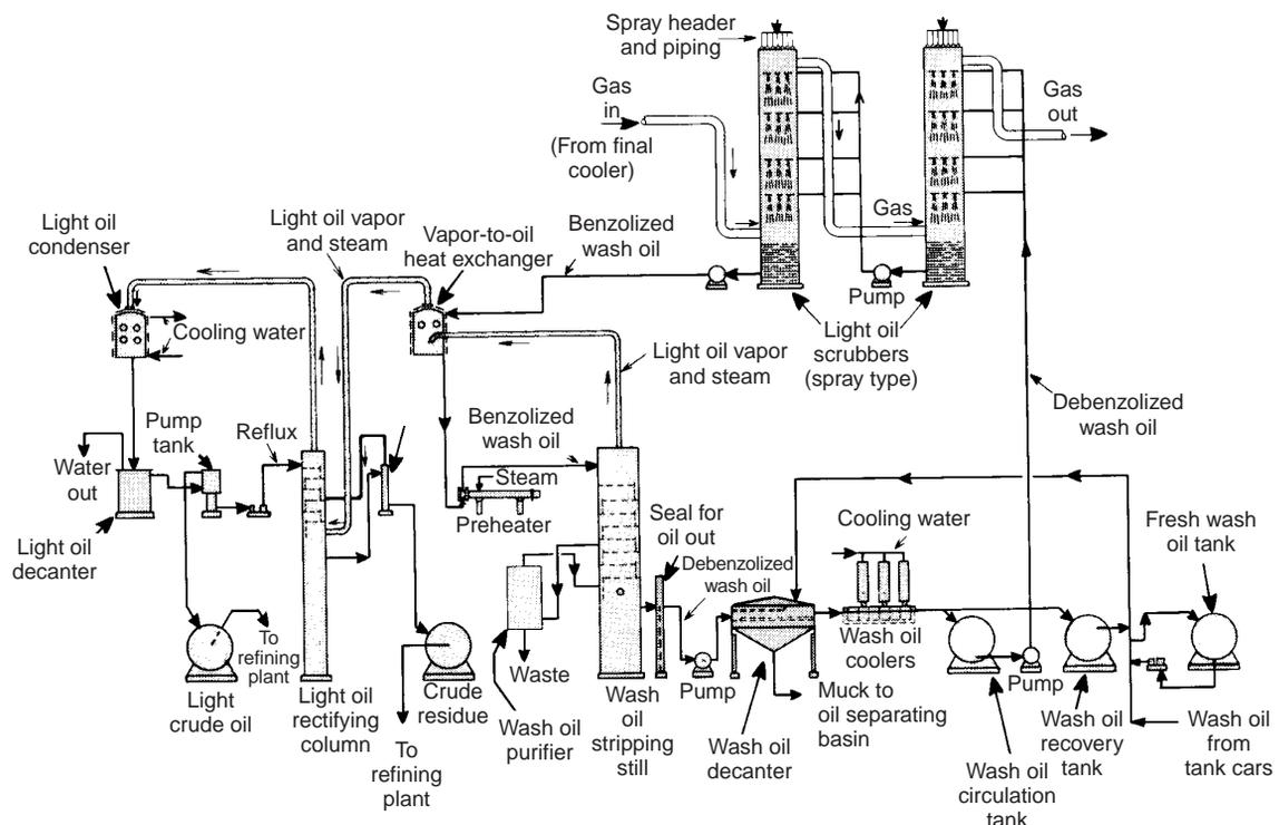
Fig. 7.106 Flowsheet of a light oil recovery system.
