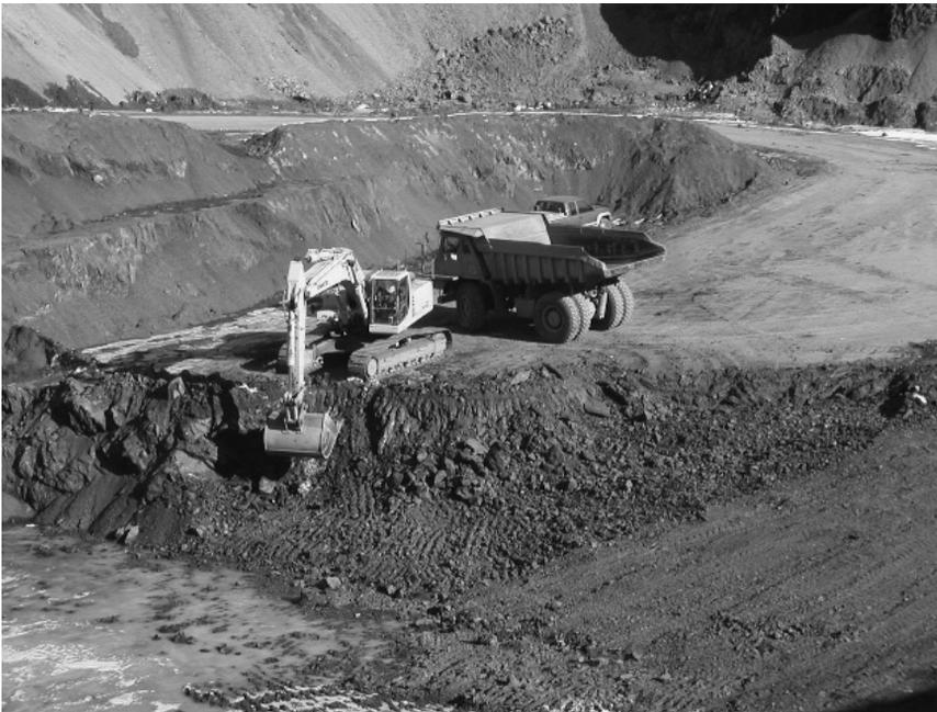
**Figure 10.11** Mining of shale feedstock for high-temperature rotary kiln lightweight aggregate. (Courtesy of Utelite Corporation, Coalville, UT.)
