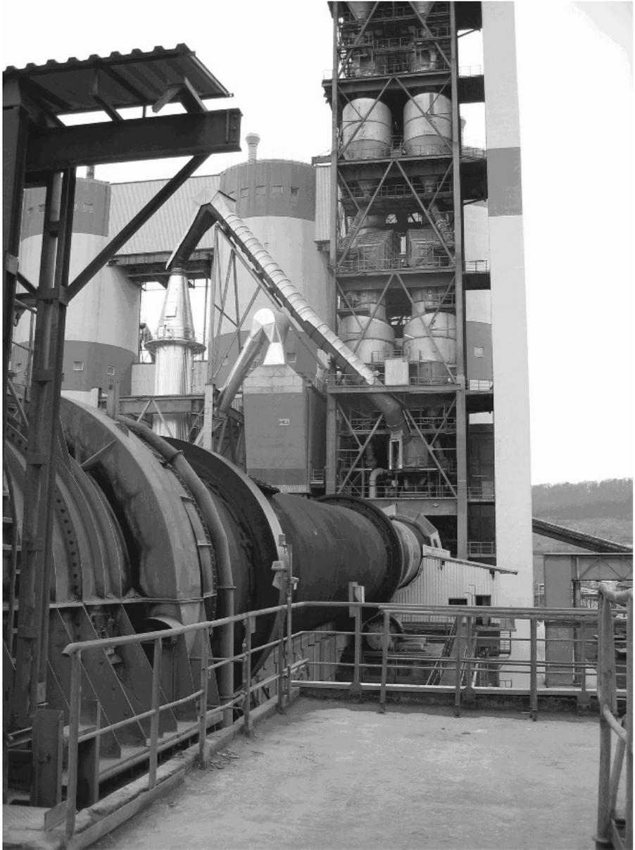
**Figure 1.7** Cement kiln equipped with cyclone preheaters.
