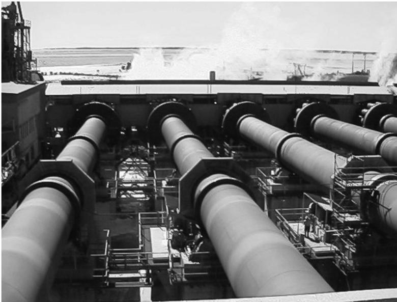
**Figure 1.6** Wet, long cement kiln. (Courtesy of FLS Minerals.)
