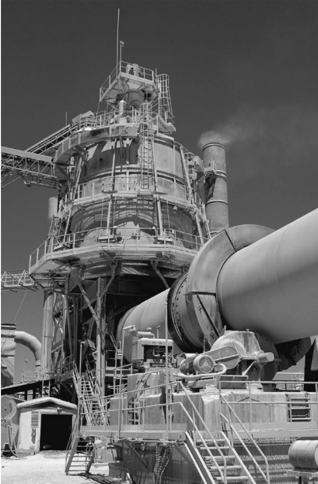
**Figure 10.4** Photo of preheater lime kiln. (Courtesy of Graymont, Inc., Cricket Mountain Plant.)
