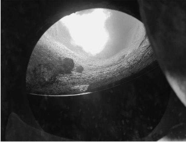
**Figure 10.15** Combustion zone region of an LWA kiln with material at incipient fusion. (Courtesy of Utelite Corporation, Coalville, UT.)
