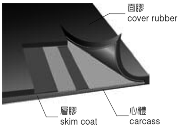
Fig. 1.6 Cross section of canvas conveyor
