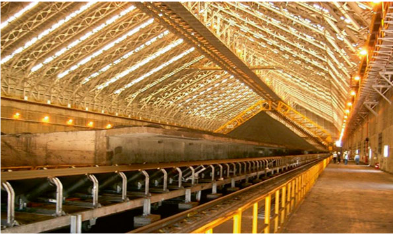
Fig. 1.13 Strip type indoor yard-interior
