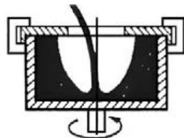
**-025 semi-centrifugal casting**
