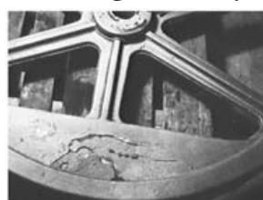
**-024 flow marks, flow figures, flow lines****رَد بار**
