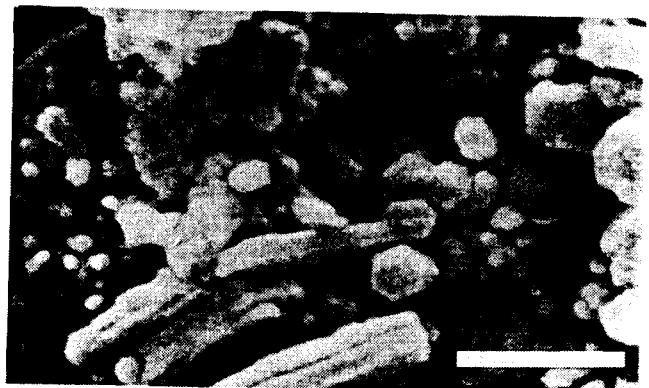
Fig. 7. Scanning electron micrograph of CAH 10 crystals (bar = 2 μm).
