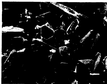
Fig. 7. Scanning electron micrograph of corundum crystals ( \times 1000 ).
