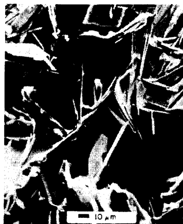
Fig. 8. Scanning electron micrograph of fracture surface of a machineable fluorophlogopite glass-ceramic. "House of cards" structure is the key to machineability.
