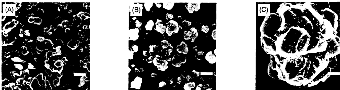
Fig. 3. Scanning electron micrographs of aluminum hydroxides for fillers (bars = (a) 0.5 μm; (b), (c) 10 μm).
