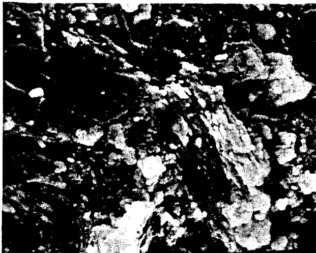
Fig. 6. Scanning electron micrograph of crystalline-type alumina ( \times 3000 ).
