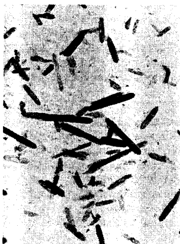
Fig. 6. Transmission electron micrograph of boehmite crystals ( \times 42\,000 ).
