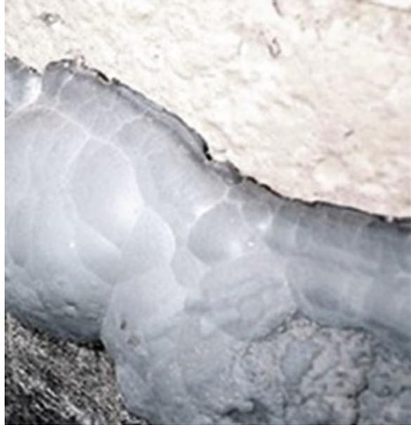
**Fig. 1.30** Cross section of the reduction cell with freezing line of electrolyte
