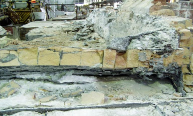
**Fig. 3.9** The failure of the holding furnace from bricks. Aluminium, which penetrated through the shafts between the bricks, can be clearly seen
