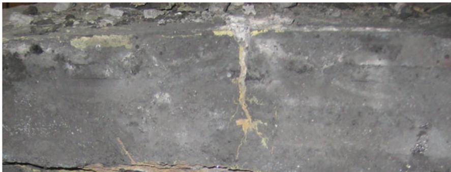
Fig. 2.47 Aluminium carbide in the crack in carbon cathode block
