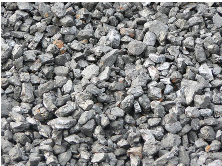
**Fig. 2.23** Raw anthracite grains with contaminations
