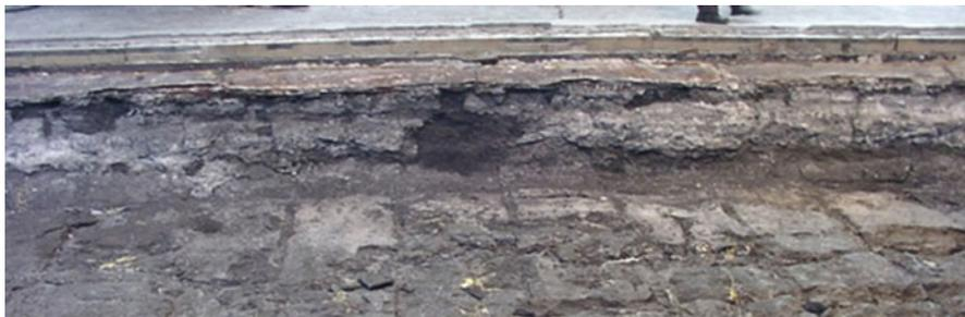
**Fig. 1.28** Carbon side lining in “out-of-service” reduction cell
