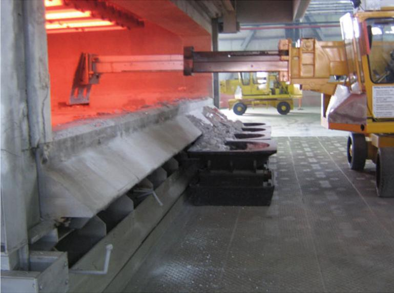
**Fig. 3.18** Holding furnace
