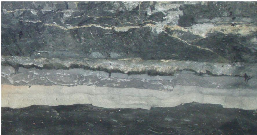
**Fig. 2.87** Picture of dry autopsy: due to pressure and the formation of the lens, the height of the heat insulation layer decreased
