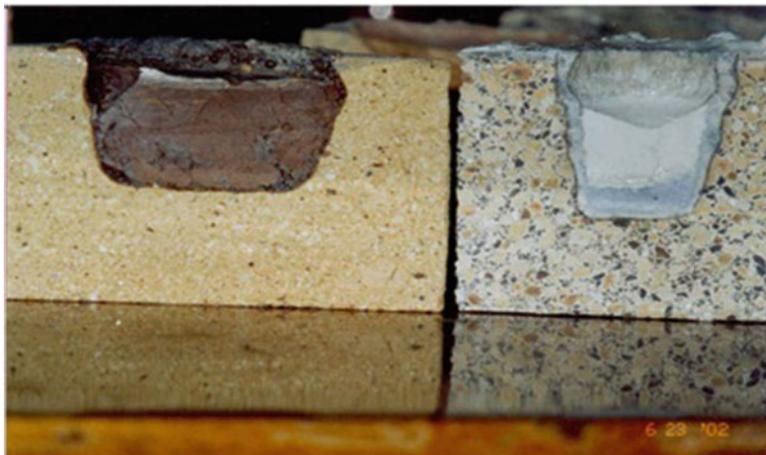
**Fig. 2.79** The results of cup test for cryolite resistance of fireclay brick and low-cement castable (concrete)
