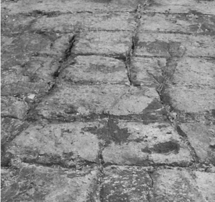
**Fig. 1.12** Cathode bottom of reduction cell before the dry autopsy
