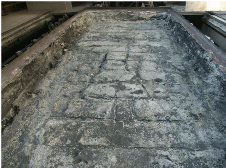
**Fig. 2.80** The cell with bottom heaving before dry autopsy
