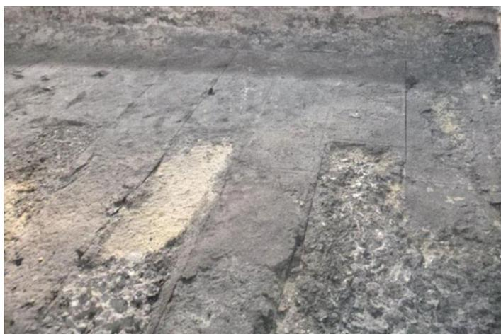
Fig. 2.16 Exfoliated carbon cathode blocks after startup
