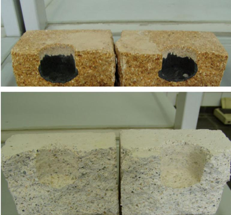
**Fig. 3.8** Cup corrosion test of fireclay brick and LCC. The LCC refractory is unchanged
