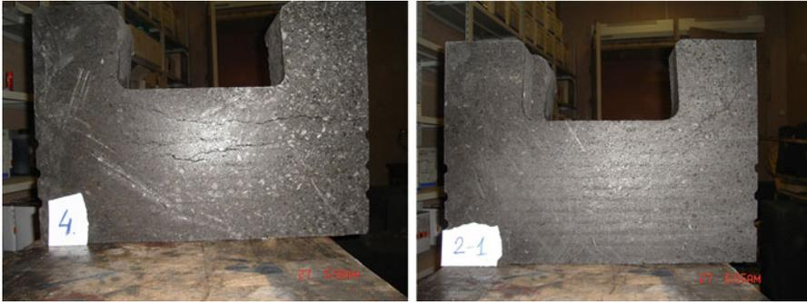
**Fig. 2.32** Examples of the internal cracks inside the carbon cathode blocks that are not seen on the surface but are seen on cross section after cutting
