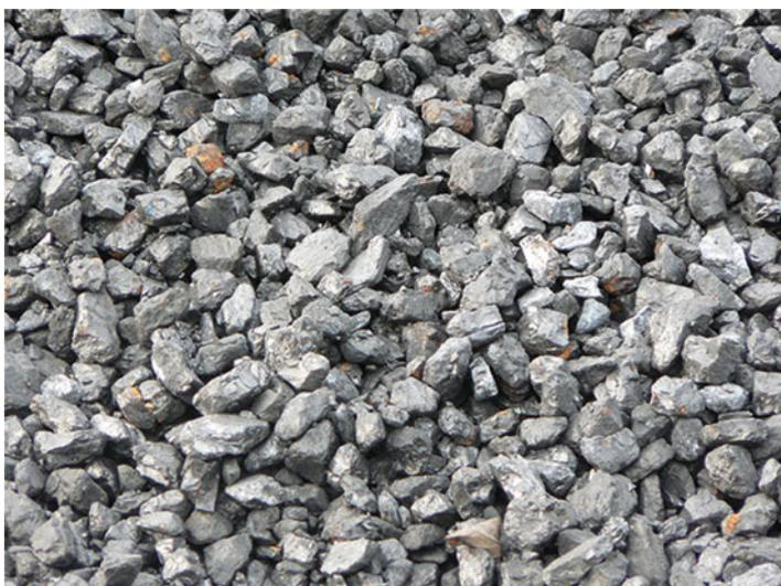
**Fig. 2.23** Raw anthracite grains with contaminations
