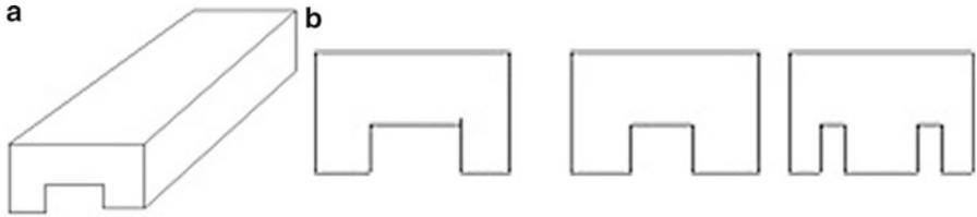
Fig. 2.17 (a) Carbon cathode bottom block; (b) shapes of the slots
