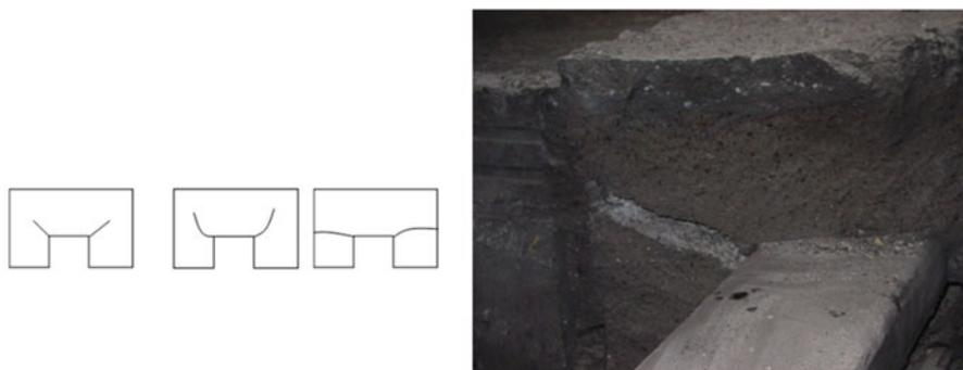
**Fig. 2.42** Cracking of the carbon cathode block in the angles of the slot
