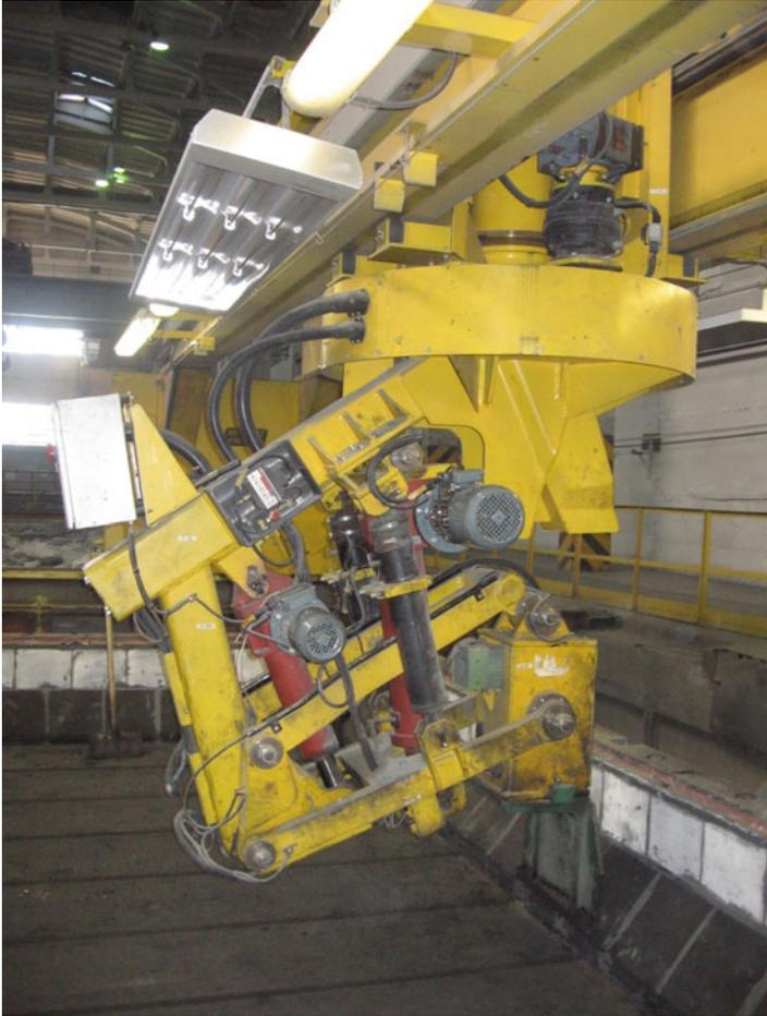
**Fig. 2.57** Machined ramming of peripheral seam
