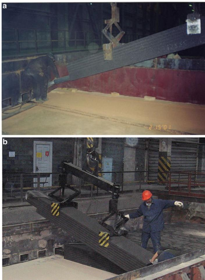
**Fig. 2.8** Installation of carbon cathode block with sealed steel collector bar in the shell
