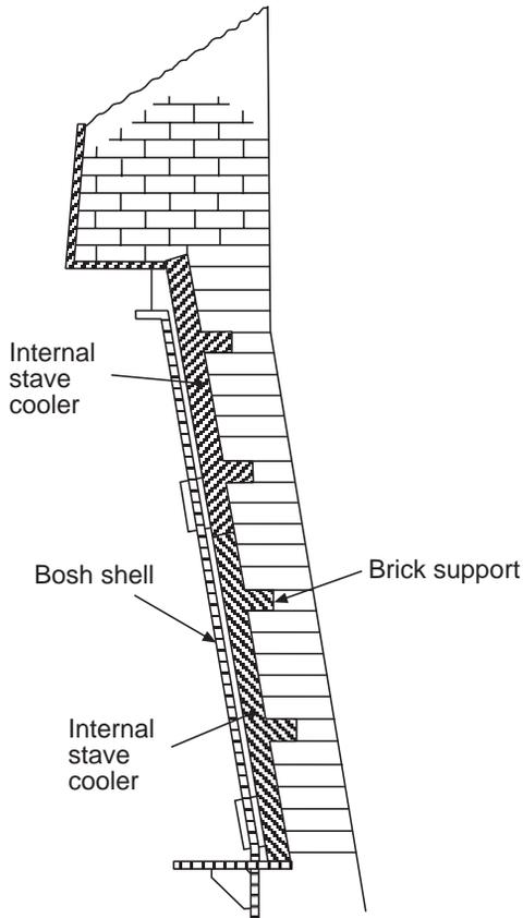
Fig. 9.11 Cast iron staves with brick supports.
