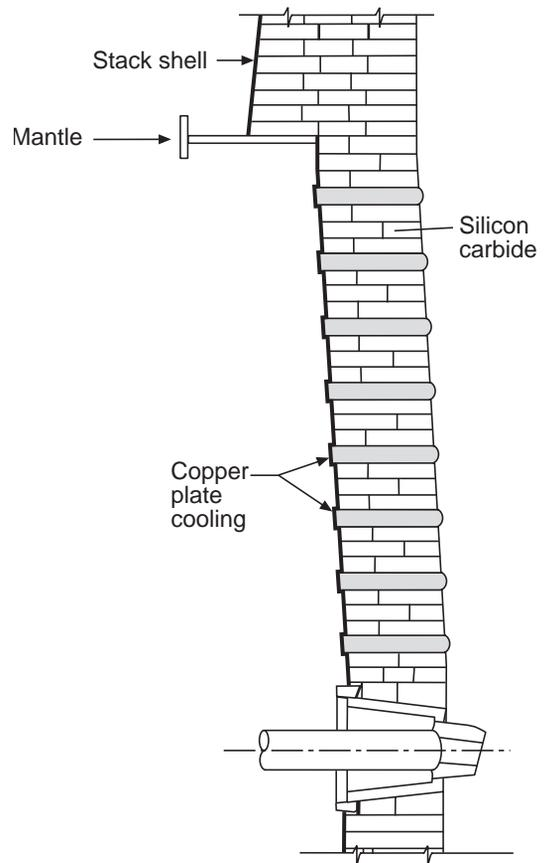
Fig. 9.10 Bosh cooling by radially spaced copper elements.
