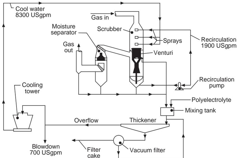
Fig. 9.33 Schematic of a modern closed-circuit water system for gas cleaning.
