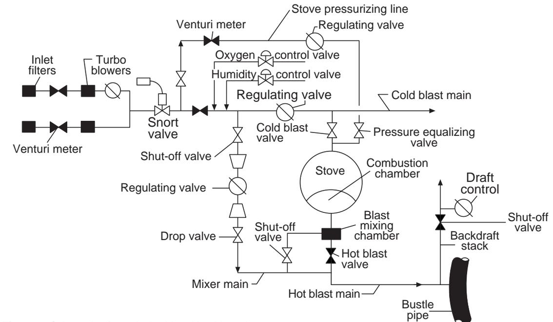
**Fig. 9.40** Schematic of a typical cold and hot blast air system.
