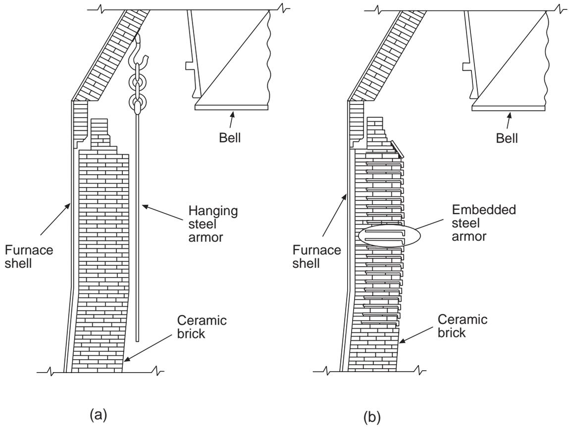
Fig. 9.15 Schematic of stockline armor: (a) hanging armor, (b) fixed armor.
