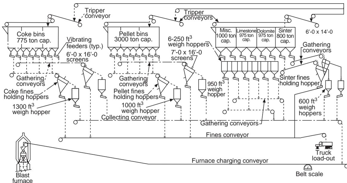
Fig. 9.19 Automated stockhouse for a conveyor belt-fed blast furnace.
