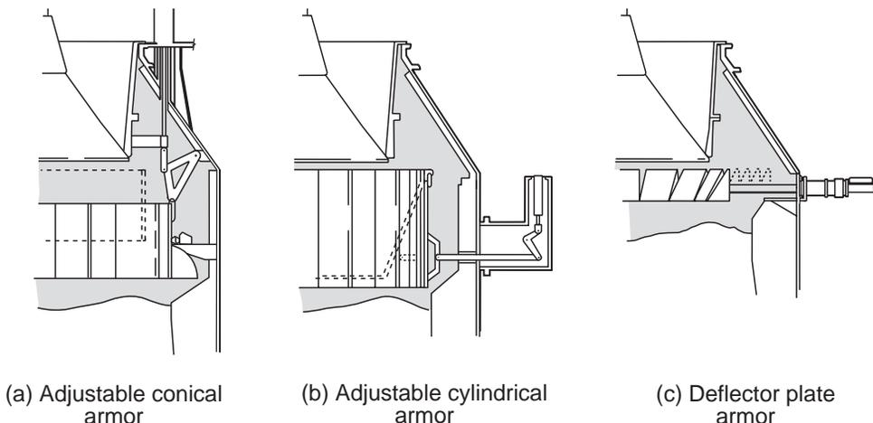
Fig. 9.25 Types of adjustable throat armor used to control burden distribution.
