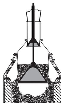
Small bell closed to prevent escape of gas to atmosphere and large bell open to admit charge to the furnace.
