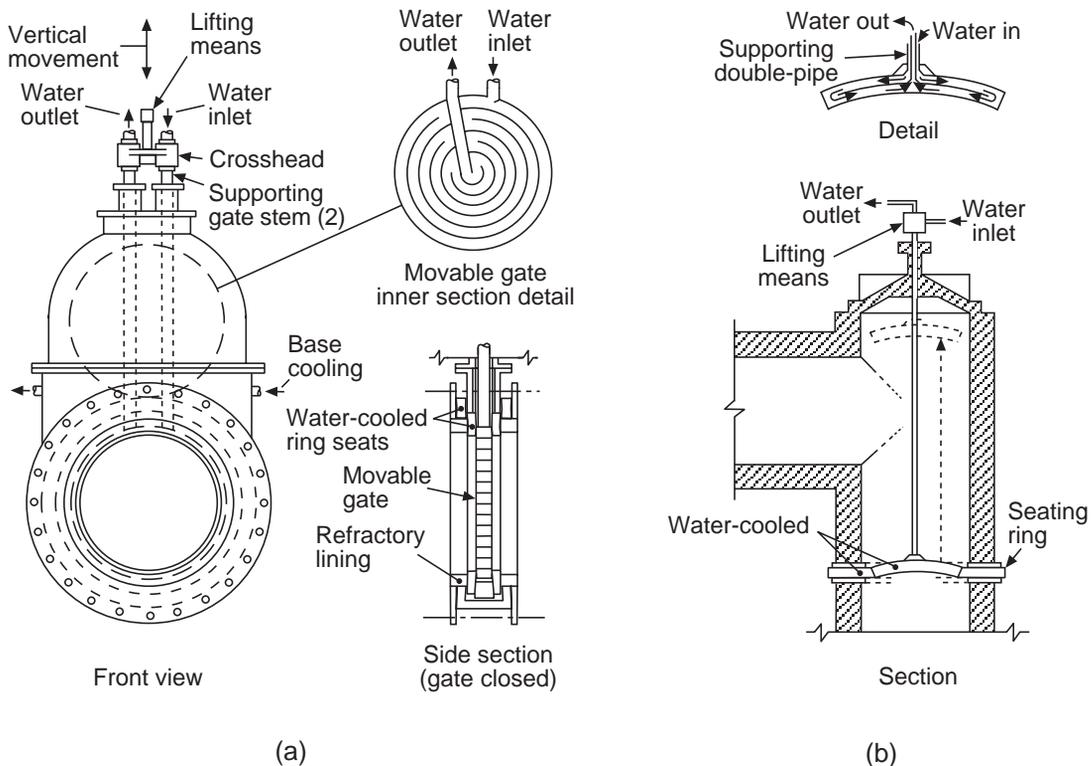
Fig. 9.37 Hot blast valves.
