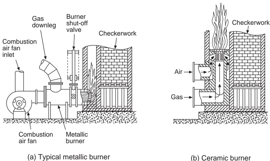
Fig. 9.36 Schematic of hot blast stove burners.
