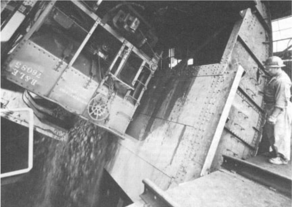
Fig. 9.43 Rotary car dumper with the railroad car in the inverted position.
