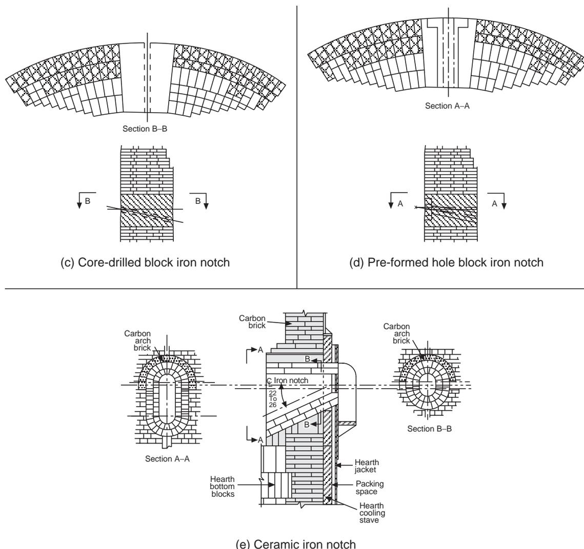
Fig. 9.4 Typical iron notch configurations
