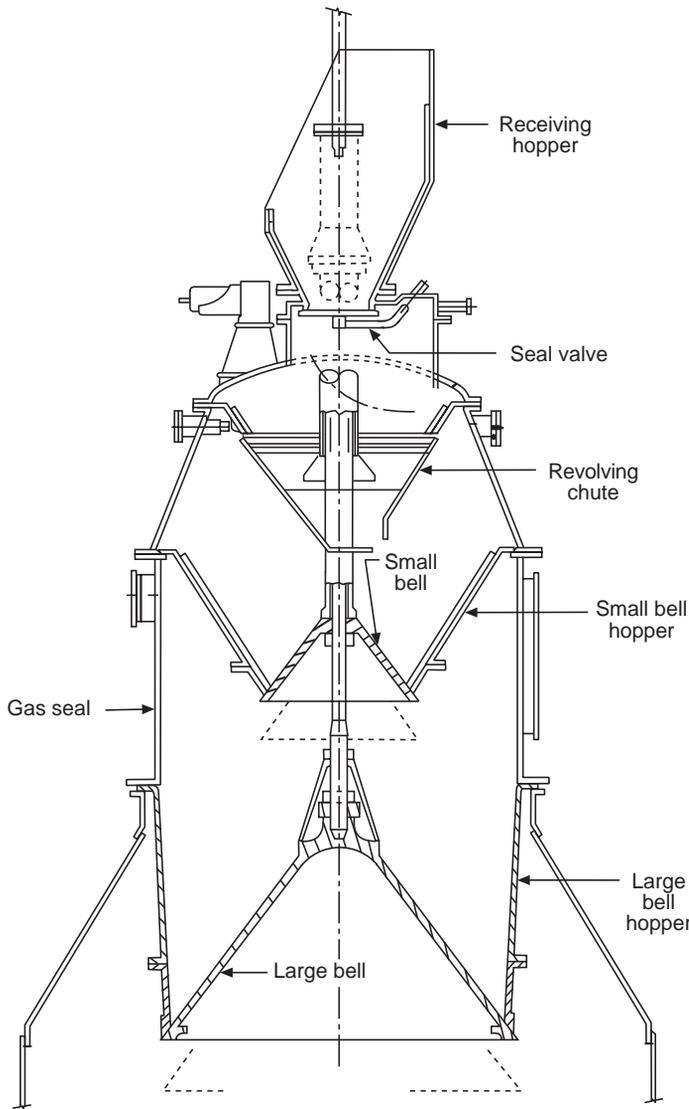
Fig. 9.24 Schematic of two-bell top with seal valves and a revolving chute.
