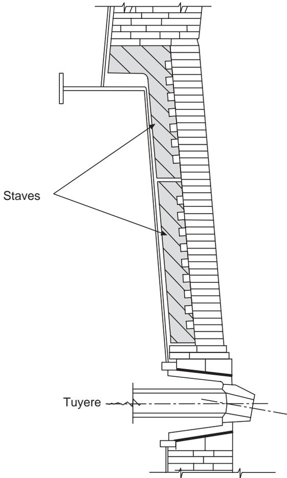
Fig. 9.9 Cast iron stave cooling.
