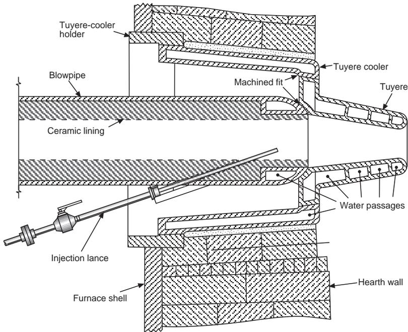
Fig. 9.6 Tuyere and blowpipe assembly.
