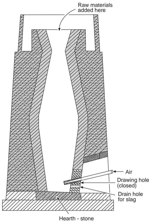
Fig. 9.20 Schematic cross-section of a Stuckofen with an open top.
