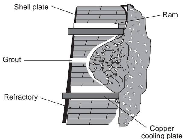
Fig. 9.13 Typical example of a grout repair.
