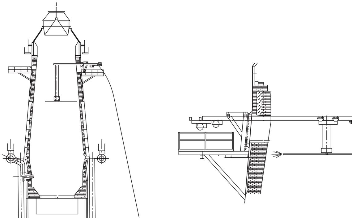
Fig. 9.14 Platform and gantry installation for gunning the blast furnace
