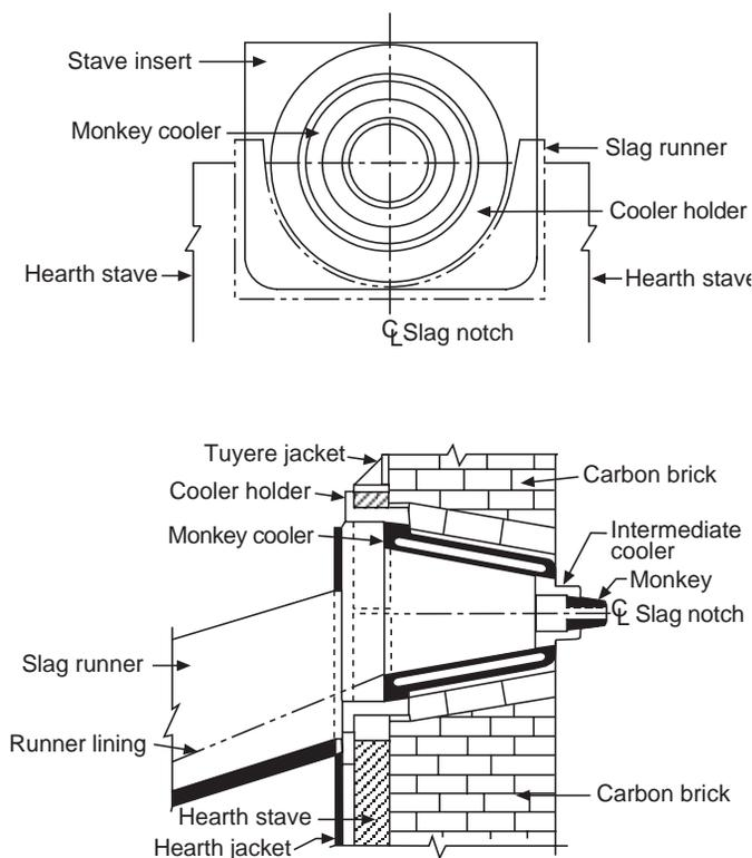
Fig. 9.5 Section and developed view of a cinder (slag) notch.
