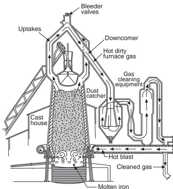
Fig. 9.29 General arrangement of blast furnace gas equipment.
