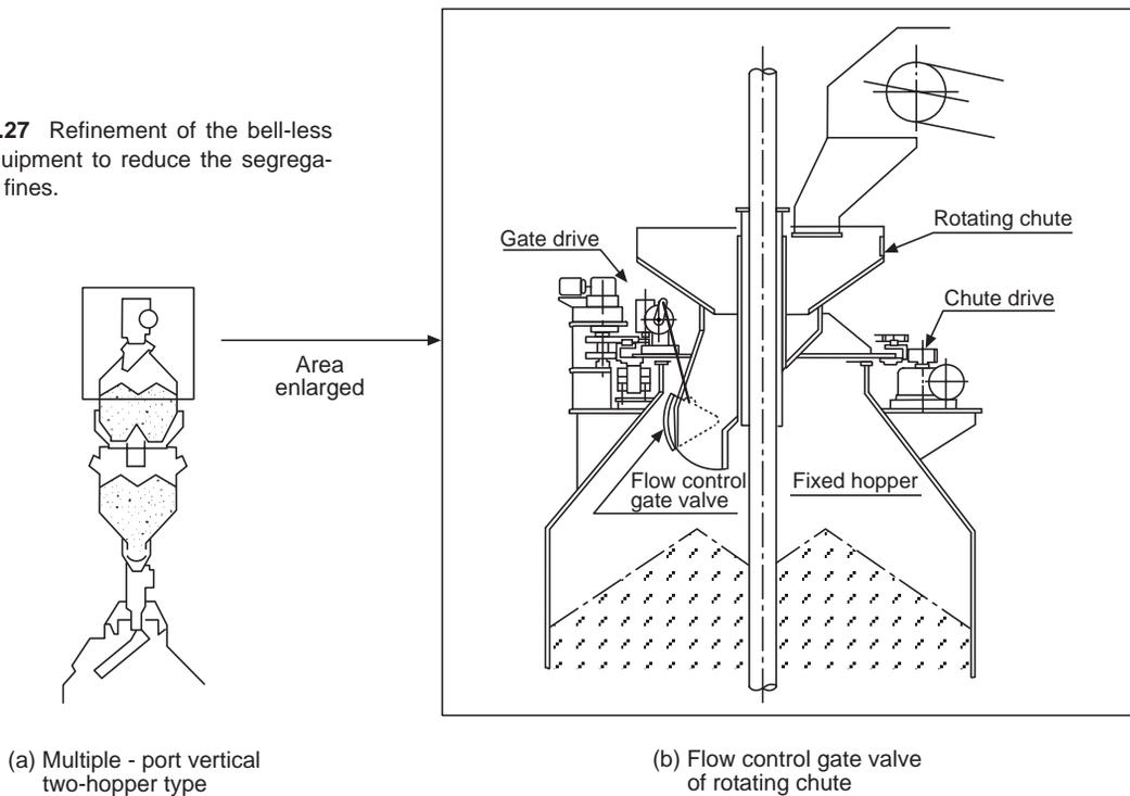
a rotating chute into a large receiving hopper that is positioned above the single large lockhopper yields the desired result of dispersing the finer material evenly throughout the burden, Fig. 9.27.
