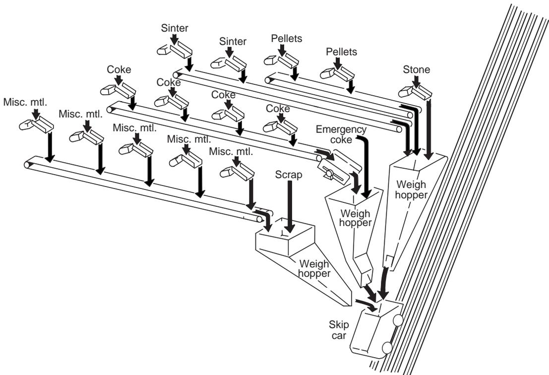
Fig. 9.18 Simplified schematic of an automated stockhouse for a skip-fed furnace.
