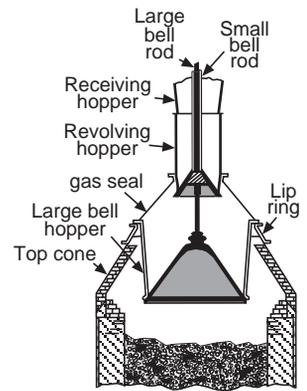
Both bells closed, ready to repeat charging cycle. Note that rod supporting large bell passes through hollow rod supporting small bell, permitting independent operation of bells.
