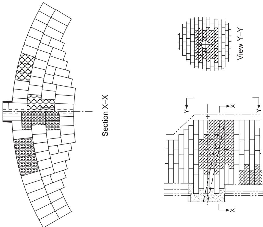
(a) Core-drilled brick iron notch
