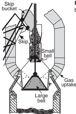
Small bell and large bell both closed, skip bucket tipped to dump charge in hopper above small bell. Gas flowing from top of furnace through uptakes located in dome (top cone).
