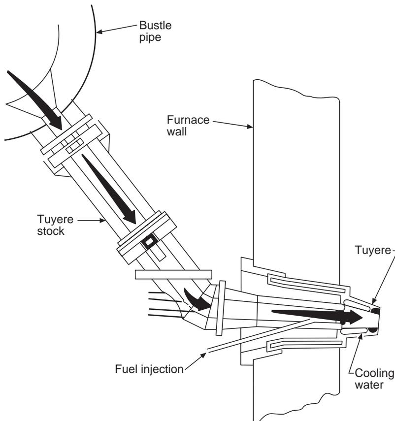
Fig. 9.41 Schematic of a typical tuyere stock arrangement.
