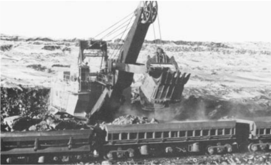
Fig. 8.16 Electric power shovel loading material from an open pit iron ore mine for transfer to an ore processing plant.
