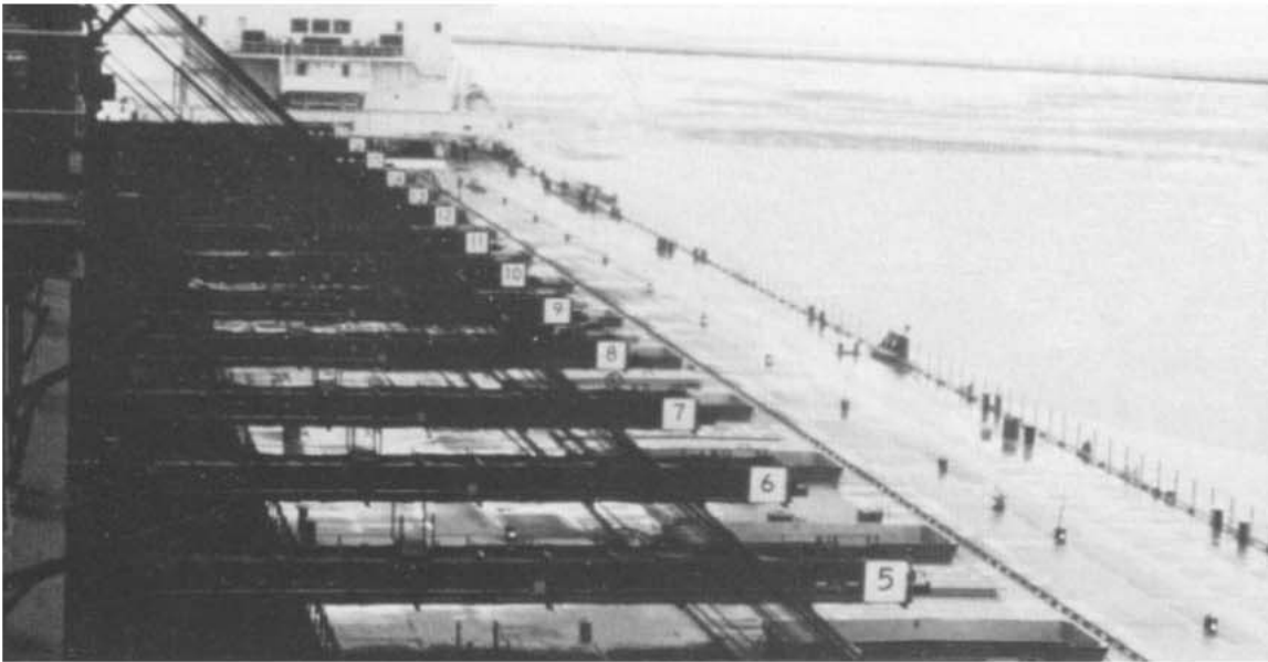
Fig. 8.39 Great Lakes vessel Edwin H. Gott , 305 m (1000 ft) in length, being loaded with pellets at a modern conveyor loading dock.
