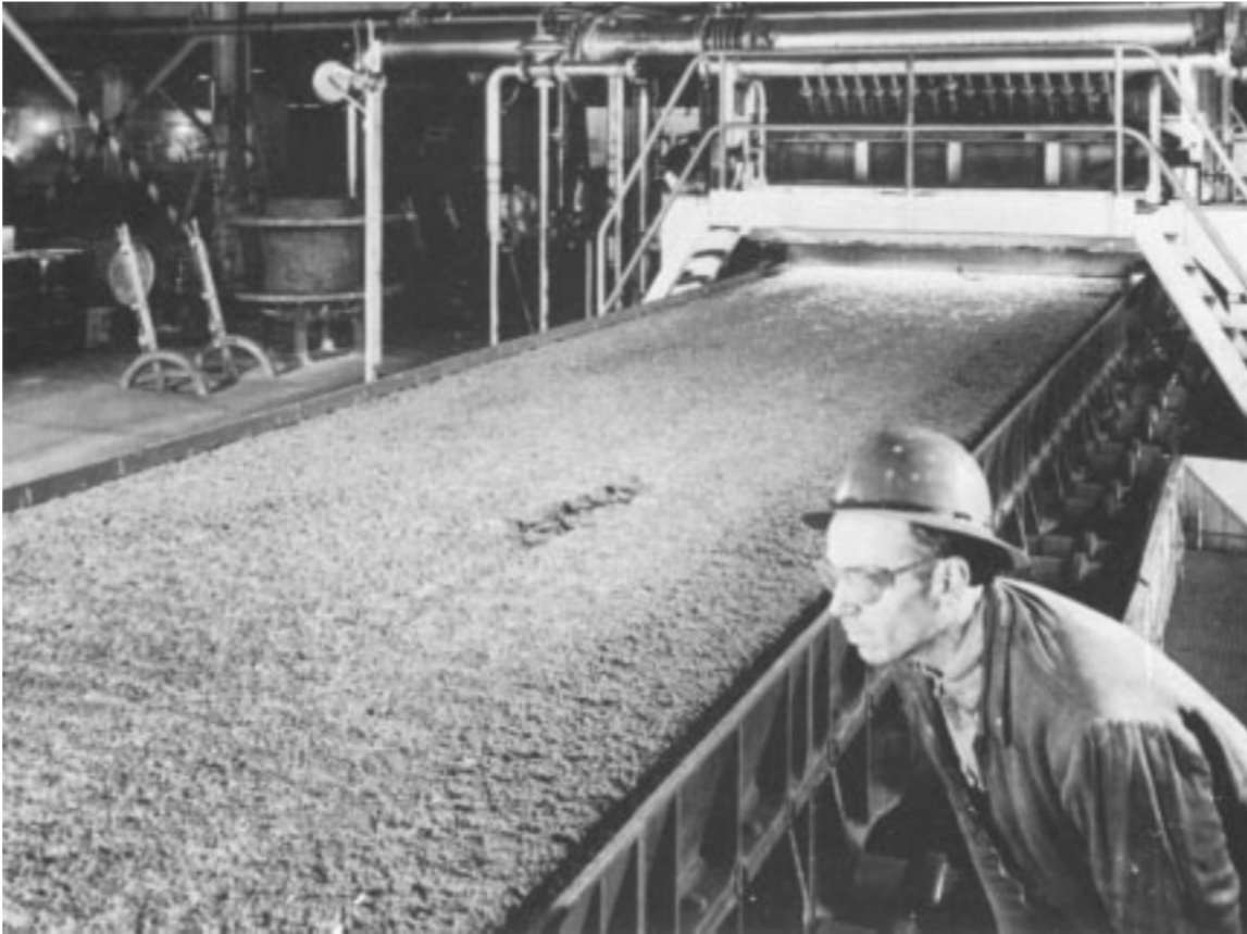
Fig. 8.31 Sintering machine in operation. The ignition furnace in the center background ignites the fuel in the surface layer of the sinter mix. As the bed of sinter progresses into the foreground, air is pulled down through the bed to cause the burning zone to move downward through the bed by igniting fuel in deeper and deeper zones of the mix. By the time the discharge end of the machine is reached, sintering will have taken place throughout the depth of the bed.
