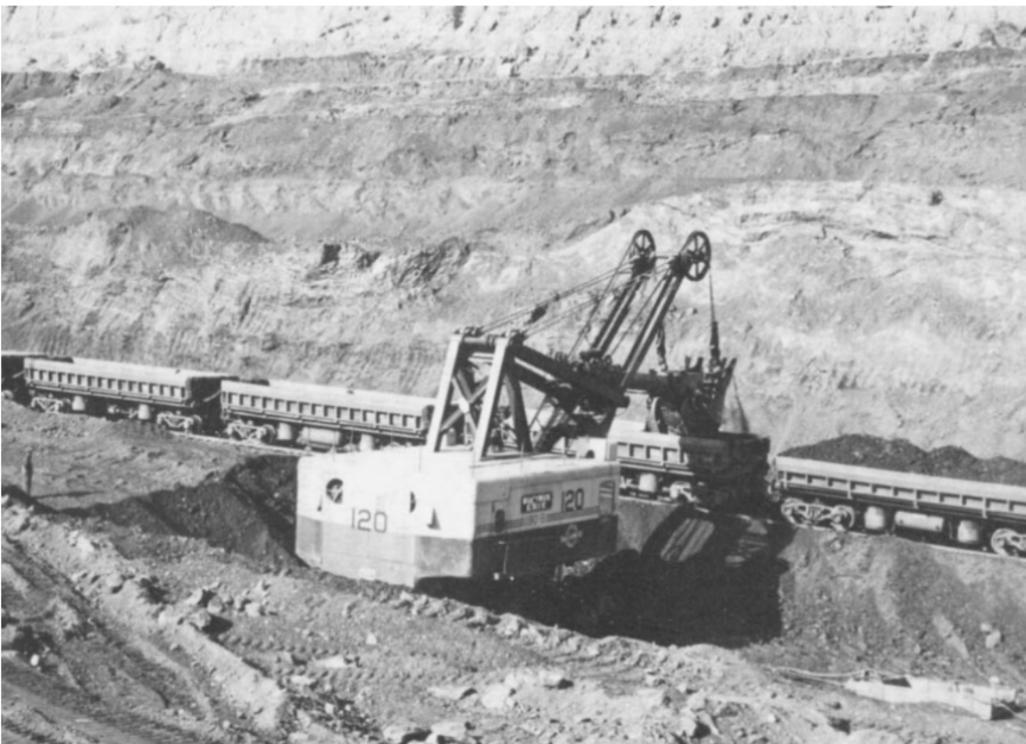
Fig. 8.17 Electric power shovel on caterpillar tracks, making a sinking cut and loading ore into steel dump cars for haulage from an open pit mine to a beneficiation plant. Diesel-electric locomotives handle the dump cars while a cable carries power to the shovel.
