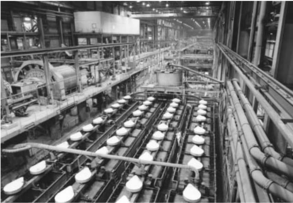
Fig. 8.25 Flotation section in foreground, grinding mills and magnetic separation in the background at U.S. Steel Minntac
