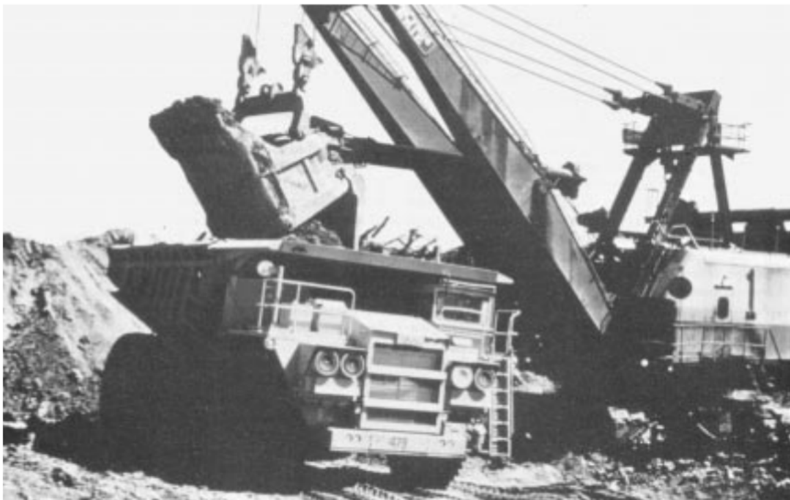
Fig. 8.15 Electric power shovel in an open pit mine loading iron bearing material into a diesel powered truck for transfer to a processing plant.
