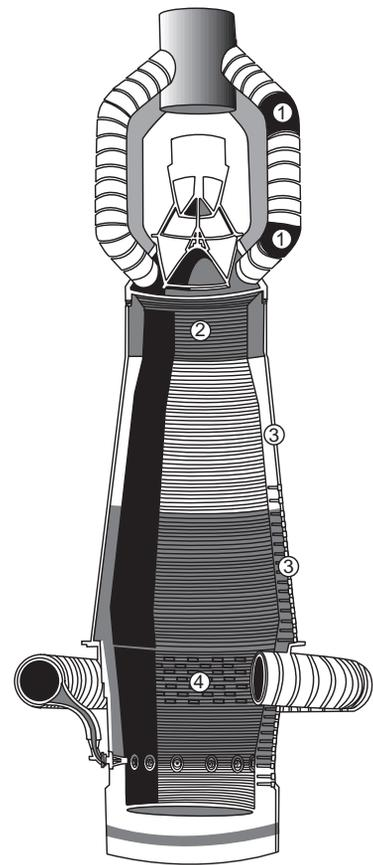
Fig. 4.2 Use of gunning mixes for blast furnace repair. Refer to Table 4.9.
