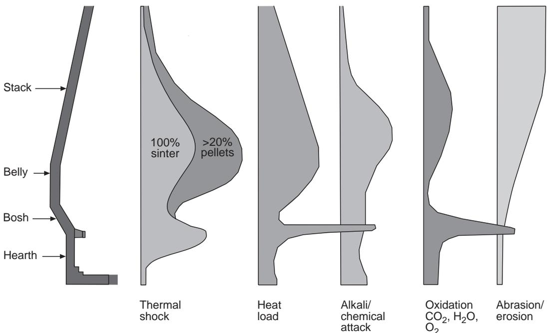
Fig. 4.1 Blast furnace refractory wear mechanisms and their severity by zone.
