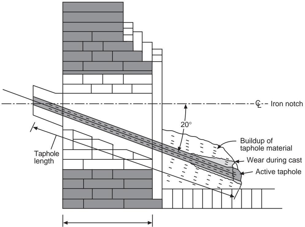
Fig. 4.3 Taphole construction and buildup inside furnace.
