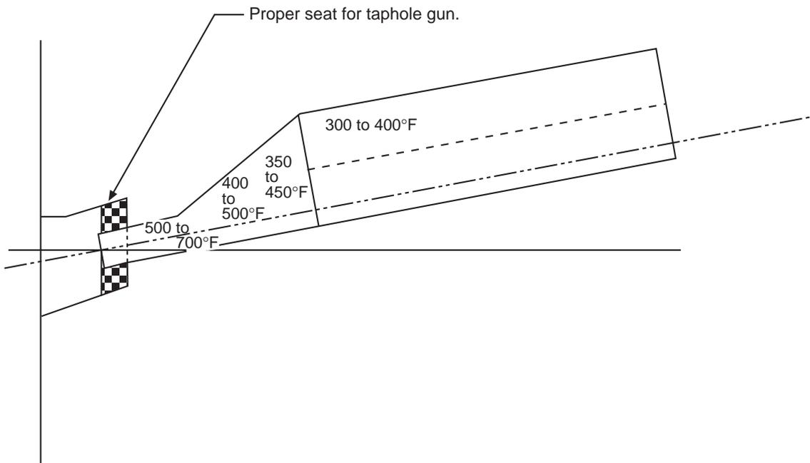
Fig. 4.4 Ideal position of taphole gun in iron notch for closing off a cast.
