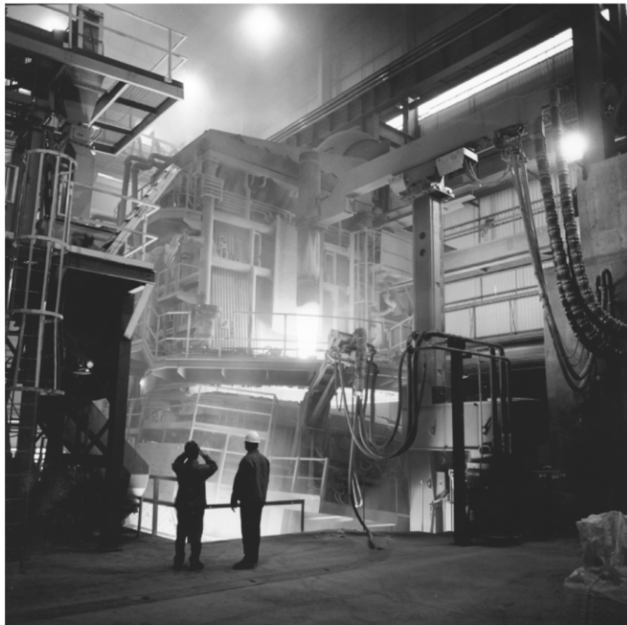
Fig. 10.84 Shaft furnace in operation at North Star Steel, Kingman, Arizona.
