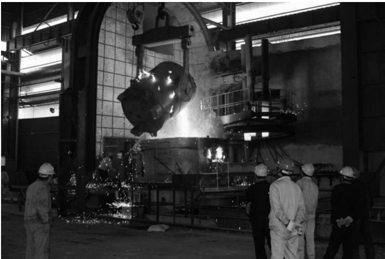
FIGURE 1.13 Ladle (steel industry).
