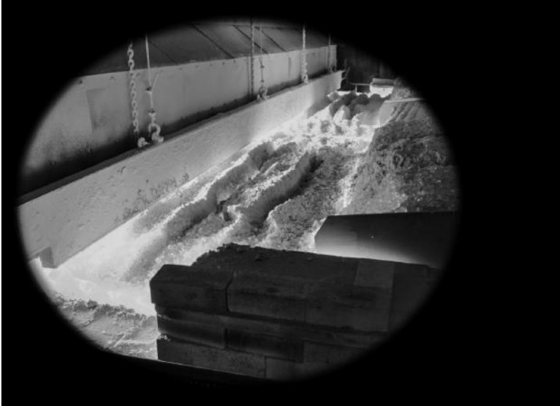
FIGURE 1.18 Glass tank (glass industry).
