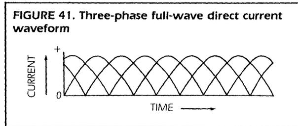
Three-phase full-wave direct current has all of the advantages of single-phase full-wave direct current plus some additional benefits. The current draw on the power line is spread over three phases, reducing the demand by nearly half. The demand on the line is also balanced, with each leg providing a portion of the current (single-phase pulls all of
