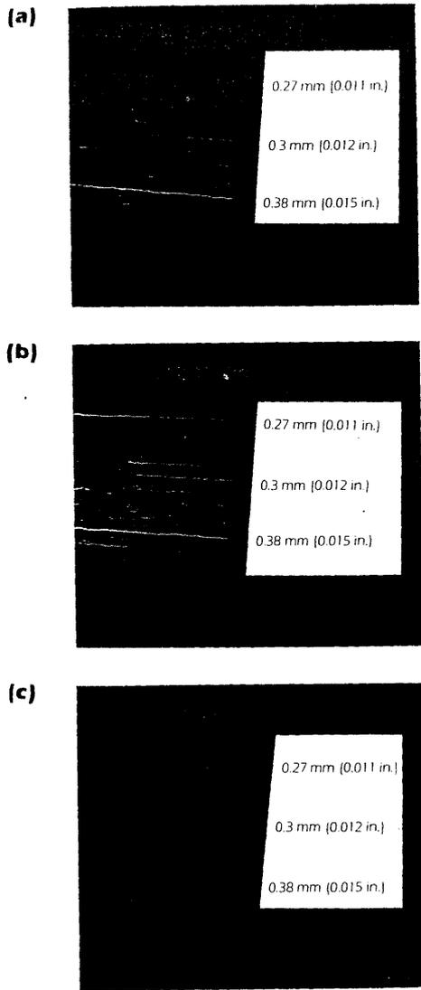
FIGURE 17. Ultraviolet photographs taken at the ends square steel billets for comparison of magnetic particle indication brightness versus crack depth: (a) continuous direct current at 200 A; (b) continuous direct current at 800 A; and (c) residual direct current at 200 A
