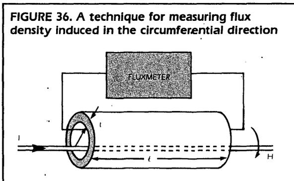
**FIGURE 36. A technique for measuring flux density induced in the circumferential direction**
