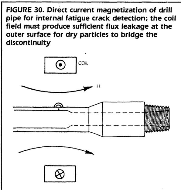
inspected with a borescope. The presence of one fatigue crack is sufficient for rejecting the tube. The field strength used for the test in Fig. 30 is around 40 mT (400 G). The coil is passed back and forth over the suspect region to obtain a crack indication in the presence of furring. When a borescope is used, appropriate crack indications can generally be produced with longitudinal residual induction techniques.
