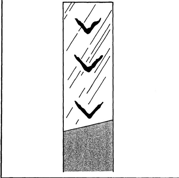
Cooling cracks are generally longitudinal but because they tend to curve around the object shape, they are not necessarily straight. Such cracks may be long and often vary in depth along their length. Magnetic particle indications of cooling cracks therefore can vary in intensity (heavier where the crack is deepest).
