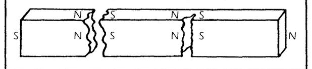
If the center piece in Fig. 14 is reversed so that similar poles are adjacent, the lines of force repel one magnet from the other. If one of the bars is small enough, the lines of force can cause it to rotate so that unlike poles are again adjacent. This illustrates the most basic rule of magnetism: unlike poles attract and like poles repel.
