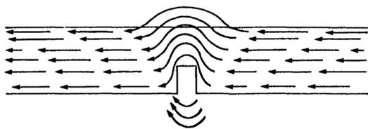
**FIGURE 19. Internal or midwall discontinuity in a magnetized test object; there may or may not be magnetic flux leakage, depending on the value of the flux in the object**
