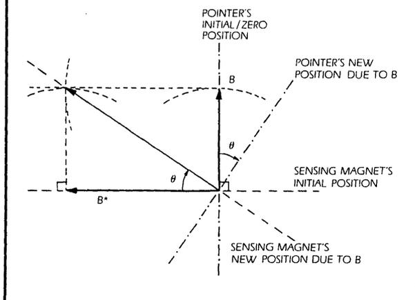
**FIGURE 24. Pointer deflection  $\alpha$  and  $\beta$  when  $B$  is not perpendicular to  $B^*$  ( $\alpha < \theta < \beta$ )**
