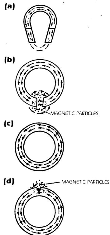
**FIGURE 17. Bar magnet illustrating longitudinal magnetization: (a) horseshoe magnet straightened into a bar magnet with north and south poles; (b) bar magnet containing a machined slot and corresponding flux leakage field; and (c) a crack in a longitudinally magnetized object produces poles that attract and hold magnetic particles**
