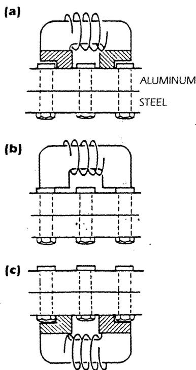
**FIGURE 8. Improved contact and improved magnetic field using pole pieces:** (a) poor contact (field partially lost); (b) improved field with the addition of pole pieces; and (c) magnetic field and contact are improved with correct pole piece configuration
