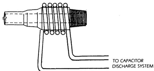
For magnetizing the end of a 200 mm (8 in.) outside diameter drill collar, the diameter of the coil is about 225 mm (9 in.). The number of ampere-turns is  $230 \times 225$  or  $5,800 \times 9$  or about 52,000. Should the capacitor discharge system produce a peak current of 9,000 A, then six turns are required. Alternatively, two or three pulses should be fired and the resulting residual induction checked with a field indicator.
