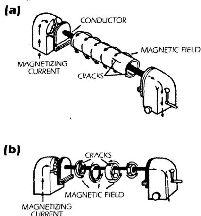
with negligible flux on the inside surface. The inside surface is often equally important when testing for discontinuities. Since a magnetic field surrounds a conductor, it is possible to induce a satisfactory field in the tube by inserting a copper bar or some other conductor through the component and passing the current through the bar.
