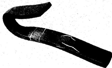
**FIGURE 3.** Experimental magnetic particle testing equipment used by F.B. Doane in 1930
