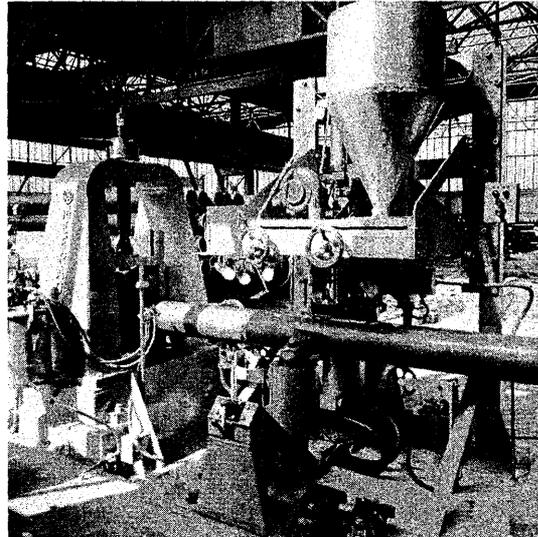
**FIGURE 33.** Noncontact magnetic particle system using the induced current method for testing of bearing races
