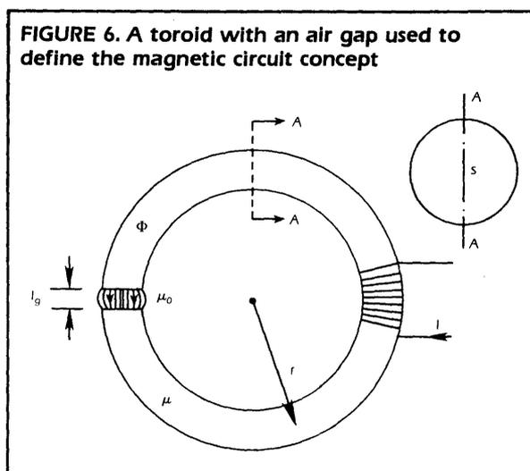
FIGURE 6. A toroid with an air gap used to define the magnetic circuit concept
