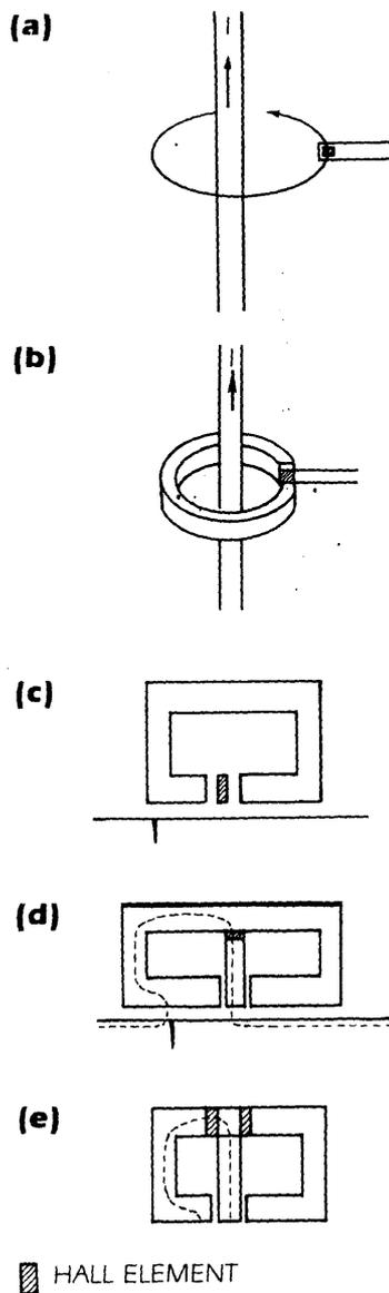
**FIGURE 15. Checking external field level with a meter after partial demagnetization**
