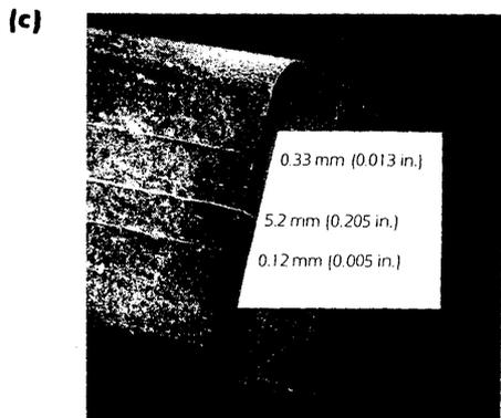
FIGURE 13. Ultraviolet photographs taken at the ends of square steel billets for comparison of magnetic particle indication brightness versus crack depth: (a) continuous direct current at 200 A; (b) continuous direct current at 800 A; and (c) residual direct current at 200 A
