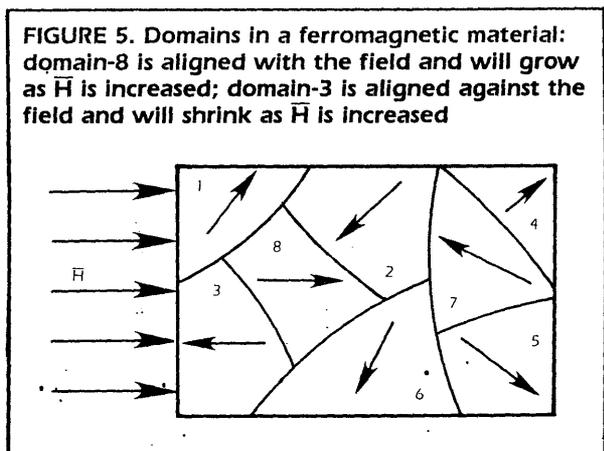
**FIGURE 5. Domains in a ferromagnetic material: domain-8 is aligned with the field and will grow as  $\bar{H}$  is increased; domain-3 is aligned against the field and will shrink as  $\bar{H}$  is increased**
