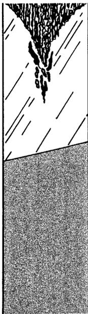
discarded, removing most of the shrinkage cavity and impurities. However, if the cavity is deeper than normal or if the cropping is short, some of the unsound metal will show up in the intermediate shape as a void called *pipe*.
