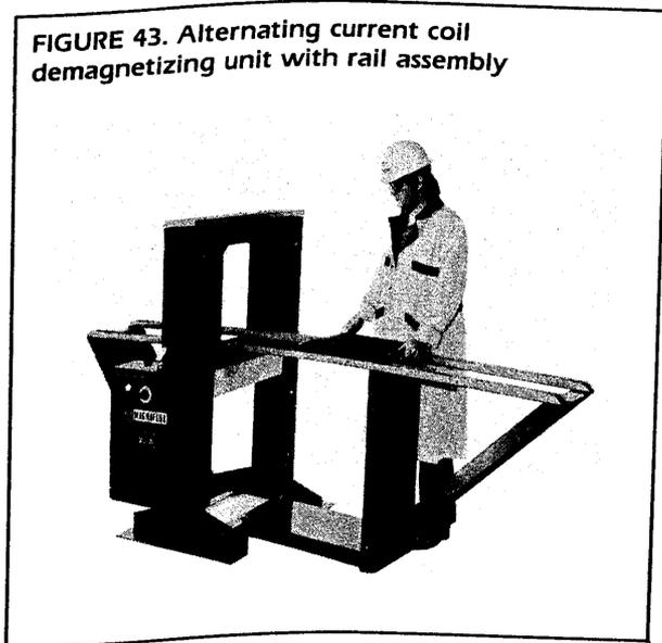
current is flowing for exposure to the maximum magnetic flux. The objects are then slowly and axially withdrawn some distance from the coil. Because flux intensity decreases with distance from its source, this procedure serves to reduce the magnetic field strength. To ensure that the flux is reduced to a minimum level, the objects should be withdrawn to a distance at least twice the coil diameter.
