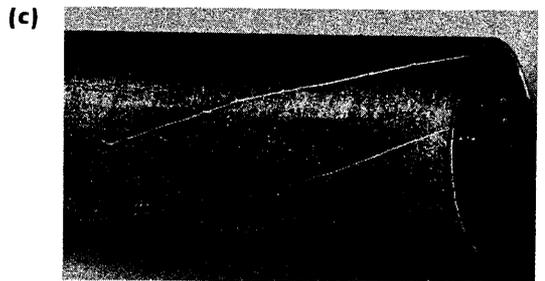
using magnetic particle testing to disclose detrimental seams. The method proved far superior to unaided visual testing, pickling and visual inspection, or skinning of the entire surface (in spite of its great waste, skinning was widely used at that time, especially for high quality steels). In 1958, another fluorescent magnetic particle system was installed for production testing of wire rod billets from 50 mm (2 in.) to 64 mm (2.5 in.) square and nominally 9 m (30 ft) long.
