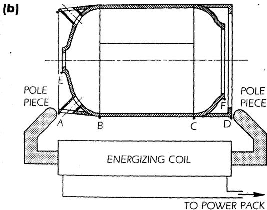
central conductor arrangement (not shown) for testing thin walled motor cases with a circumferential field. Figure 39 shows a special fixture for inducing alternating current in the cases' nozzle area without making electrical contact with the test object. This technique was used for detecting critical circumferential discontinuities in the welded area.
