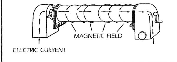
**FIGURE 23. Inducing a circumferential magnetic field using an internal conductor for: (a) a tube with inside and outside surface discontinuities; and (b) multiple ring shapes with cracking on the inside and outside surfaces**
