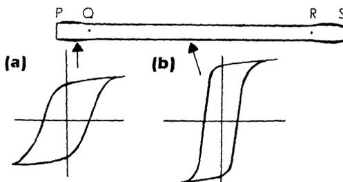
FIGURE 11. The axial bulk flux density in a 10 m (30 ft) long tube: (a) after longitudinal magnetization to saturation; and (b) after direct current coil demagnetization using a constant current; note the remanent flux density (1.14 T), the opposed dipole effect caused by the demagnetization process, and the values of the flux densities in the tube after this form of demagnetization
