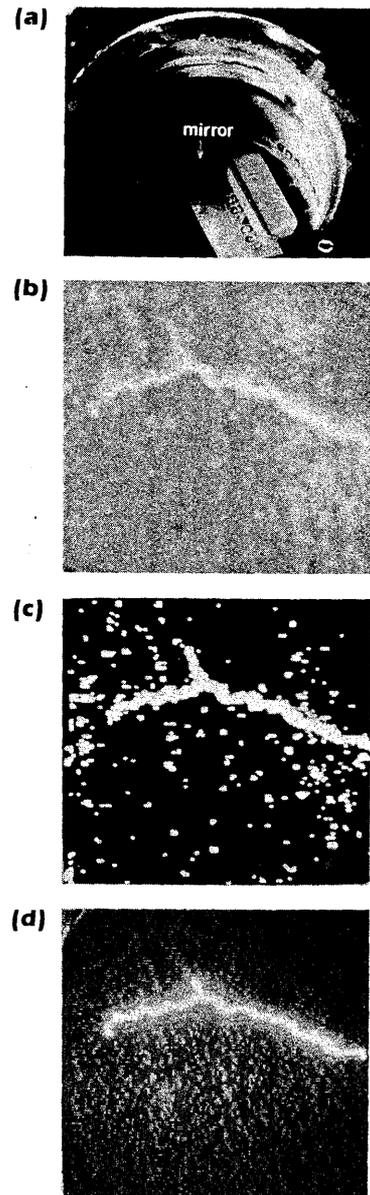
FIGURE 21. Use of neighborhood processing to enhance the image of a tube section, starting with the image before processing, progressing through several enhancement techniques to remove background, and ending with the final image of the discontinuity
