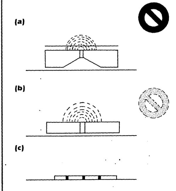
The device's sensitivity may be defined as the ability to produce a particle indication in an ambient magnetic surface field. In simple Foerster leakage field theory,<sup>13</sup> the particle holding ability depends on the product  $(H_g L_g)^2$ , where  $H_g$  is the magnetic field strength in the gap and  $L_g$  is the gap width.
