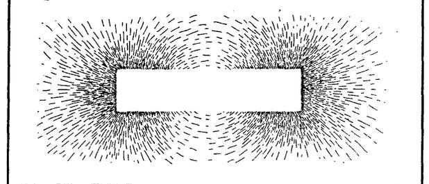
**FIGURE 14. Broken bar magnet illustrating locations of newly formed magnetic poles**
