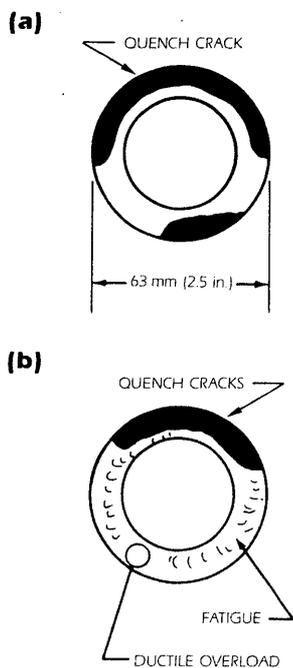
**FIGURE 16. Enlargement of magnetic particle crack indication in unfailed bellcrank**
