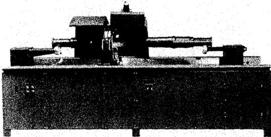
**FIGURE 16. Magnetic particle testing of steam turbine rotor blades**
