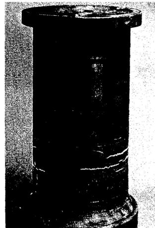
internal or external, and are at the same time exposed to a corrosive atmosphere, a particular kind of cracking results. Known as *stress corrosion cracking*, this discontinuity is easily detected by magnetic particle testing.
