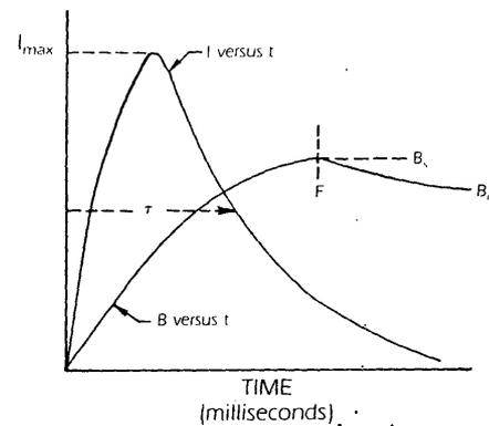
While the surfaces are magnetized sufficiently to form indications of longitudinal discontinuities, no information on the interior condition is required. However, when relatively thin elongated tubes can be inspected from the outside diameter surface only, saturation of the material is necessary for inside diameter discontinuities to produce magnetic flux leakage at the outside diameter.
