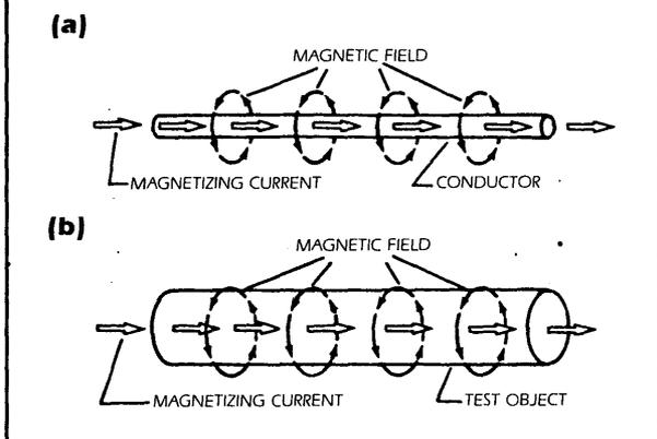
**FIGURE 22. Inducing a circumferential magnetic field in an object used as a conductor**
