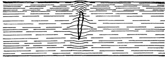
number of magnetic flux lines; (2) the depth of the discontinuity; and (3) the width of the discontinuity's air gap at the surface (the distance between the magnetic poles).
