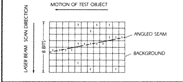
**FIGURE 16. Scanner memory matrix after an angled discontinuity has moved out of the array (at bottom) and a new discontinuity parallel to test object motion is in storage (near center)**
