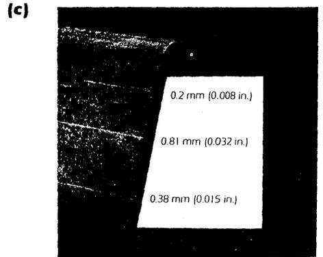
FIGURE 16. Ultraviolet photographs taken at the ends of square steel billets for comparison of magnetic particle indication brightness versus crack depth: (a) continuous direct current at 200 A; (b) continuous direct current at 800 A; and (c) residual direct current at 200 A
