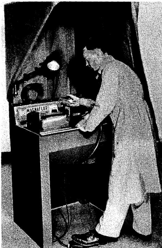
(Fig. 21). Gray iron foundries discovered the handheld magnetic yoke for detection of handling cracks in materials. Such tests were often included on the production line (Fig. 22).
