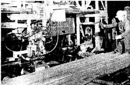
**FIGURE 21. Mobile magnetic particle testing unit using prods; system employed half-wave current on a 3,400 kg (7,500 lb) steel casting (early 1950s)**
