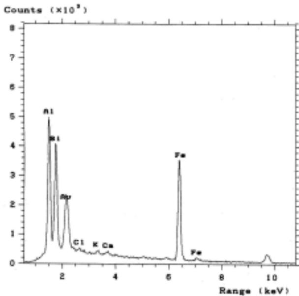
Figure 7. X-ray spectroscopy of damaged part of the crucible
