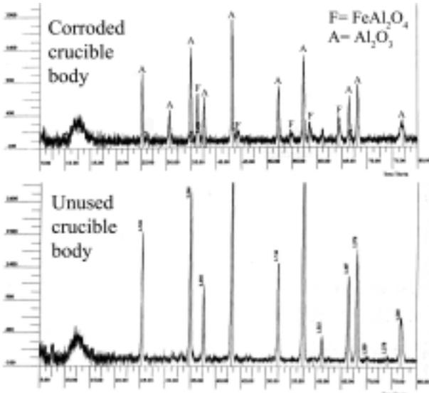
Figure 3. XRD pattern of the corroded crucible body vs. the unused crucible body
