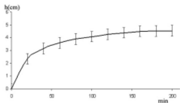
Figure 2. Relation between thermite reaction time (min) and thickness of corroded crucible (cm) (Bars refer to standard error)
