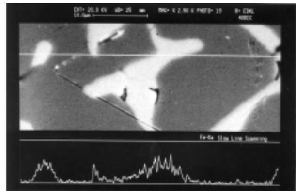
Figure 8. SEM micrograph of the corroded parts with Fe line scan
