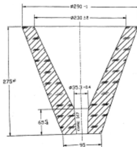
Figure 1. Schematic figure of crucible
