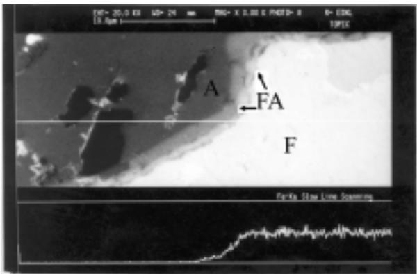
Figure 4. SEM micrograph of the surface of corroded parts with Fe line scan
