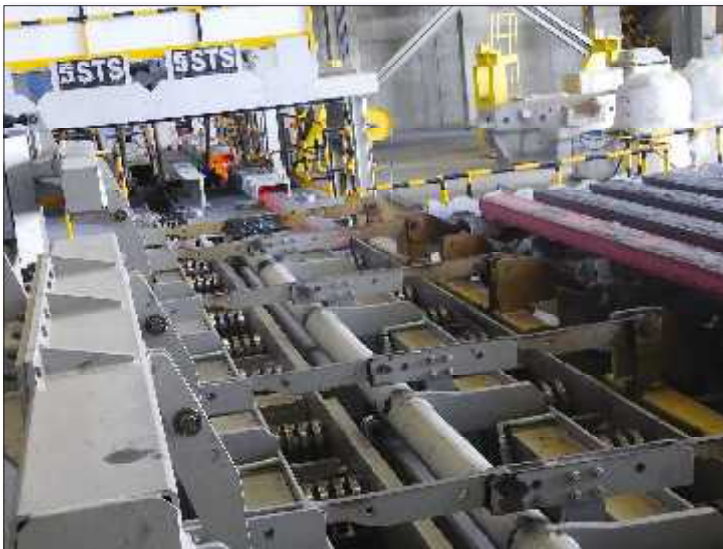
Fig 5 Cut to length blooms on cooling bed
